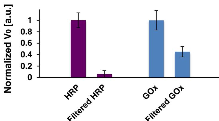
**Figure S1.** Normalized initial rate of reactions in arbitrary units for unfiltered and filtered HRP and GOx samples (determined from triplicate samples).
