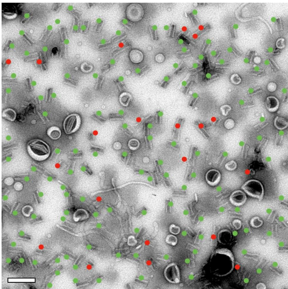
*Figure S2. Additional TEM image of origami dimers. In this typical image taken after 1-day incubation of monomers at room temperature, 86 % of all the observed objects are correctly formed dimers (marked with green dots) and only 14 % of the objects (marked with red dots) are either monomers or incorrectly assembled multimers. The scale bar is 100 nm.*
