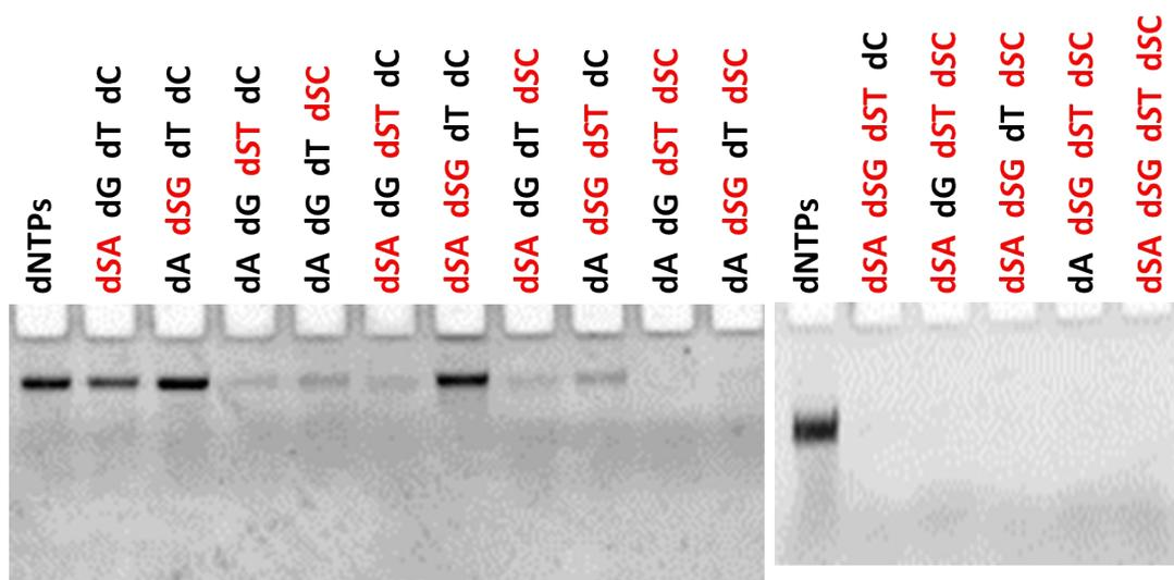
**Fig. S1.** Representative gel image of the *in vitro* transcription of natural RNA for various DNA templates containing 4'-thionucleotides by T7 RNA polymerase.
