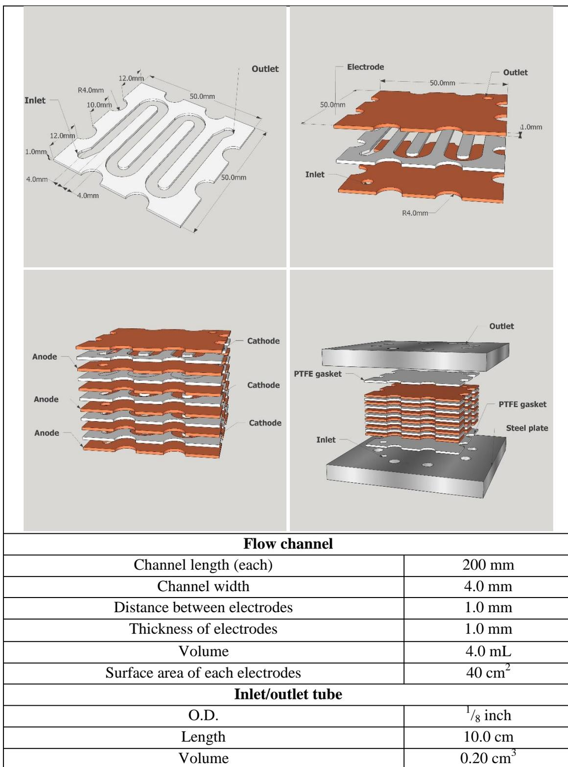
**Figure S5.** Simulated design images of flow-cell comprising a PTFE flow channel/spacer (top left), cathode-spacer-anode sequence (top right), extended stacked-disk arrangement (bottom left) and steel encasement (bottom right).
