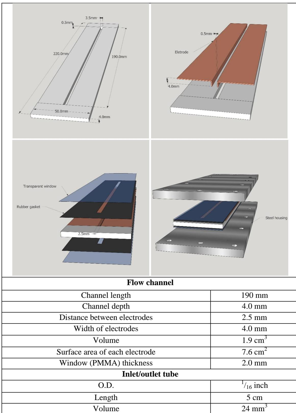
**Figure S2.** Simulated design images of flow-cell comprising a PTFE flow channel (top left), two copper electrodes (top right), rubber gaskets (bottom left) and steel encasement (bottom right).
