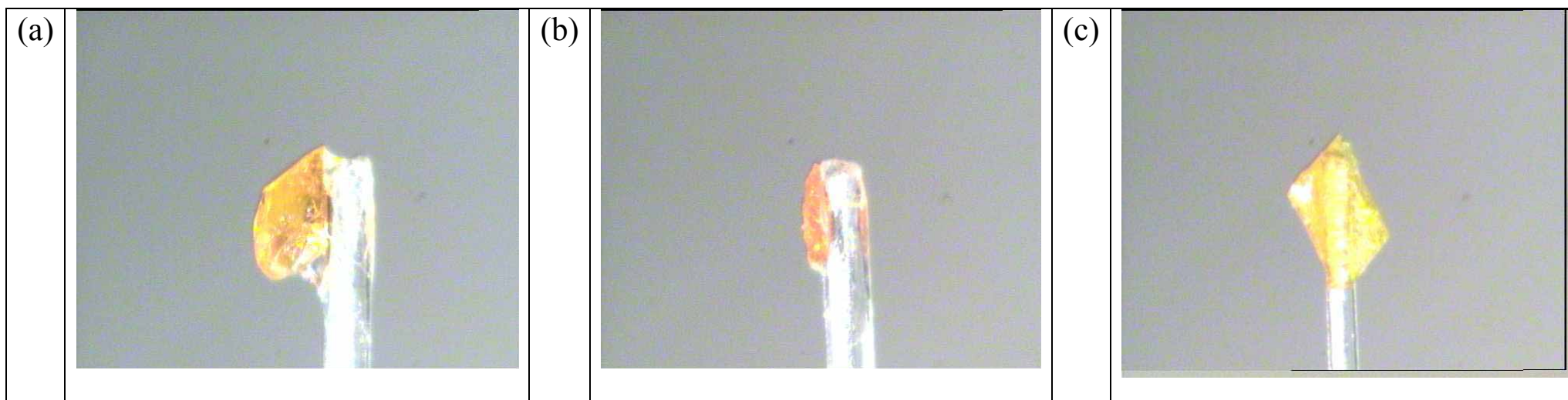
Figure S1 Pictures of crystals of (a) form I, (b) form II and (c) form III of 1 mounted for single crystal X-ray diffraction.
