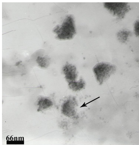
Fig. S2. The TEM image of intermediate of stearic acid wrapped nanocrystals during purification process, which were captured by purifying incompletely. The arrow in the picture showed the dissociation of the stearic acid in the purifying process and the nanocrystals were released from s unwrapping stearic acid. See detail discussions in the text.
