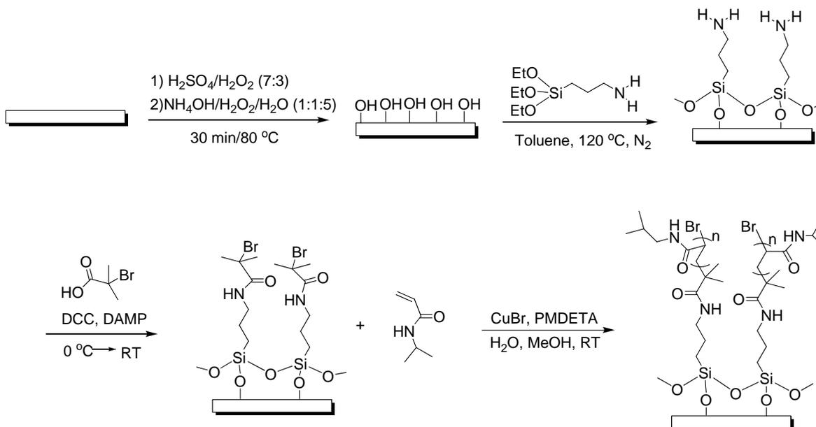
**Scheme S1** Synthesis of poly(*N*-isopropylacrylamide) by surface-initiated ATRP.
