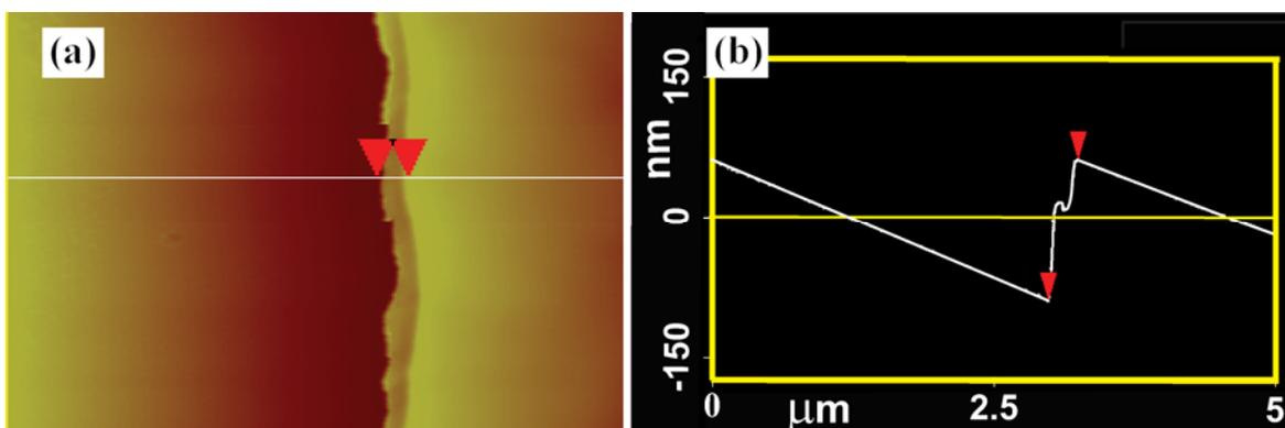
**Fig. S1** A cross-sectional tapping mode AFM image of the surface-initiated poly(NIPAm) immobilized on a glass substrate: (a) height image; (b) cross-sectional profile along the line in the part (a).
