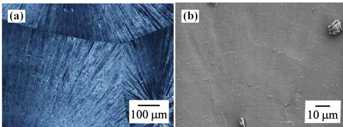
**Fig. S3** Calcium carbonate crystals grown on the poly(NIPAm) brush matrix in the presence of poly(acrylic acid) (PAA) ( $2.5 \times 10^{-3}$  wt%) at 40 °C: (a) polarized optical micrograph (POM) image; (b) scanning electron microscopy (SEM) image (top view).
