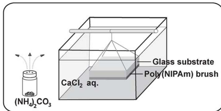
**Fig. S2** Schematic representation of the experimental setup for the crystallization of CaCO<sub>3</sub> on poly(NIPAm) matrices using an ammonium carbonate diffusion method.
