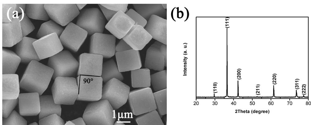
Fig. S1 (a) FESEM image and (b) XRD pattern of the cubic  $\text{Cu}_2\text{O}$  seeds.
