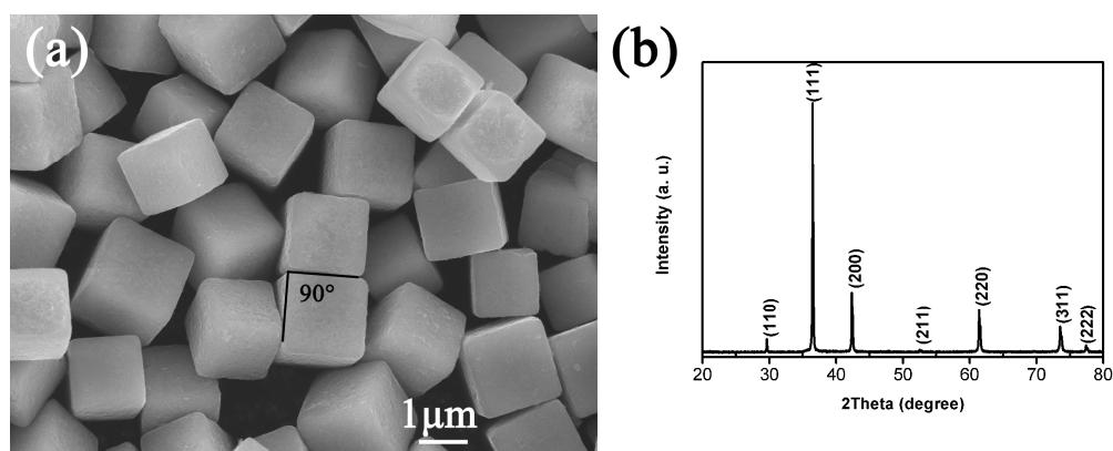
Fig. S1 (a) FESEM image and (b) XRD pattern of the cubic Cu<sub>2</sub>O seeds.
