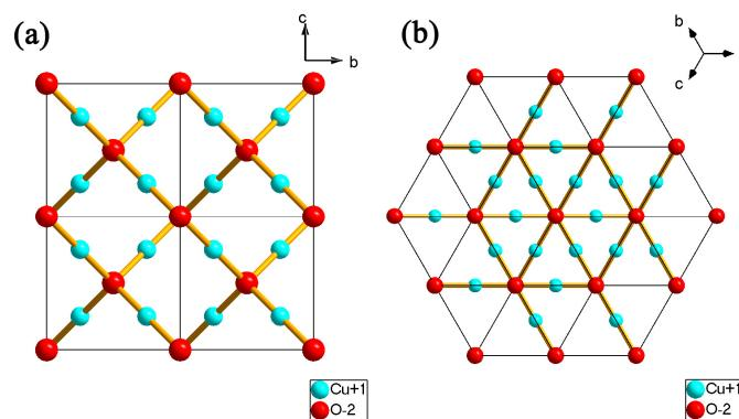
Fig. S2 The crystallographic structures of {100} (a) and {111} (b) facets of Cu<sub>2</sub>O crystal.
