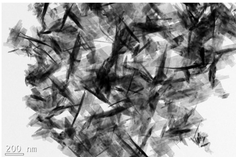
**Fig. S4** A TEM image of the products obtained in the in the concentration of reagents ( $\text{Cu}(\text{NO}_3)_2 = 0.4 \text{ M}$ ,  $\text{NaOH} = 2 \text{ M}$ ) under otherwise the same conditions.
