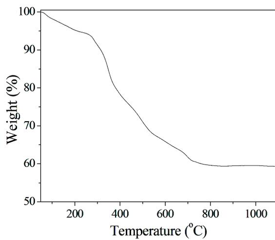
**Fig S10.** The TGA curve of compound 2.
