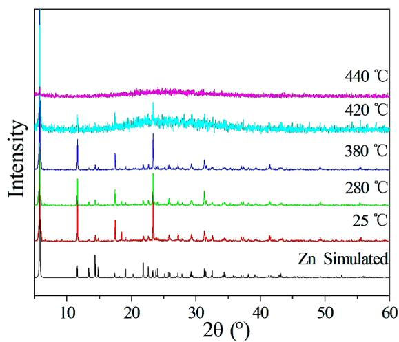
**Fig S15.** The PXRD patterns for compound **4** on heating from 25–440 °C.
