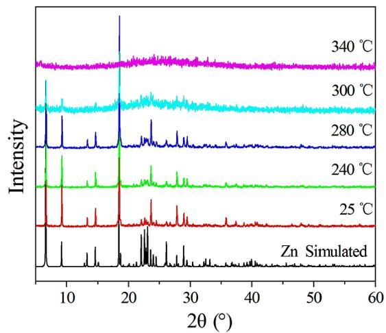
**Fig S13.** The PXRD patterns for compound **3** on heating from 25–340 °C.
