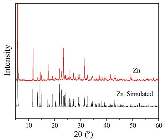
**Fig S4.** The experimental powder XRD patterns and the simulated XRD patterns of compound **4**.
