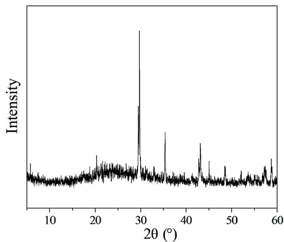
**Fig S14.** The X-ray power diffraction patterns of the final products in the thermal decomposition for compound **4**.
