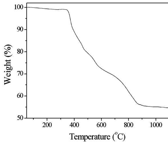
**Fig S11.** The TGA curve of compound 3.
