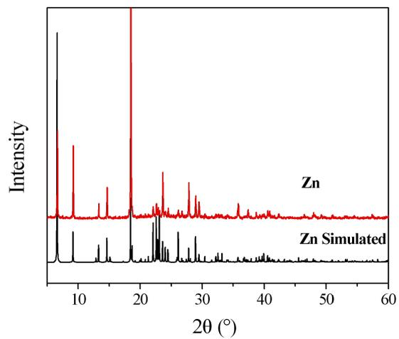
**Fig S3.** The experimental powder XRD patterns and the simulated XRD patterns of compound **3**.
