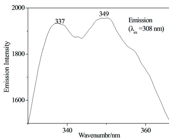
**Fig S16.** Solid-state emission spectrum of H<sub>5</sub>L at room temperature.
