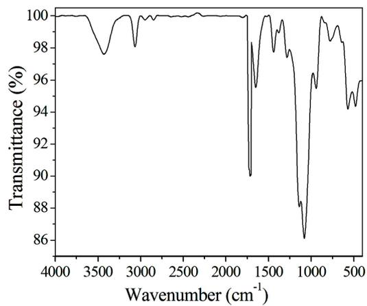
**Fig S6.** The IR spectrum of compound **2**.
