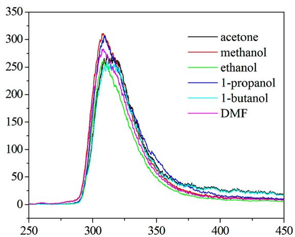
**Fig S17.** Emission spectrum of compound **3** in various pure solvents when excited at 240 nm.
