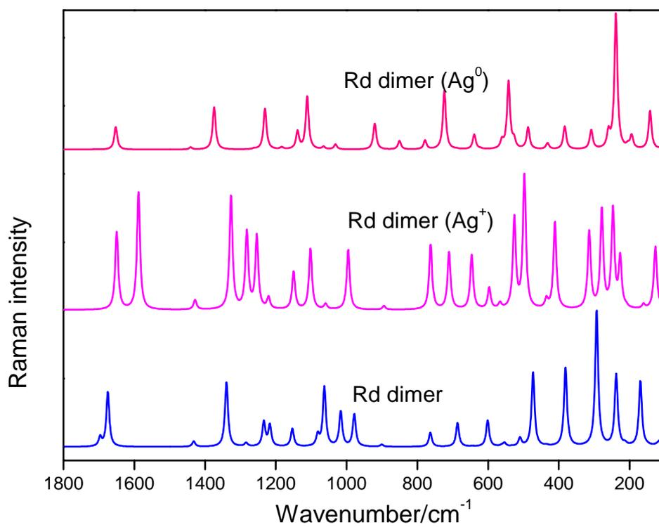
**Fig. S2** Calculated SERS spectra for the hypothetical (“polymer”/ $\text{N}^+=\text{C}$ ) Rd dimers shown in Fig. S1.
