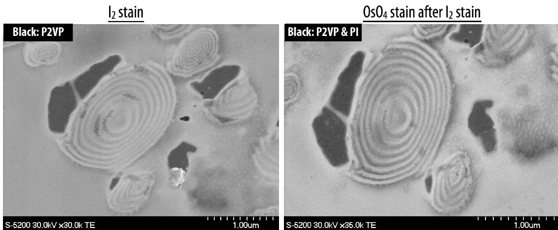
S2. TEM images of sliced #1 particles sequencially stained with I<sub>2</sub> (left) and OsO<sub>4</sub> (right), respectively. The same region was staind after OsO<sub>4</sub> treatment.
