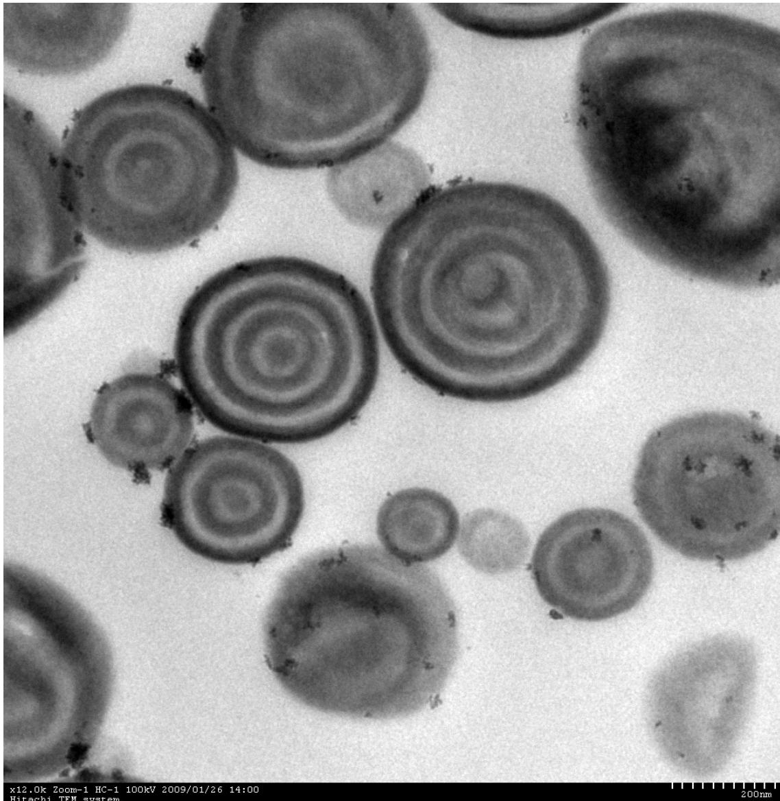
S1. Cross-sectional TEM image of #1 particles. All particles have onion-like structure.
