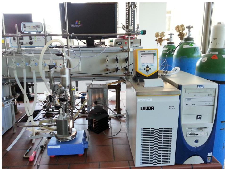
Figure 2. Photocatalytic setup for stirred dispersions.
