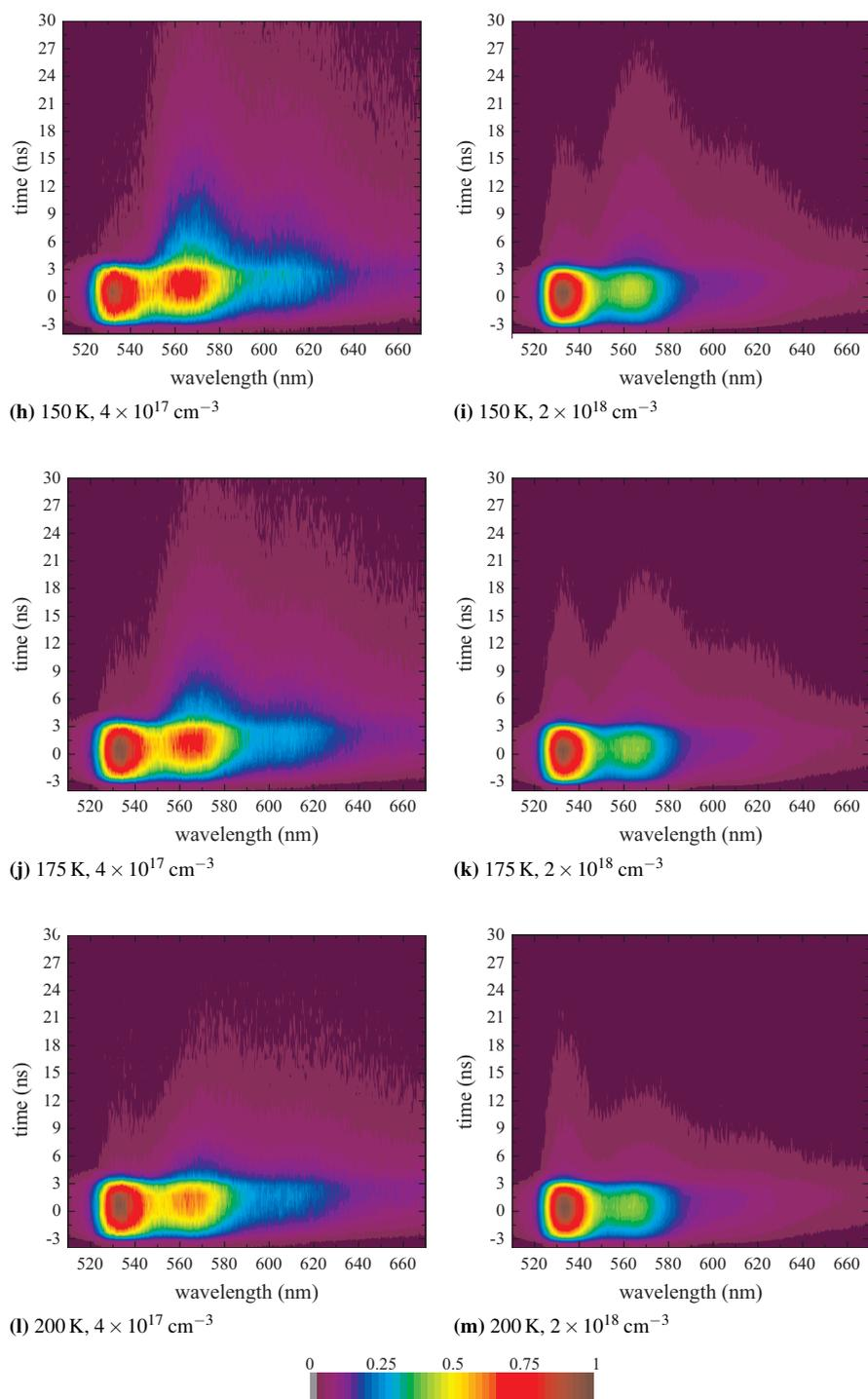
**Fig. 4** Contour plots of the normalized PL of Tc thin films as a function of time and wavelength conducted at 150 K, 175 K, and 200 K after excitation at 500 nm. The exciton density at which the experiments were conducted are also shown.
