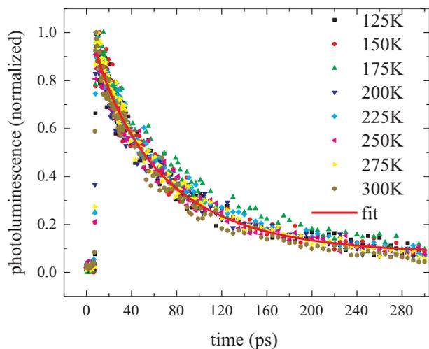
**Fig. 1** Ultrafast time-resolved PL at 575 nm of tetracene thin films after pumping at 500 nm, achieving an exciton density of  $4 \times 10^{17} \text{ cm}^{-3}$  at a number of different temperatures. The fit parameters are  $1/k_1 = 80 \text{ ps}$  and  $\beta_{ssa} = 0.34$ .
