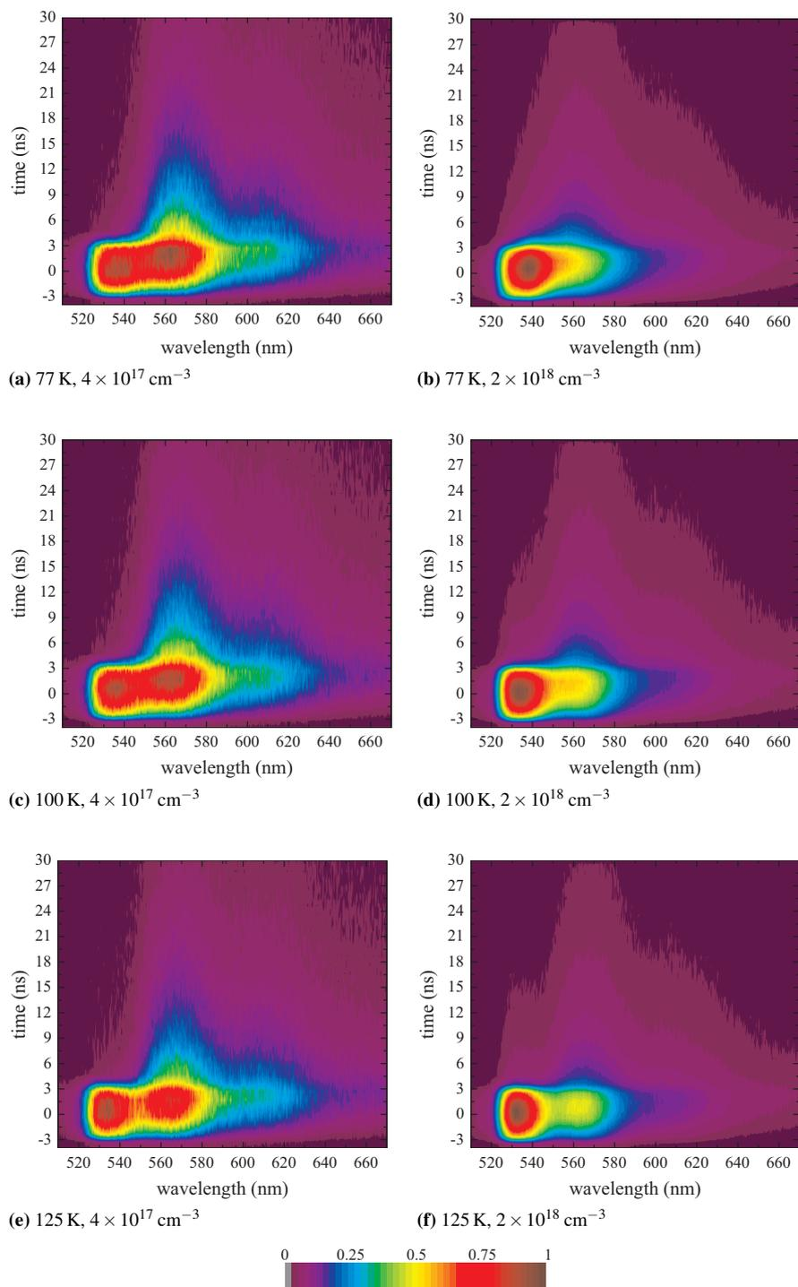
**Fig. 4** Contour plots of the normalized PL of Tc thin films as a function of time and wavelength conducted at 77 K, 100 K, and 125 K after excitation at 500 nm. The exciton density at which the experiments were conducted are also shown.
