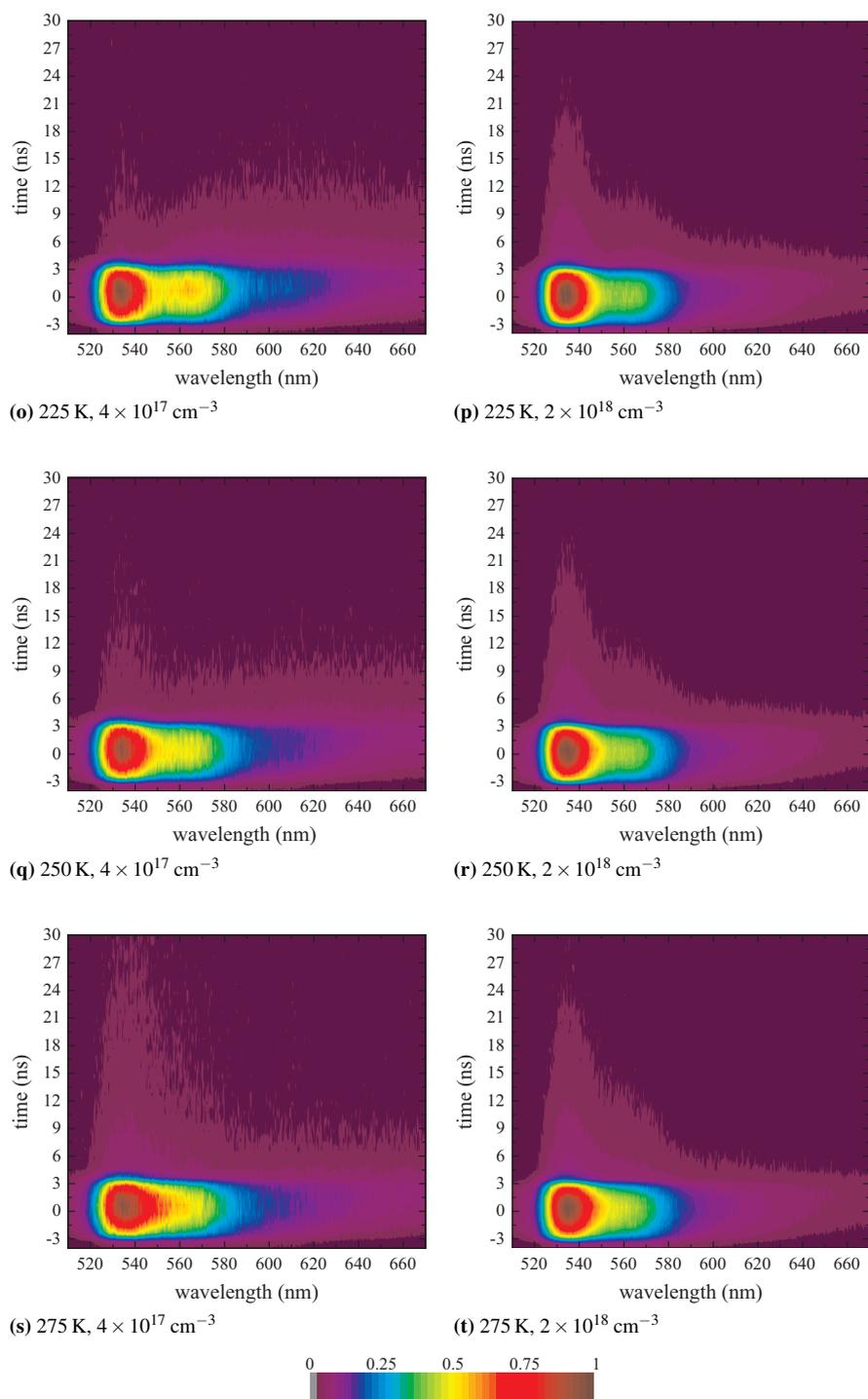
**Fig. 4** Contour plots of the normalized PL of Tc thin films as a function of time and wavelength conducted at 225 K, 250 K, and 275 K after excitation at 500 nm. The exciton density at which the experiments were conducted are also shown.
