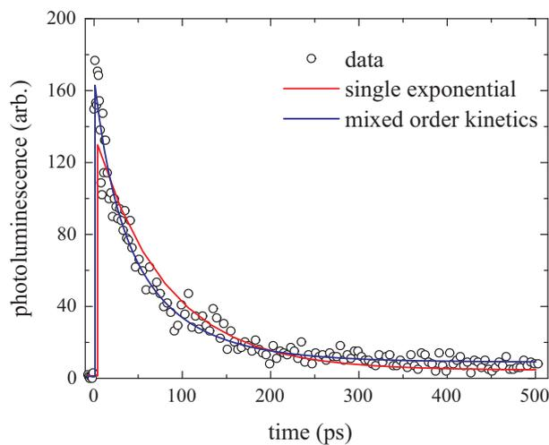
**Fig. 2** Ultrafast time-resolved PL of tetracene thin films at 560 nm after pumping at 500 nm, achieving an exciton density of  $\sim 8 \times 10^{17} \text{ cm}^{-3}$ . The single exponential fit uses a value of  $1/k_1 = 80 \text{ ps}$ . The mixed kinetics model uses an additional parameter  $\beta_{ssa} = 0.54$ .
