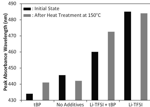
**SI Figure 1.** Peak wavelength of solid-state absorbance of D35-dyed  $\text{TiO}_2$  films with varying additives present in the film introduced during spiro-OMeTAD deposition. Effect of heating the films to 150°C is shown and demonstrates that tBP is evaporating.
