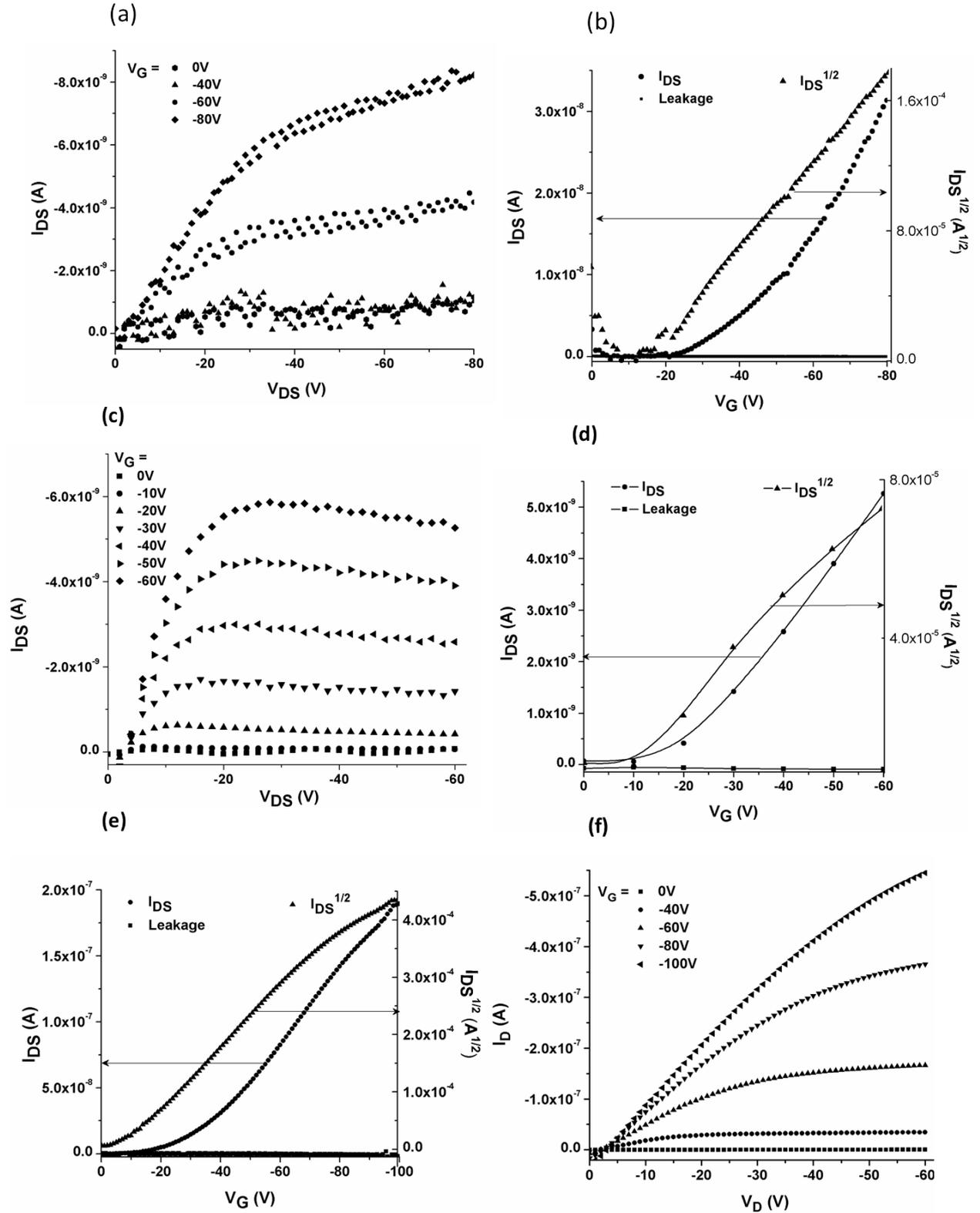
**Figure S19.** (a) Output characteristic curve of **1** for unmodified substrate, (b) Transfer characteristic curve of **1** for unmodified substrate, (c) Output characteristic curve of **2** for unmodified substrate, (d) Transfer characteristic curve of **2** for unmodified substrate, (e) Transfer characteristic curve of **3** for unmodified substrate and (f) Output characteristic curve of **4** for modified substrate.
