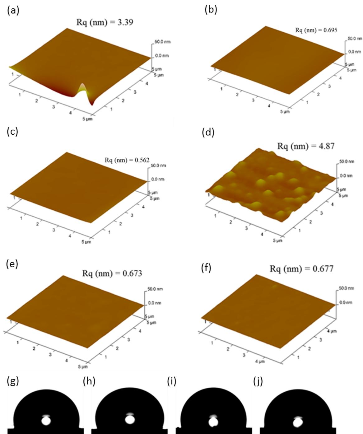
**Figure S17.** AFM height images and root mean square roughness ( $R_q$ ) of thin films: On unmodified SiO<sub>2</sub> substrate of **2** (a), **3** (b) and **4** (c) and on modified SiO<sub>2</sub> of **1** (d), **2** (e) and **3** (f). CA of **1** (g), **2** (h), **3** (i) and **4** (j) coated on HMDS modified SiO<sub>2</sub> surface.
