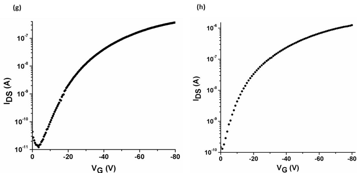
**Figure S21.** Drain current,  $I_D$  versus gate voltage,  $V_G$  plots for CSMs on unmodified and modified substrates.  $I_D$  is plotted on a semi-logarithmic scale as a function of gate voltage at constant Drain voltage: Plots for silane modified substrates: (g) **3**, and (h) **4**.
