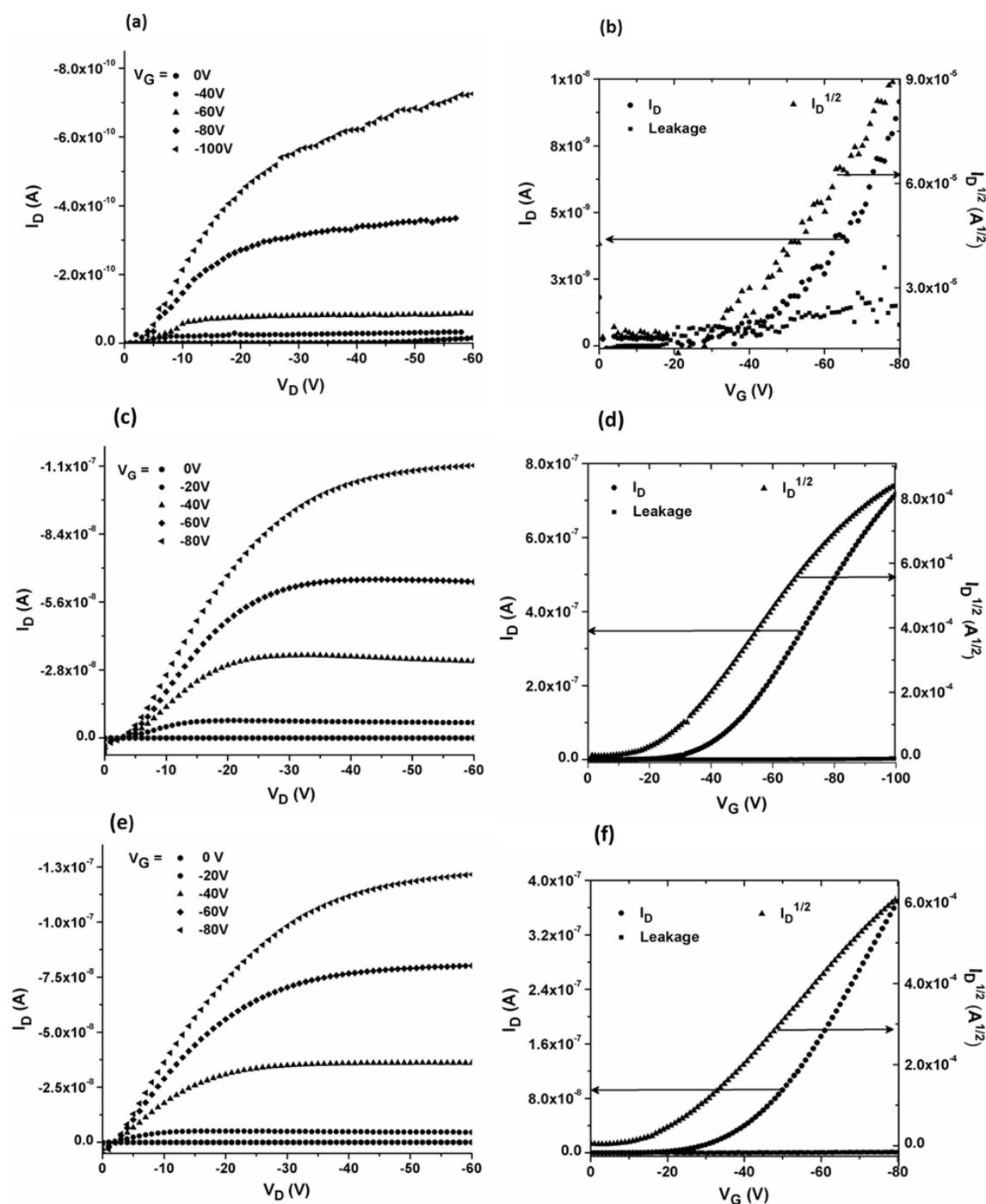
**Figure S18.** (a) Output characteristic curve of (a) **1** for HMDS modified substrate, (b) Transfer characteristic curve of **1** for HMDS modified substrate, (c) Output characteristic curve of **2** for HMDS modified substrate, (d) Transfer characteristic curve of **2** for HMDS modified substrate, (e) Output characteristic curve of **3** for HMDS modified substrate and (f) Transfer characteristic curve of **3** for HMDS modified substrate.
