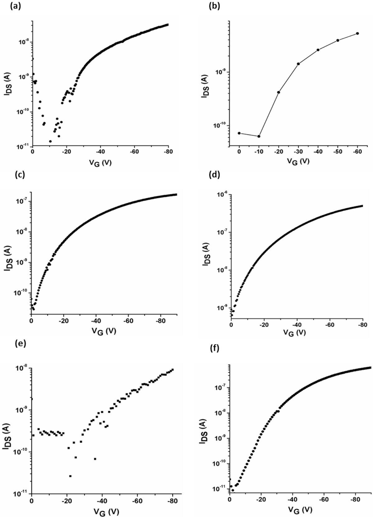
**Figure S20.** Drain current,  $I_D$  versus gate voltage,  $V_G$  plots for CSMs on unmodified and modified substrates.  $I_D$  is plotted on a semi-logarithmic scale as a function of gate voltage at constant Drain voltage: (a) 1, (b) 2, (c) 3, and (d) 4 on unmodified substrates. Plots for silane modified substrates: (e) 1, (f) 2.
