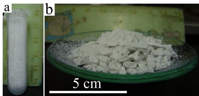
Fig. SI 1. The digital images of the as-prepared S 1 (a) and S 2 (b). S 2 (0.66g~1g) was prepared by using 40 mmol B 2 O 3 , 200 mmol zinc powder and 50 mmol N 2 H 4 ·2HCl
