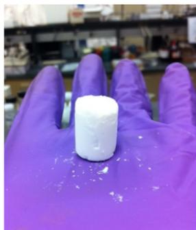
ESI Fig. S2: Free standing aerogel after supercritical drying
