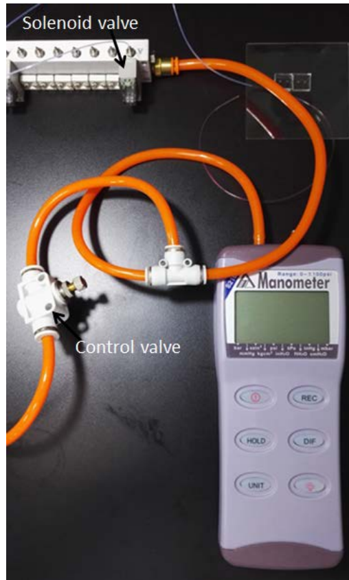
Figure S2 Set-up used for the leakage test of the modular microfluidic circuits. The solenoid valve is normally open and here just used as an adapter.
