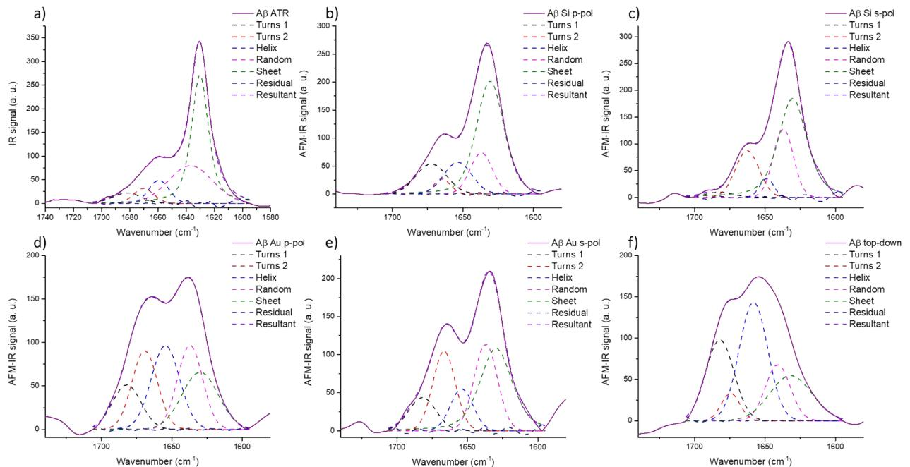
Figure SI 5. Secondary structure analysis of A $\beta$  : a) ATR-FTIR, b) AFM-IR bottom-up configuration with Si-tip and p-pol, c) AFM-IR bottom-up configuration with Si-tip and s-pol,
