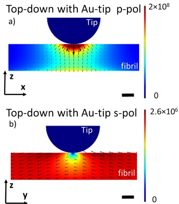
Figure SI 3. Finite elements simulation of the electric field induced in fibrils by Top-down illumination with Au-tip and gold substrate in a cross-section along the fibril axis: p-
