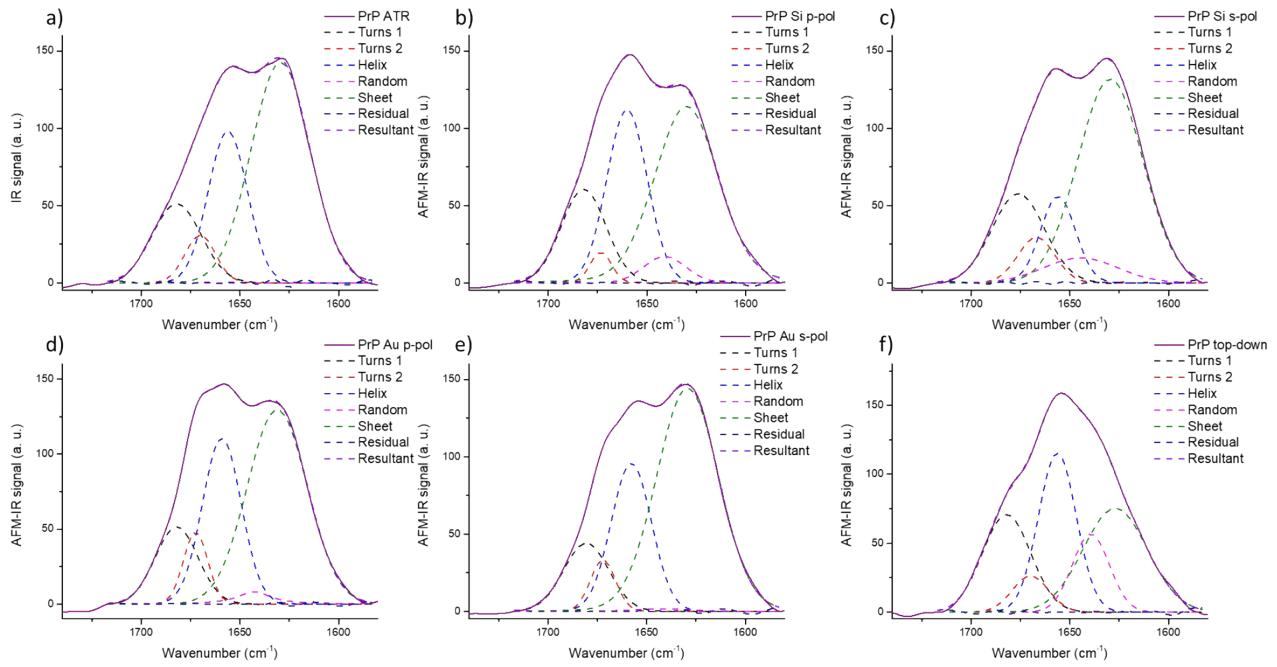
Figure SI 7. Secondary structure analysis of PrP : a) ATR-FTIR, b) AFM-IR bottom-up configuration with Si-tip and p-pol, c) AFM-IR bottom-up configuration with Si-tip and s-pol, d) AFM-IR with top-down illumination with Au-tip and p-pol, e) AFM-IR bottom-up configuration with Au-tip and p-pol and f) AFM-IR bottom-up configuration with Au-tip and s-pol. The colored dashed line corresponds to the curve fitting for the different components and solid line to the spectra
