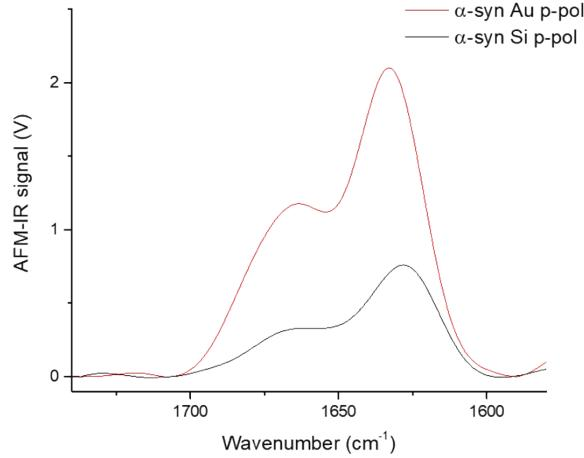
Figure SI 4. Effect of the enhancement of the Au-coating. Black curves correspond to Si-tip and red curves to Au-tip with a bottom-up illumination at p-pol and without scaling. The signal obtained with the Au-tip is around 2 times bigger than the signal with Si-tip.
