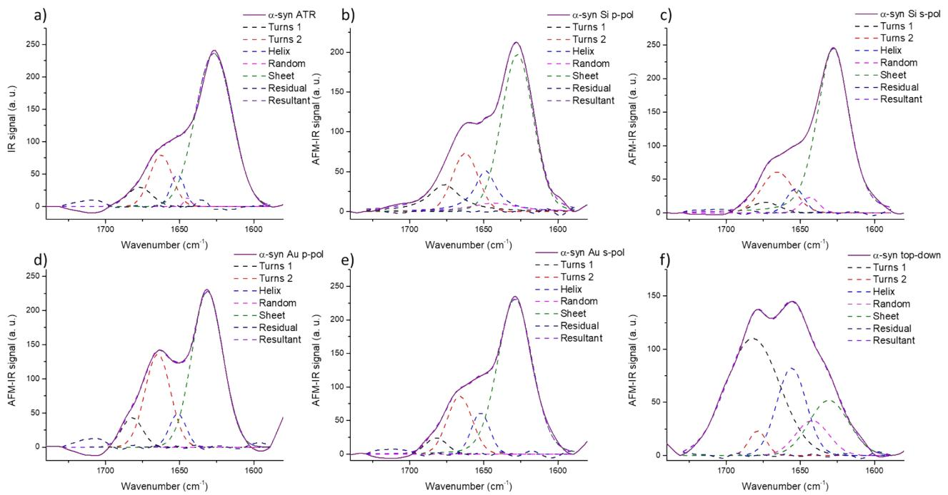
Figure SI 6. Secondary structure analysis of  $\alpha$ -syn : a) ATR-FTIR, b) AFM-IR bottom-up configuration with Si-tip and p-pol, c) AFM-IR bottom-up configuration with Si-tip and s-pol, d) AFM-IR with top-down illumination with Au-tip and p-pol, e) AFM-IR bottom-up configuration with Au-tip and p-pol and f) AFM-IR bottom-up configuration with Au-tip and s-pol. The colored dashed line corresponds to the curve fitting for the different components and solid line to the spectra
