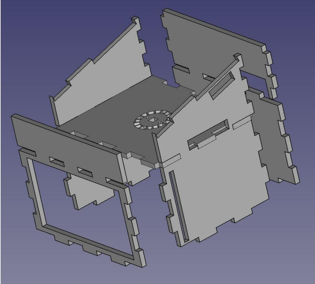
13) Lay the whole assembly over the [BOTTOM\_BASE].
