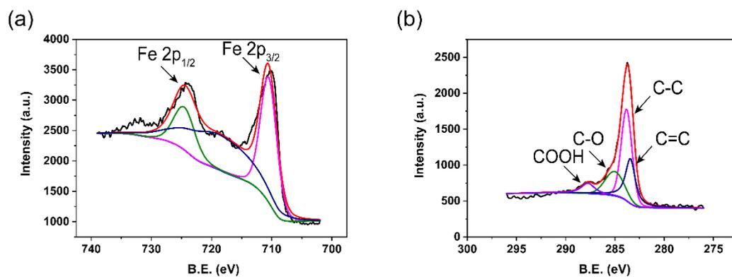
**Figure S1.** XPS spectra of Fe 2p (a) and C 1s (b) of Fe<sub>3</sub>O<sub>4</sub>@GO MNCs.
