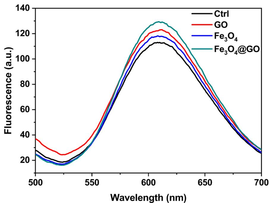
**Figure S4.** SOD-like activity of indicated NPs. Fluorescent spectra of dihydroethidine (HE) after reacting with xanthine (X) and xanthine oxidase (XO), in the absence and presence of GO, Fe<sub>3</sub>O<sub>4</sub>, and Fe<sub>3</sub>O<sub>4</sub>@GO MNCs, respectively.
