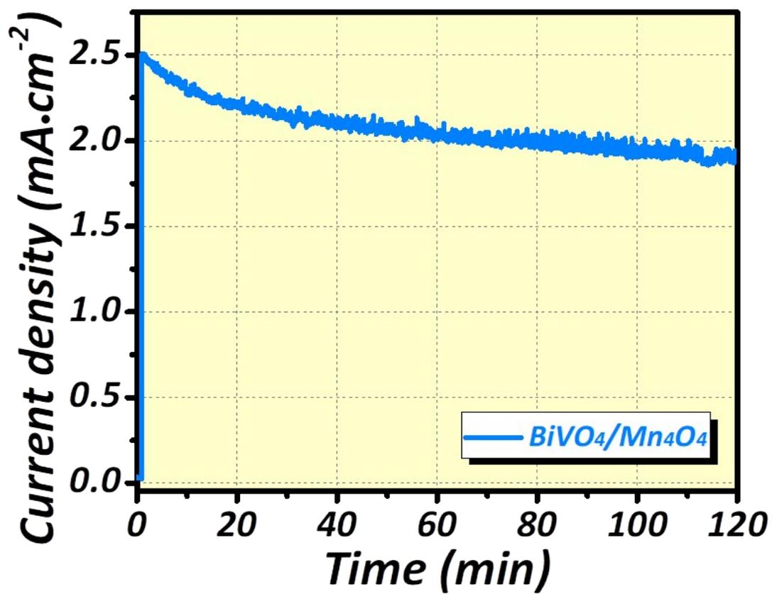
Figure S6. I-t curve of BiVO<sub>4</sub>/Mn<sub>4</sub>O<sub>4</sub>.
