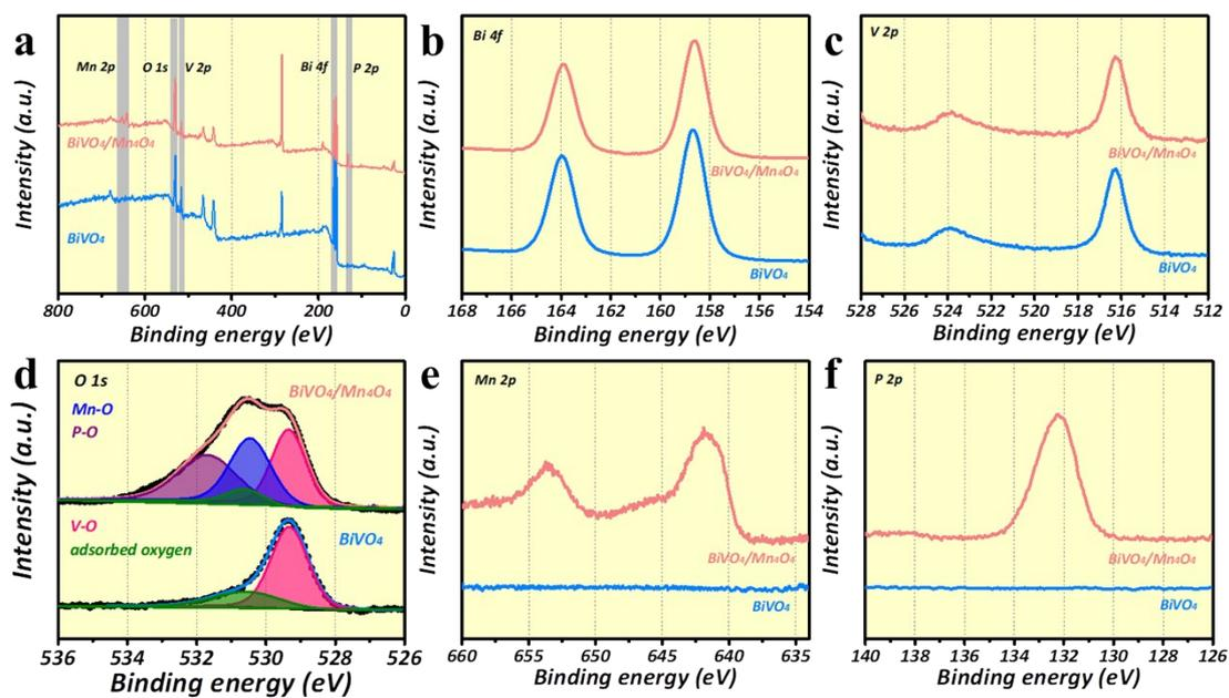
**Figure S4.** XPS survey spectra (a) and high-resolution of Bi 4f (b), V2p (c), O 1s (d), Mn 2p (e) and P 2p (f).
