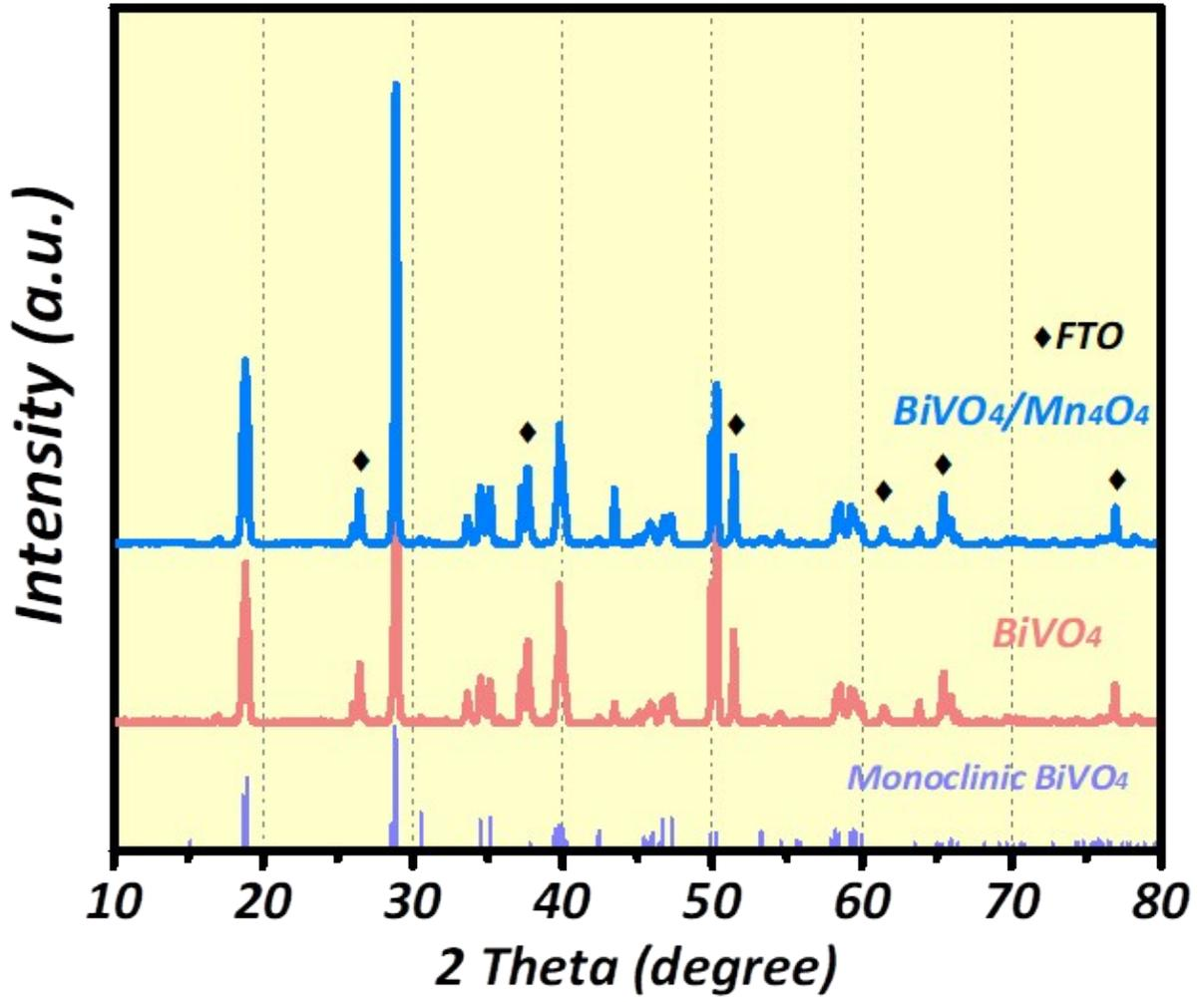
Figure S2. XRD spectra of  $\text{BiVO}_4$  and  $\text{BiVO}_4/\text{Mn}_4\text{O}_4$ .
