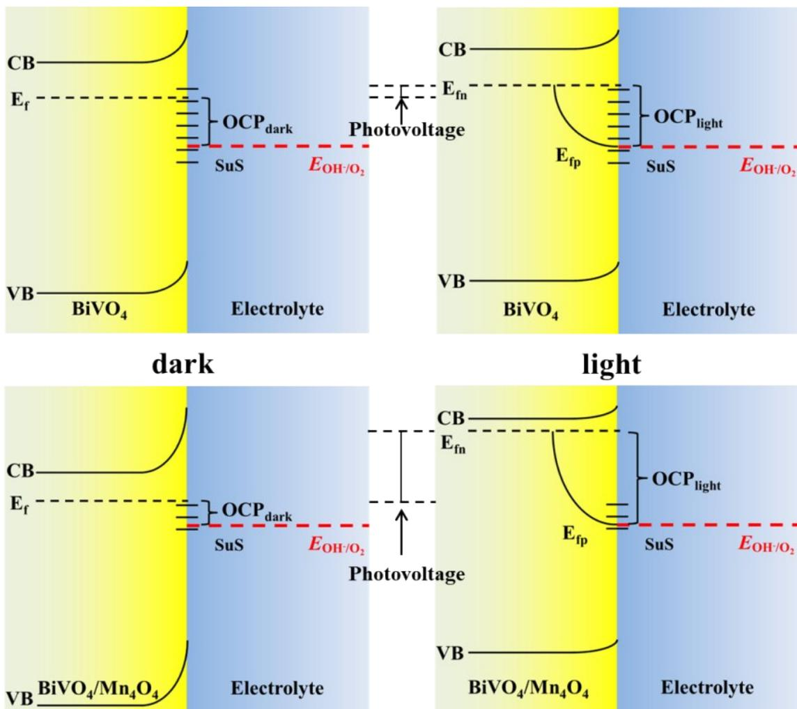
**Figure S7.** Band structure and band bending schematics of BiVO<sub>4</sub> and BiVO<sub>4</sub>/Mn<sub>4</sub>O<sub>4</sub>.
