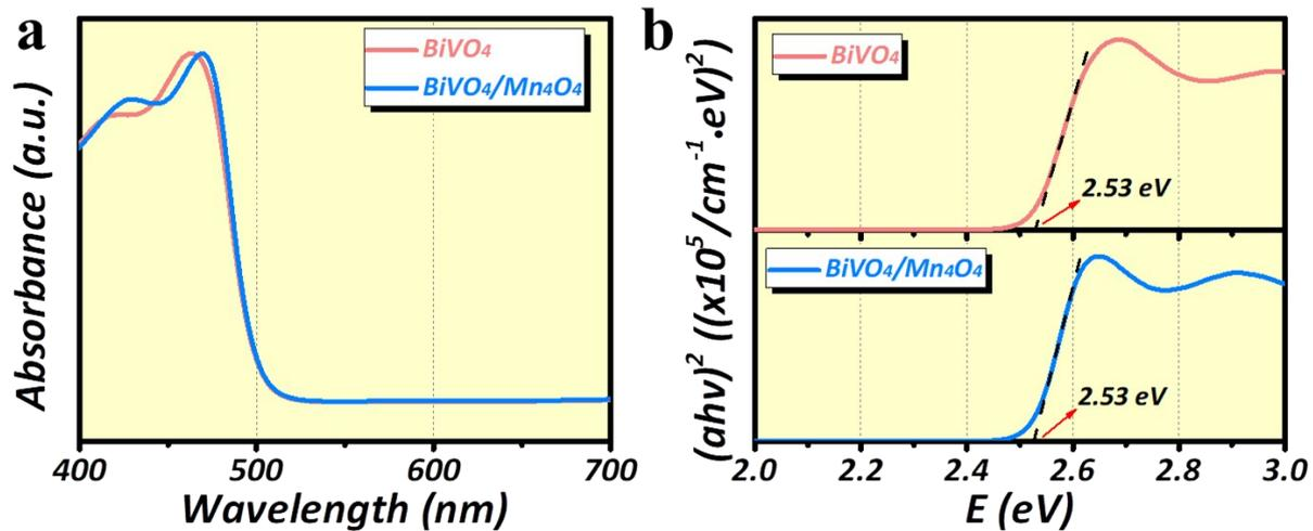
Figure S5. UV-Vis spectra (a) and Tauc-plots (b) of  $\text{BiVO}_4$  and  $\text{BiVO}_4/\text{Mn}_4\text{O}_4$ .
