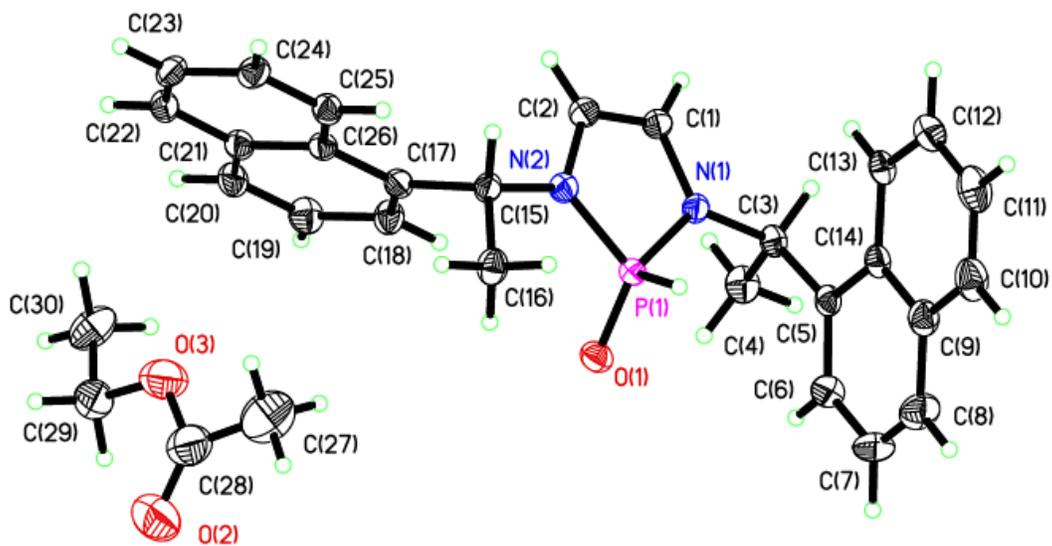
**Figure S1.** Structural diagram of compound **2b** including one part of the disordered ethyl acetate solvent molecule. Thermal ellipsoids are drawn at the 50% probability level. Hydrogen atoms have not been labelled.
