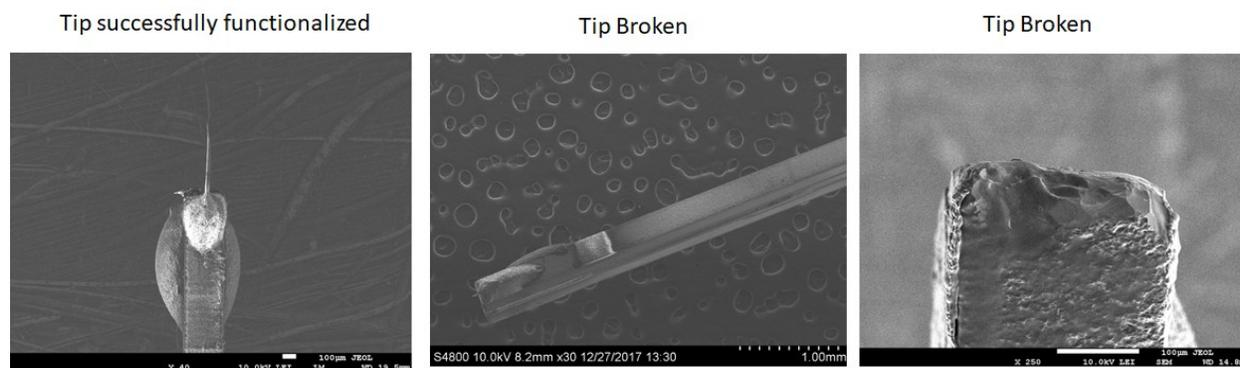
**Figure S2.** SEM images of functionalized tip and tip fail to functionalized.
