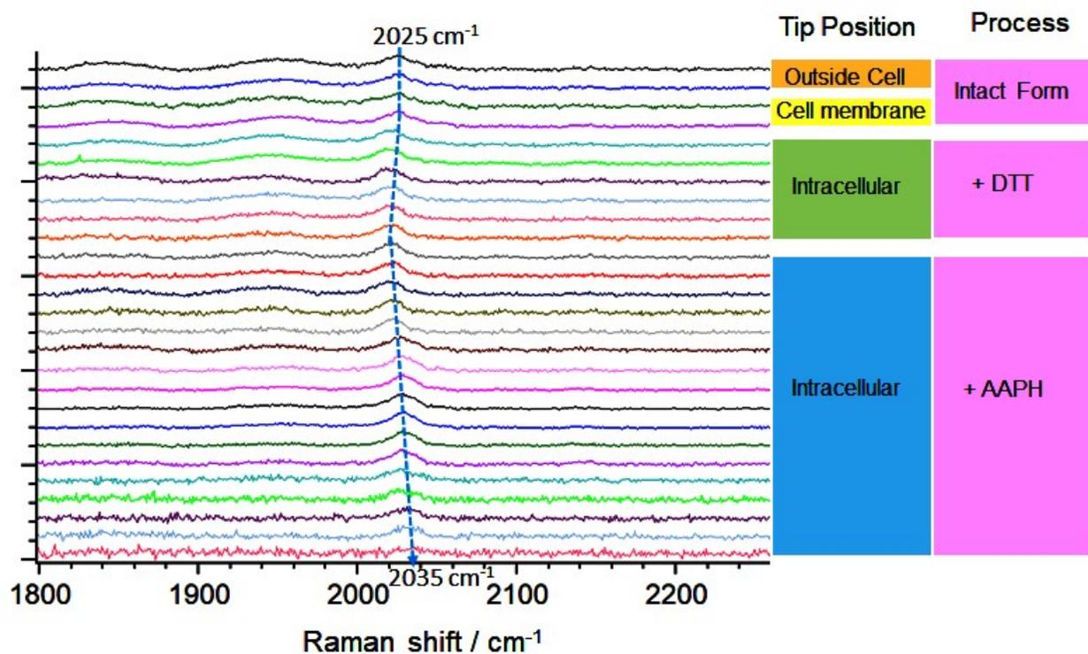
**Figure S5.** Direct detection of DTT and AAPH induce charge-transfer process as reflected by CO band position.
