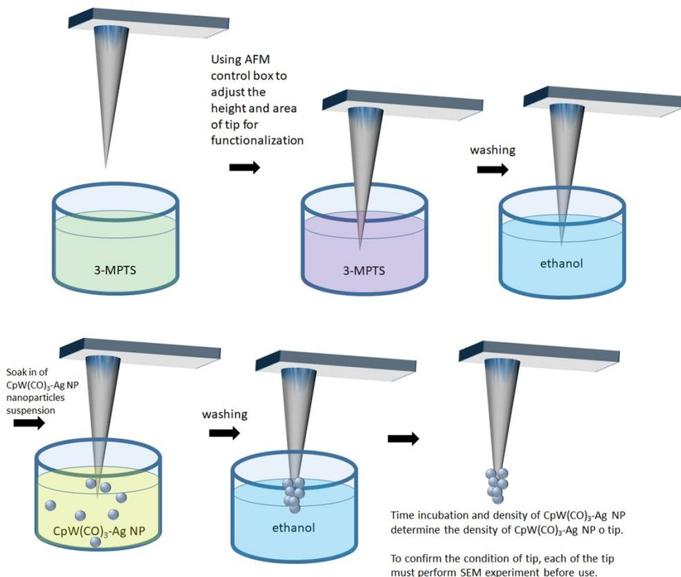
**Figure S1.** Fabrication of tip with  $\text{CpW}(\text{CO})_3\text{-Ag NP}$ .
