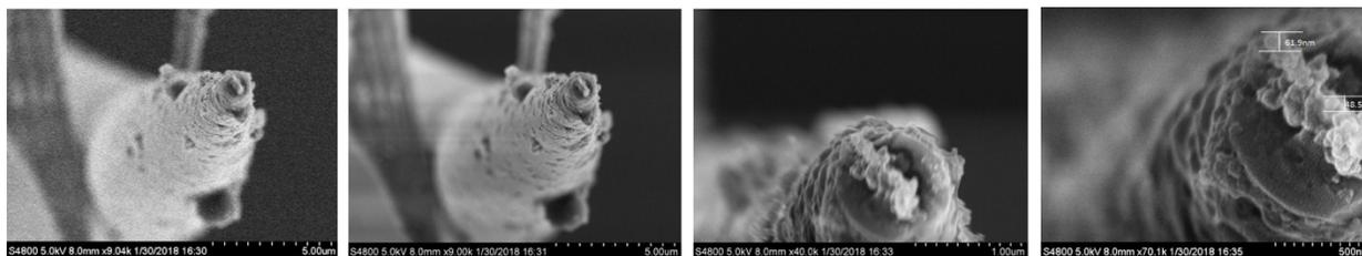
**Figure S3.** SEM images after processing AFM tip.
