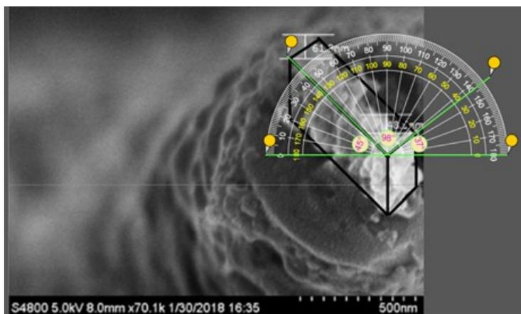
Considering the shape of nanoparticles clustered on nanotip as a cuboid shape. We then estimate the dimension of the cuboid (Length, width and height) which is 600 nm, 146.7 nm and 266.7 nm. By considering the angle of the nanotip in SEM image, we could obtain the size of the cuboid is  $[600 \text{ nm} \cdot \cos(45^\circ)] \times [146.7 \text{ nm} \cdot \cos(37^\circ)] \times [266.7 \text{ nm}] = 41,568,690 \text{ nm}^3$
