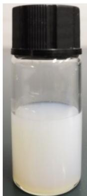
**Fig. S1.** Photograph of the g-C<sub>3</sub>N<sub>4</sub> nanosheets suspension.
