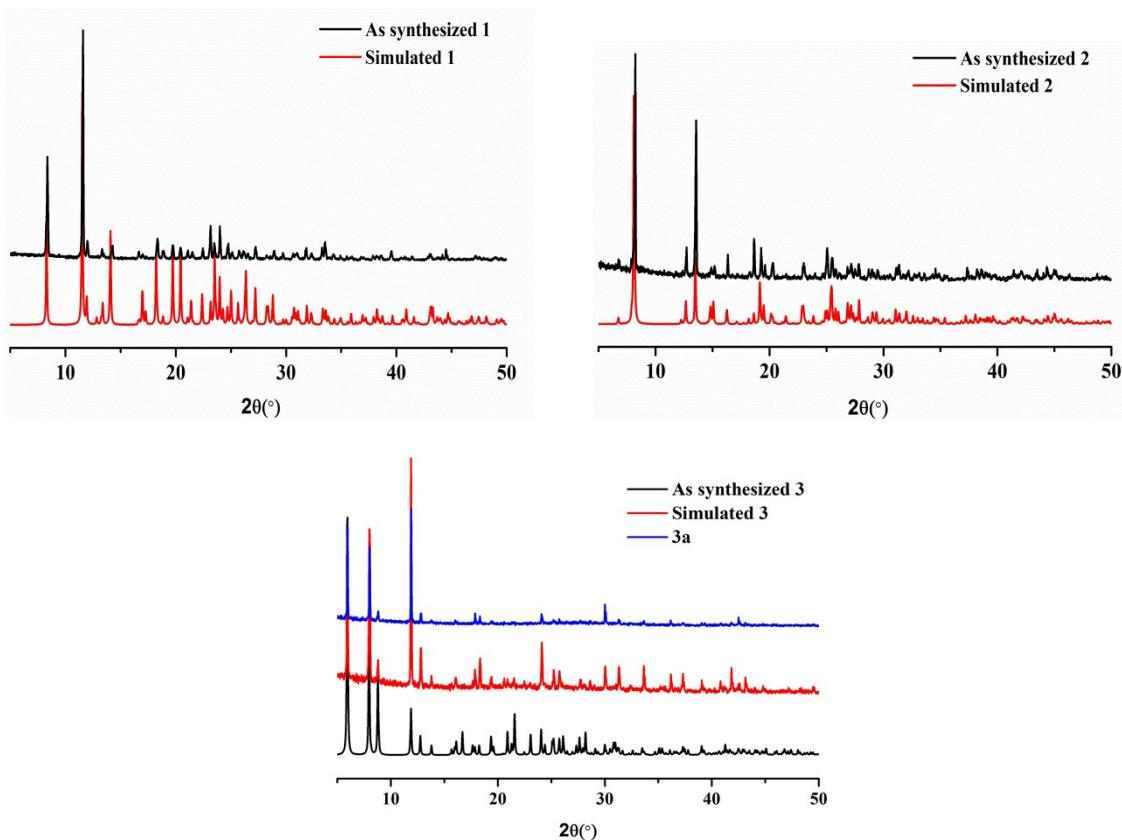
**Figure S5** PXRD patterns of the as-synthesized 1 - 3.
