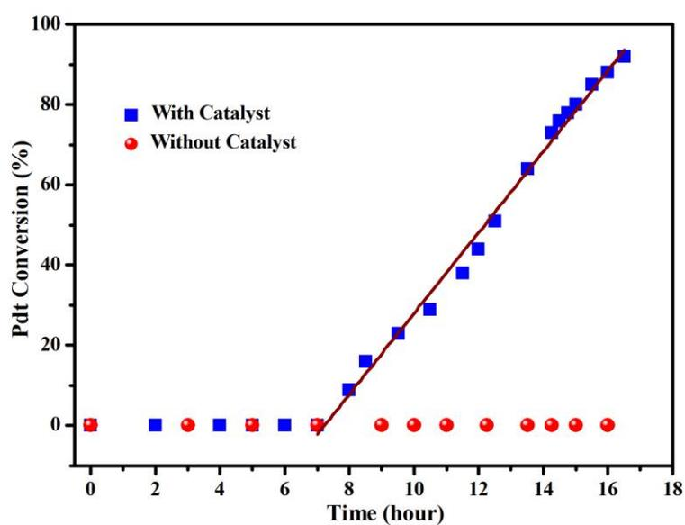
**Figure S3.** Effect of catalyst on the reaction profile: catalyzed vs uncatalyzed reaction of anisole bromination.
