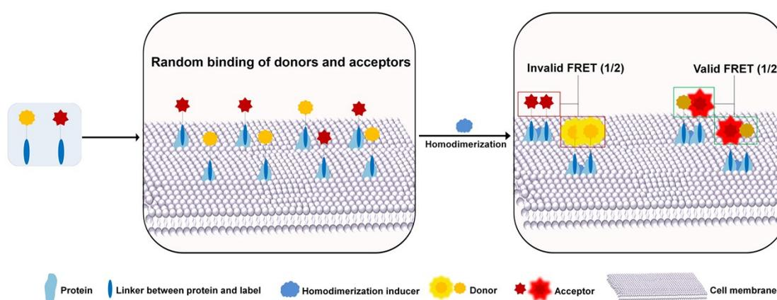
**Fig. S1** Schematic illustration of the classical FRET-based methods for protein homodimerization detection in which half homodimeric proteins lead to FRET-invalid label combinations.
