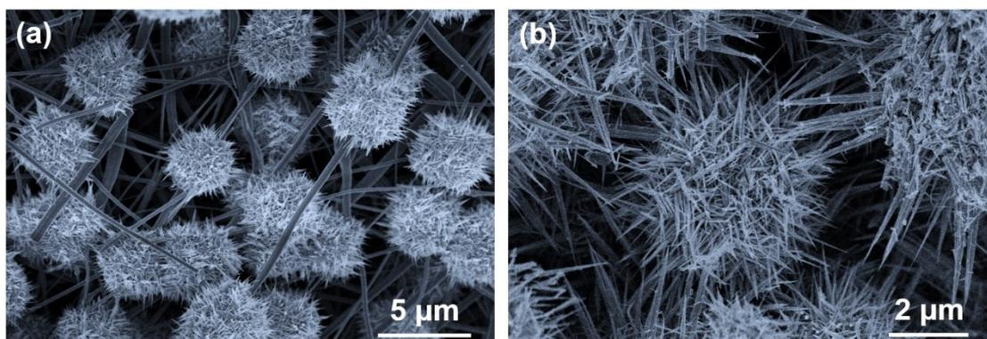
**Figure S10.** (a) Low- and (b) high-magnification SEM images of P-doped  $\text{WO}_3@\text{TiO}_2$  nanofibrous membrane after 12 h electrolysis at  $-0.55$  V vs. RHE.
