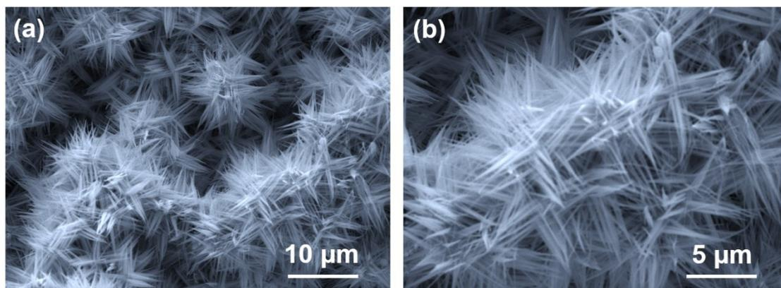
**Figure S2.** (a) Low- and (b) high-magnification SEM images of nanoneedle-constructed  $\text{WO}_3$  flowers fixed on  $\text{TiO}_2$  nanofibrous membrane.
