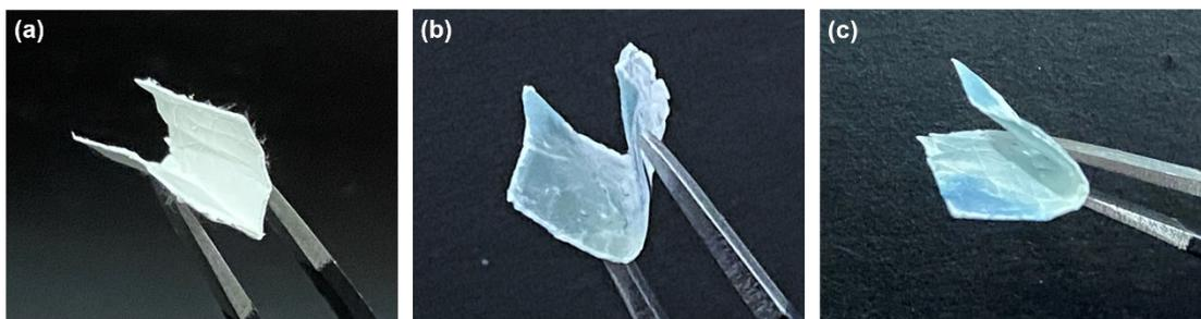
**Figure S3.** Digital images of (a)  $\text{TiO}_2$ , (b)  $\text{WO}_3@\text{TiO}_2$  and (c)  $\text{P-WO}_3@\text{TiO}_2$  nanofibrous membranes showing their excellent robustness and flexibility.
