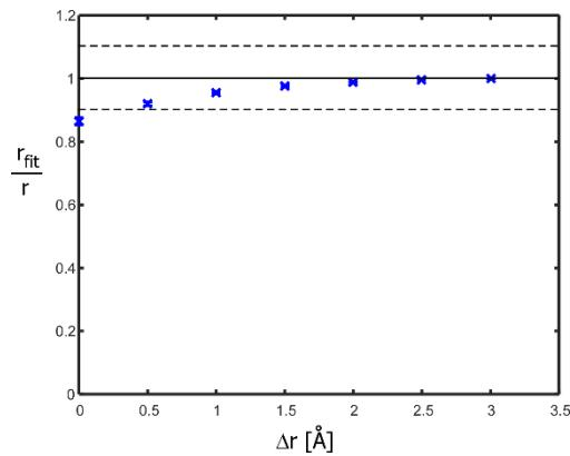
**Figure S3:** Split-PM-RESPDOR recoupling curves for a spin-1/2 coupled to a spin-3/2 having a nuclear quadrupolar coupling constant of 200 MHz.  $D=130$  Hz, the gap is  $26.3\mu\text{s}$ , PM pulse lengths are  $10T_R$  for the red squares,  $100T_R$  for the blue crosses. The solid line is the analytical Bessel function for a spin-3/2 shown in Eq. 1 of the main article.
