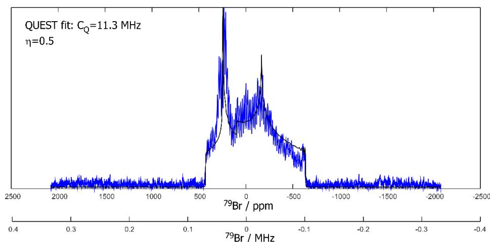
$^{79}\text{Br}$  WURST-QCPMG spectrum of tetra-n-butylammonium bromide (TBAB).  $C_Q=12.6$  MHz,  $\eta=0.16$ . For  $^{81}\text{Br}$ ,  $C_Q=10.5$  MHz.
