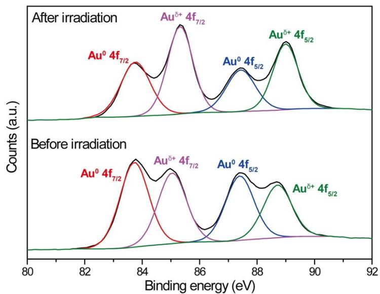
**Figure S9** Au 4f XPS spectra of porous gold nanoshells before and after laser irradiation (355 nm, 6 mJ/cm<sup>2</sup>). Each spectrum has been deconvoluted *via* the Gaussian fitting.
