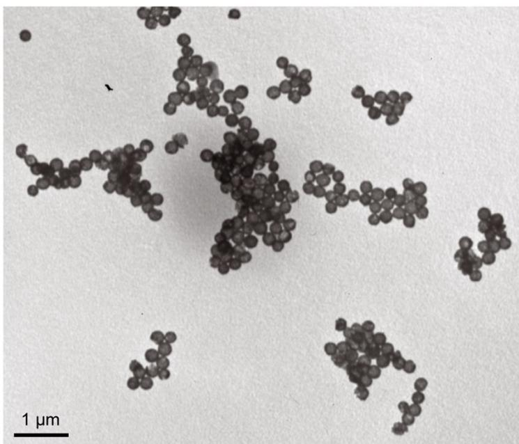
**Figure S7** Low-resolution TEM image acquired after the core  $\text{SiO}_2$  etching of irradiated porous gold nanoshells. The irradiation was conducted with 355 nm laser pulses at a fluence of  $4 \text{ mJ/cm}^2$  after the addition of PVP.
