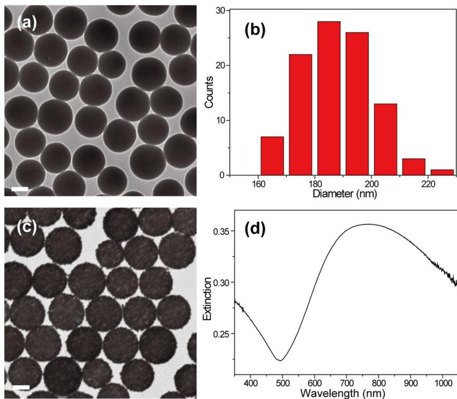
**Figure S1** Preparation of porous gold nanoshells. (a) TEM image and (b) size distribution of core SiO<sub>2</sub> nanoparticles. (c) TEM image and (d) UV-vis extinction spectrum of porous gold nanoshells (scale bars: 100 nm).
