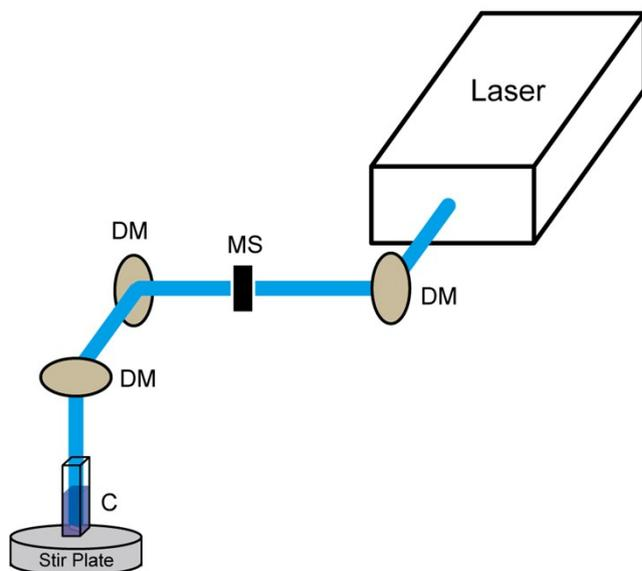
**Figure S2** Schematic of the laser irradiation setup for the structural modification of porous gold nanoshells (DM, dichroic mirror; MS, mechanical shutter; C, cell). Laser pulses of 355 nm or 532 nm were irradiated for 10 min.
