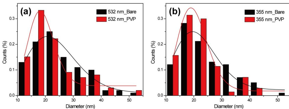
**Figure S6** Size distribution of gold nanospheres, which were generated by  $6 \text{ mJ/cm}^2$  pulses under the indicated conditions.
