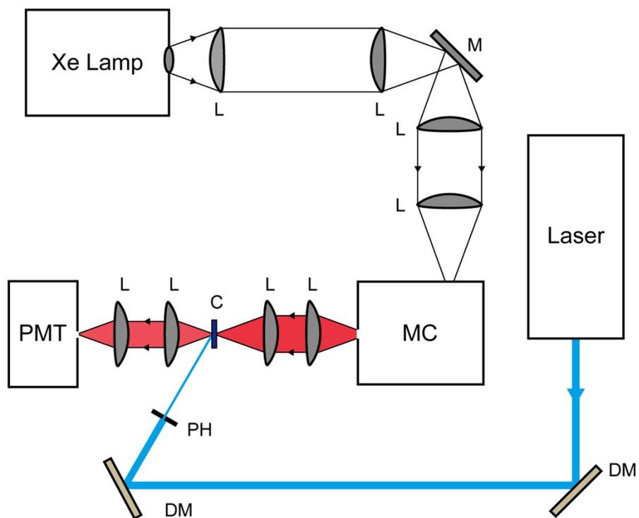
**Figure S3** Schematic illustration for the experimental setup of the transient-absorption measurement (L, lense; M, mirror; MC, monochromator; DM, dichroic mirror; PH, pinhole; C, cell; PMT, photomultiplier tube).
