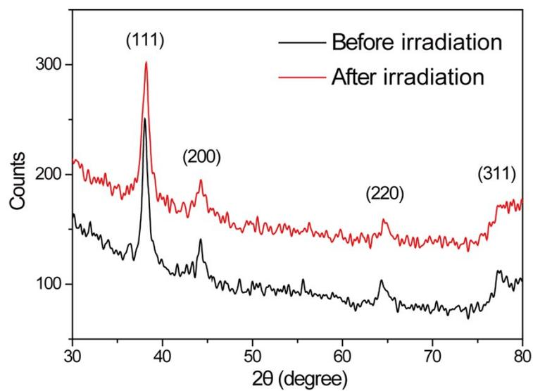
**Figure S5** XRD patterns of porous gold nanoshells before and after laser irradiation (355 nm, 6 mJ/cm<sup>2</sup>).
