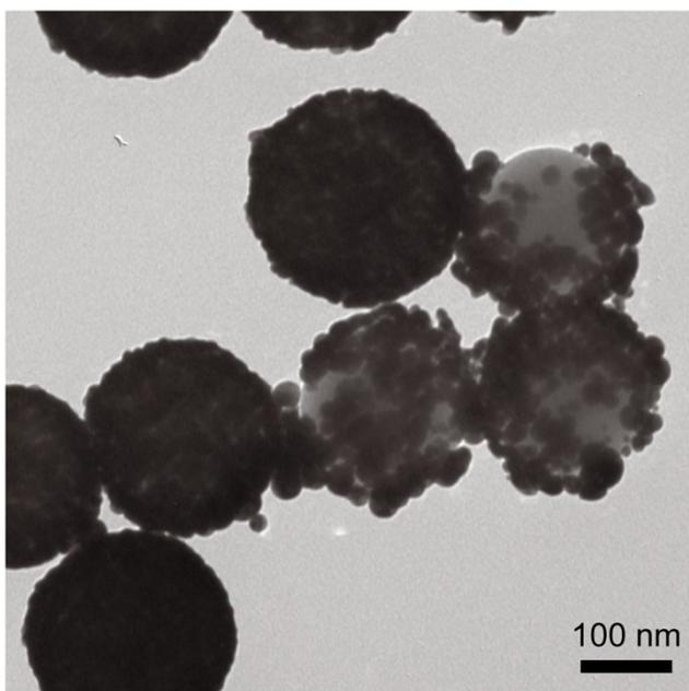
**Figure S4** TEM image of porous gold nanoshells irradiated with 532 nm pulses at a fluence of 5 mJ/cm<sup>2</sup>.
