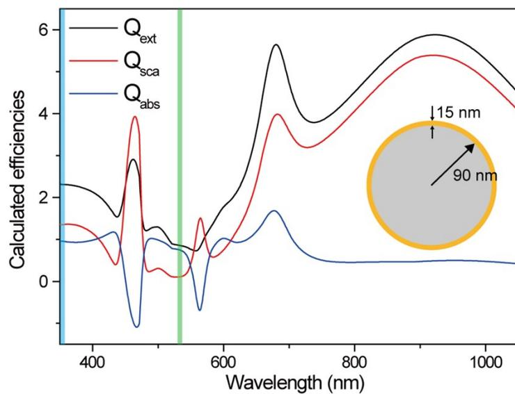
**Figure S8** The extinction, absorption and scattering spectra of gold nanoshells supported on  $\text{SiO}_2$  cores, simulated using the Mie calculation. The  $\text{SiO}_2$  core radius and the gold shell thickness were set to be 90 nm and 15 nm, respectively.
