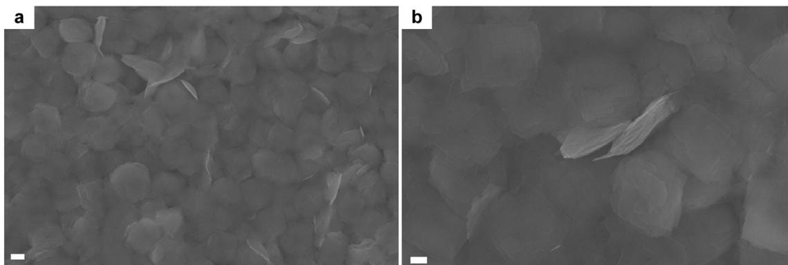
**Fig. S2** SEM images of BiOCl-UCNP from (a) low magnification and (b) high magnification. The scale bars for (a) and (b) are 200 and 100 nm respectively.
