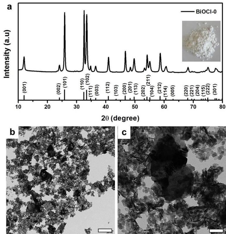
**Fig. S1** (a) The PXRD pattern of BiOCl nanoplates synthesized without using dual-surfactants (PSS and PVP) in the reaction system (denoted as BiOCl-0). Inset is the corresponding powder of BiOCl-0; representing its white color. (b) Low- and (c) high- magnification TEM images of BiOCl-0. The scale bars for (b) and (c) are 200 and 50nm respectively.
