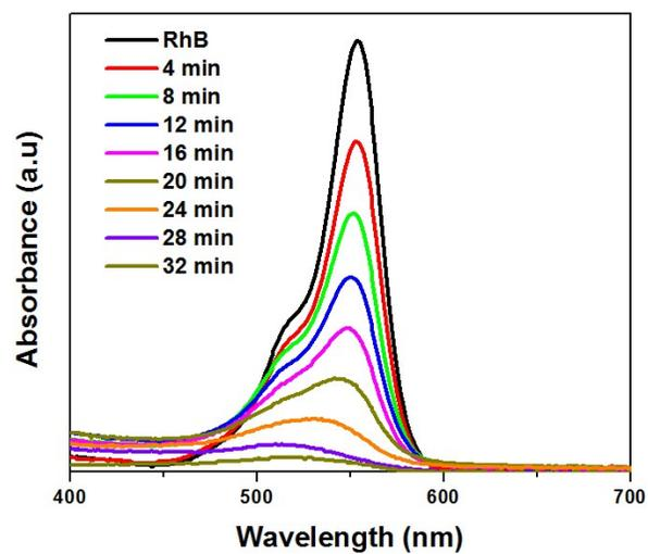
**Fig. S5** Temporal absorption spectra of the RhB solution degraded with BiOCl-UCNP under the exposure of natural sunlight. This result confirmed the potential of BiOCl-UCNP for real solar-driven applications.
