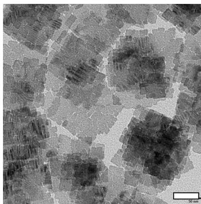
**Fig. S4** TEM image of BiOCl-UCNP observed, after using it for 8 consecutive cycles of photodegradation; displaying that BiOCl-UCNP are highly stable and retained its morphology during multi-cycles of degradation. The scale bar is 50 nm.
