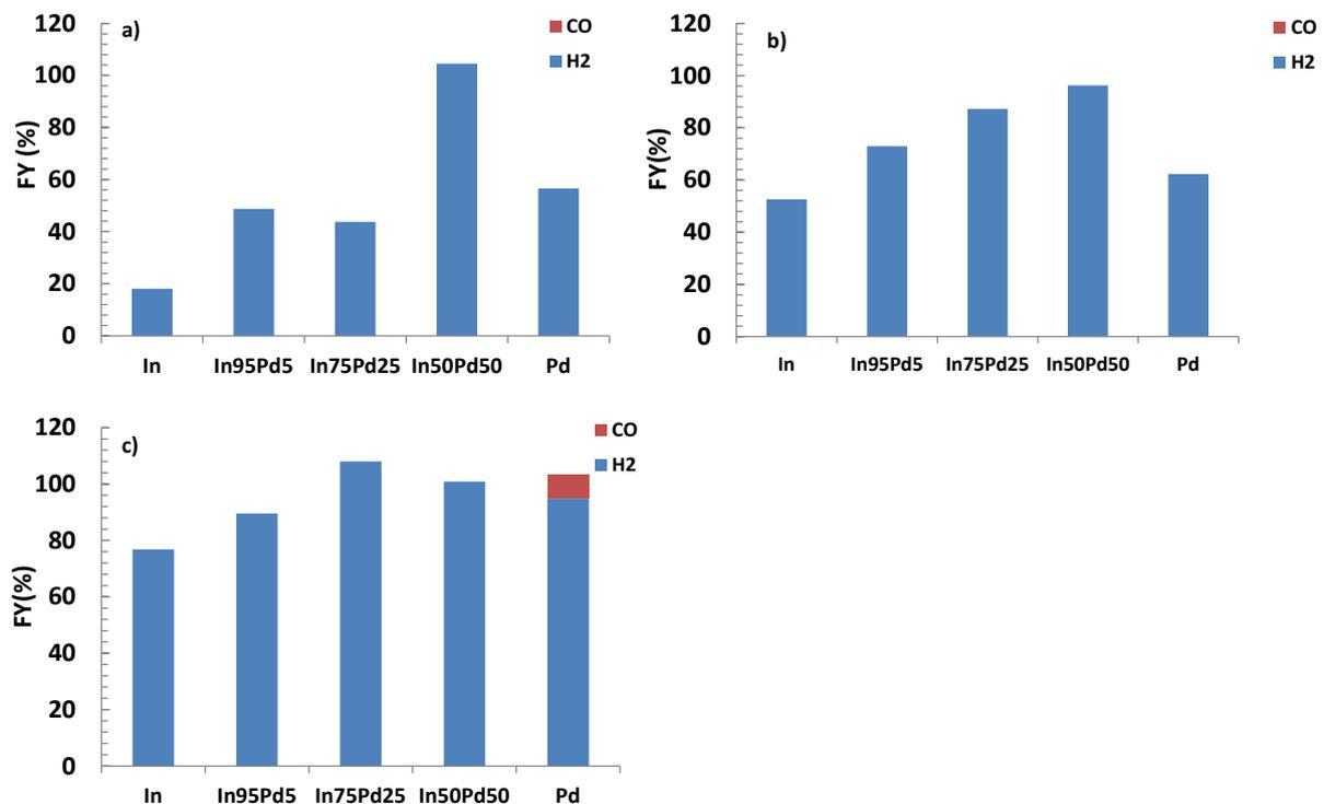
Figure S.I. 7 FY to gaseous products on the 5 catalysts at a) -0.5V vs RHE; b) -1V vs RHE and c) -1.5V vs RHE. Considering the contribution from formate to the FY (main manuscript) Pd at -0.5V and -1V gives FY lower
