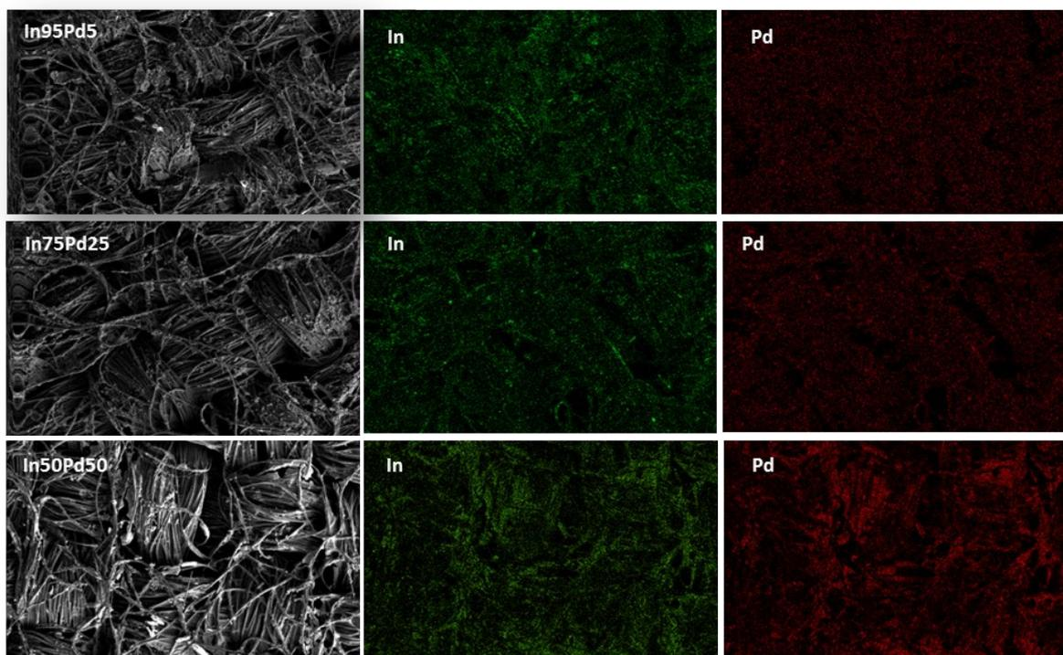
Figure S.I. 1 Elemental distribution in bimetallic catalysts. In and Pd are homogeneously dispersed on the carbon cloth.
