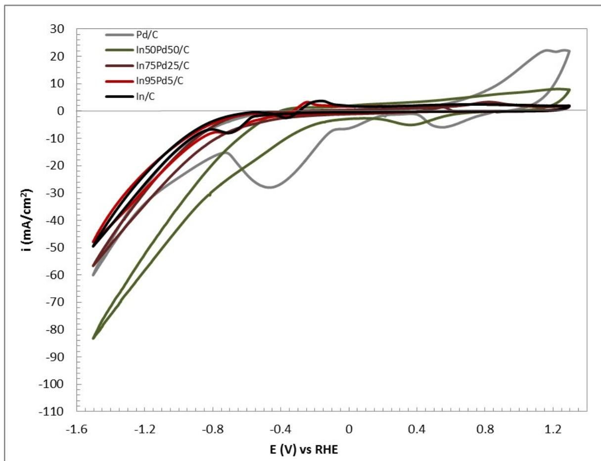
Figure S.I. 5 Cyclic voltammeteries of the 5 catalysts in CO<sub>2</sub> saturated KHCO<sub>3</sub>.
