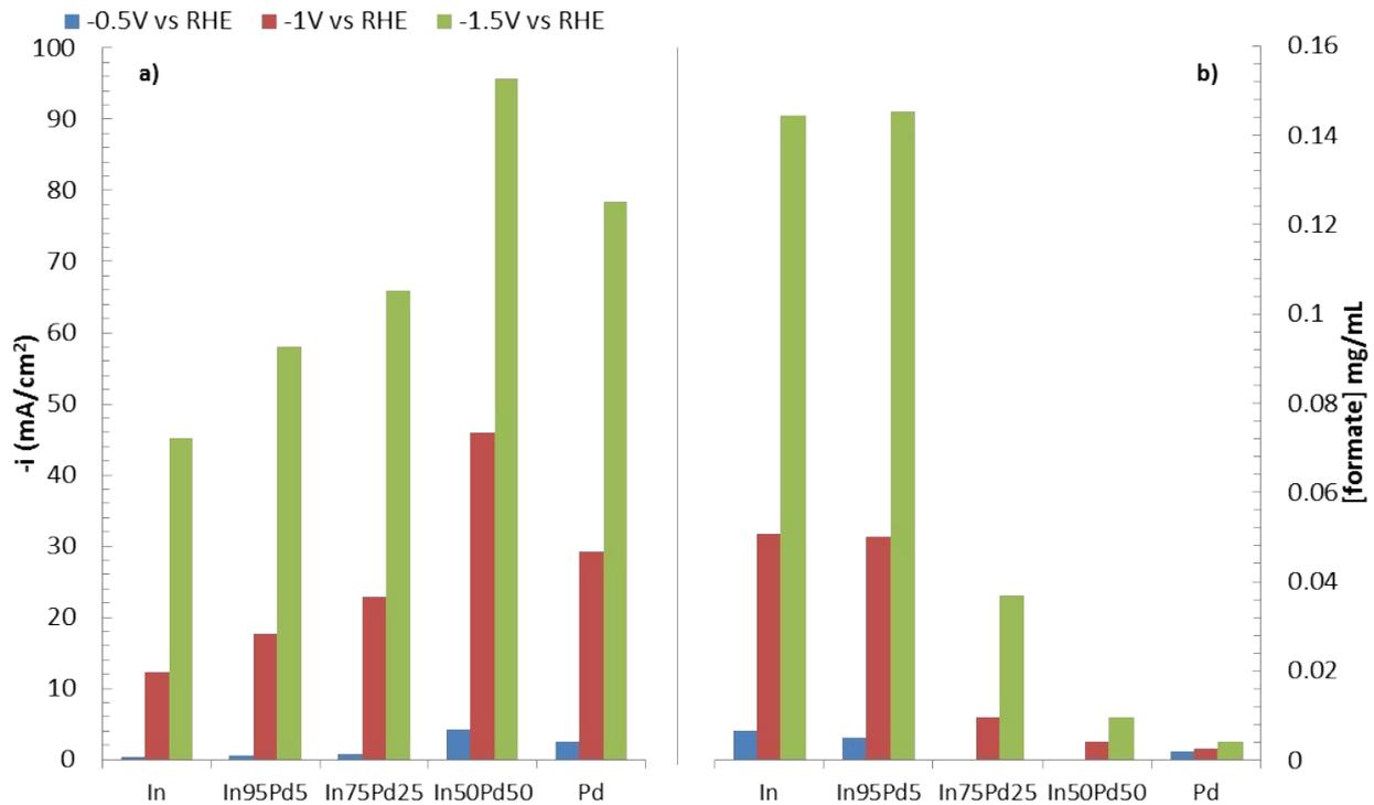
Figure S.I. 6 a) Current densities during the bulk electrolysis at the different potentials on all the catalysts. b) Concentrations of formate in mg/mL at the end of every 30 minute potential step for all the catalysts. In In95Pd5 the productivity of formate is the same as pure In, but the current is higher, resulting in a lower faradaic yield (see Figure 4 in the main manuscript).
