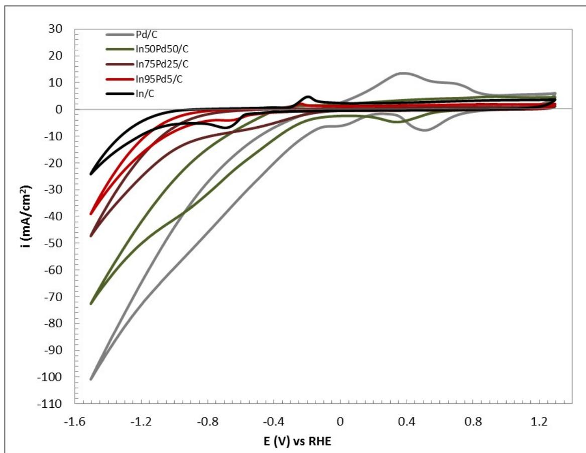
Figure S.I. 4 Cyclic voltammeteries of the 5 catalysts in  $N_2$  saturated 0.5M  $KHCO_3$ . Notice how the onset potential of HER shifts positively and results in higher currents. Also, the shape of the CVs, especially in In50Pd50/C and In75Pd25/C is dramatically changed and doesn't show characteristic peaks of either In or Pd.
