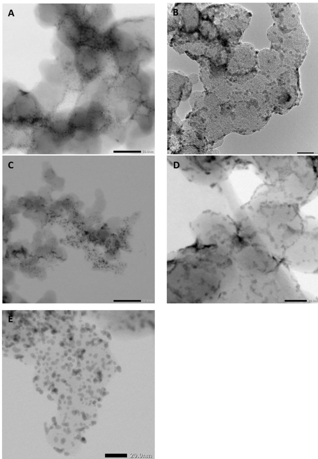
**Figure S.I. 2** Some TEM pictures of (A) In/C, (B) In<sub>50</sub>Pd<sub>50</sub>/C, (C) In<sub>75</sub>Pd<sub>25</sub>/C, (D) In<sub>95</sub>Pd<sub>5</sub>/C and (E) Pd/C nanoparticles. ( Scale bar A, C = 50 nm; scale bar B, D, E = 20 nm)
