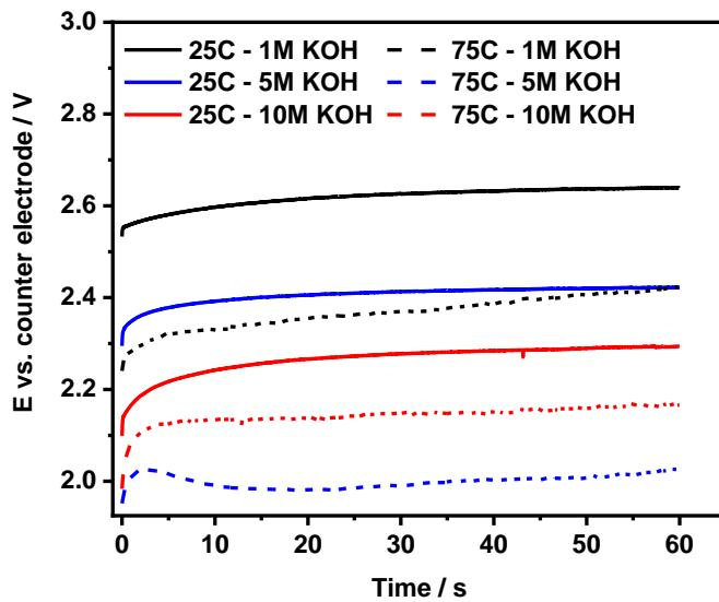
Figure S3. Chronopotentiograms of NiFeO<sub>x</sub>H<sub>y</sub> conducted at  $j = 100 \text{ mA cm}^{-2}$  at different temperatures and KOH concentrations.
