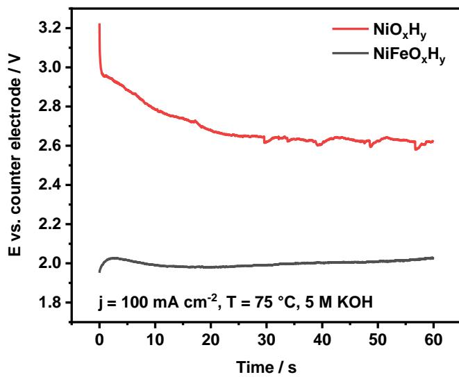
Figure S10. Chronopotentiograms of  $\text{NiO}_x\text{H}_y$  (red) and  $\text{NiFeO}_x\text{H}_y$  (black) conducted at  $j = 100 \text{ mA cm}^{-2}$ ,  $75^\circ\text{C}$ ,  $5 \text{ M KOH}$ .
