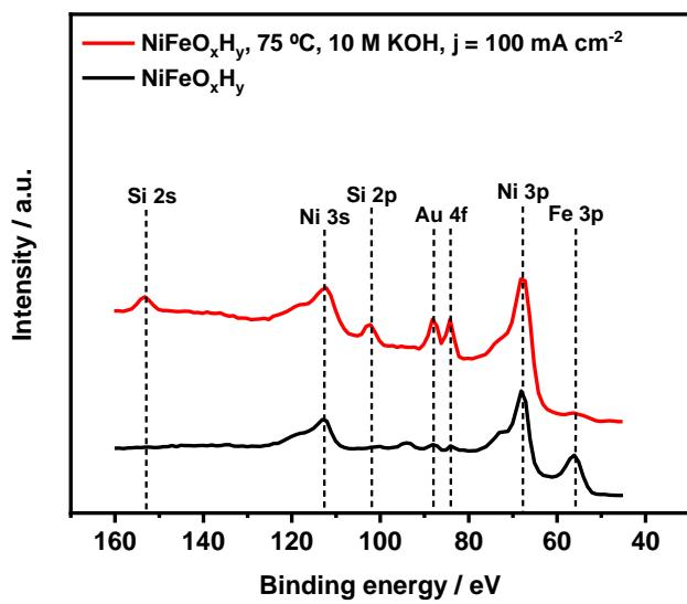
Figure S8. Low-binding energy region of XPS survey scan of NiFeO<sub>x</sub>H<sub>y</sub> before and after anodic polarization at 75 °C in 10 M KOH,  $j = 100 \text{ mA cm}^{-2}$ .
