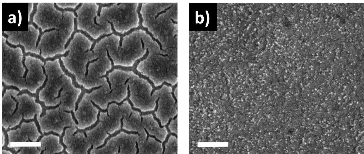
Figure S12. SEM images of  $\text{NiO}_x\text{H}_y$  a) before and b) after anodic polarization at 75 °C in 5 M KOH,  $j = 100 \text{ mA cm}^{-2}$ , 1 h. Scale bars are equal to 500 nm.
