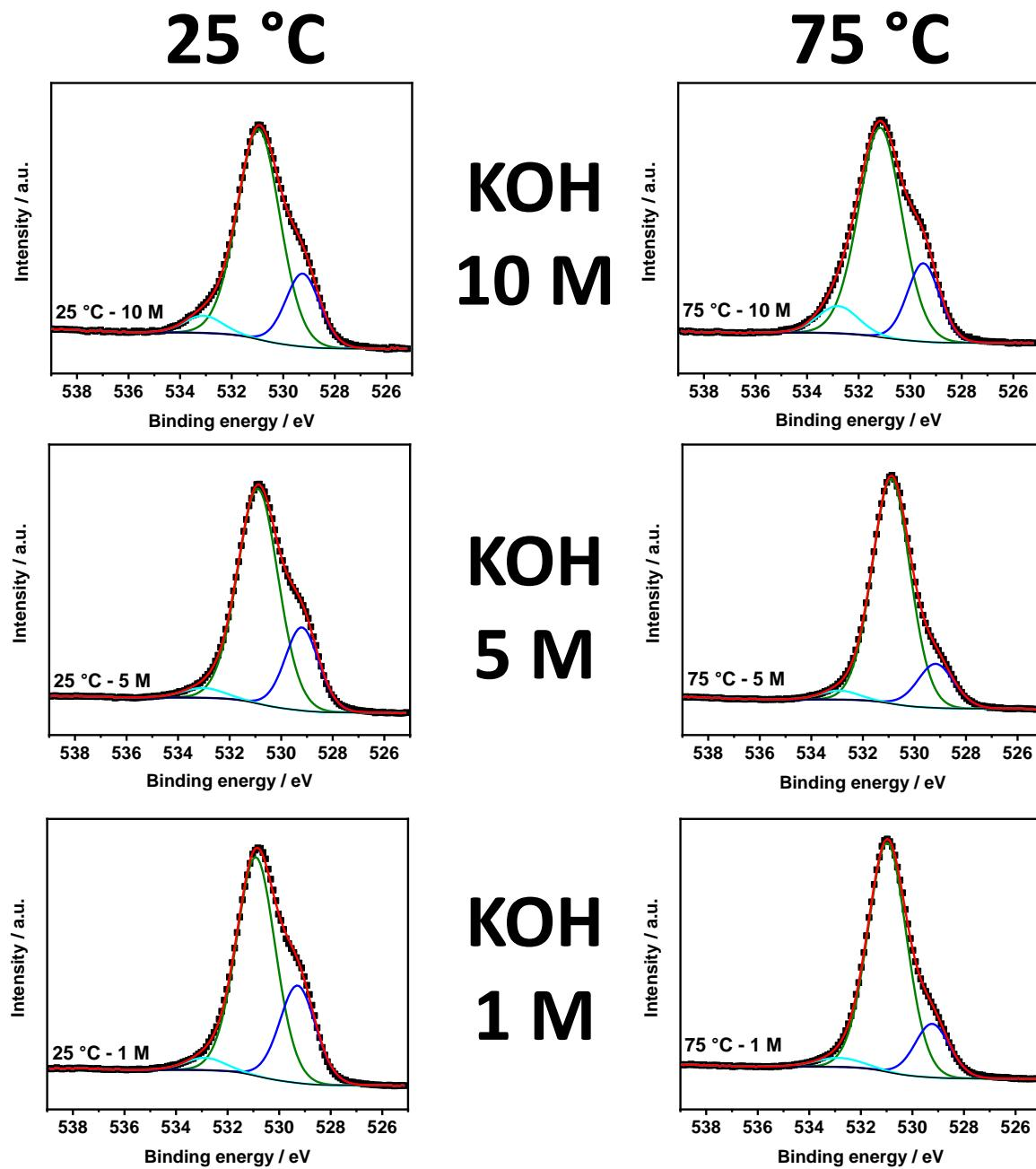
Figure S7. O 1s spectra of NiFeO<sub>x</sub>H<sub>y</sub> samples after the stability tests performed under different conditions.
