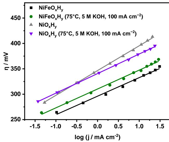
Figure S11. iR-corrected Tafel plots of  $\text{NiO}_x\text{H}_y$  and  $\text{NiFeO}_x\text{H}_y$  before and after anodic polarization at 75 °C in 5 M KOH,  $j = 100 \text{ mA cm}^{-2}$ . Measurements were carried out in 1 M KOH at 25 °C; the dots represent the experimental data, the lines represent the fittings.
