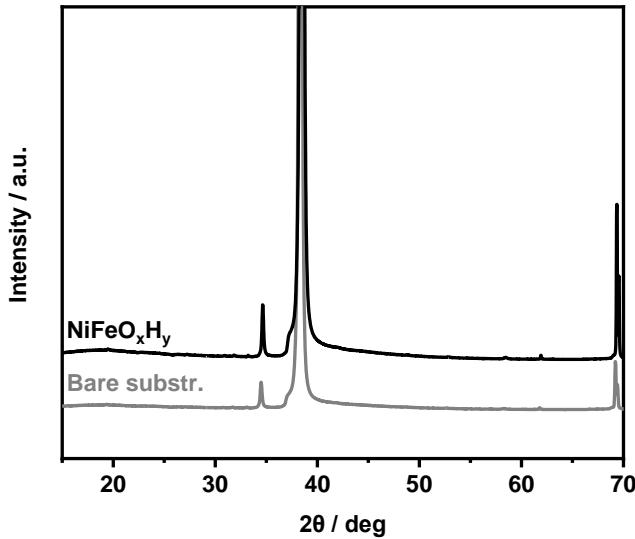
Figure S2. XRD patterns of fresh supported NiFeO<sub>x</sub>H<sub>y</sub> sample and bare Au-coated Si substrate.
