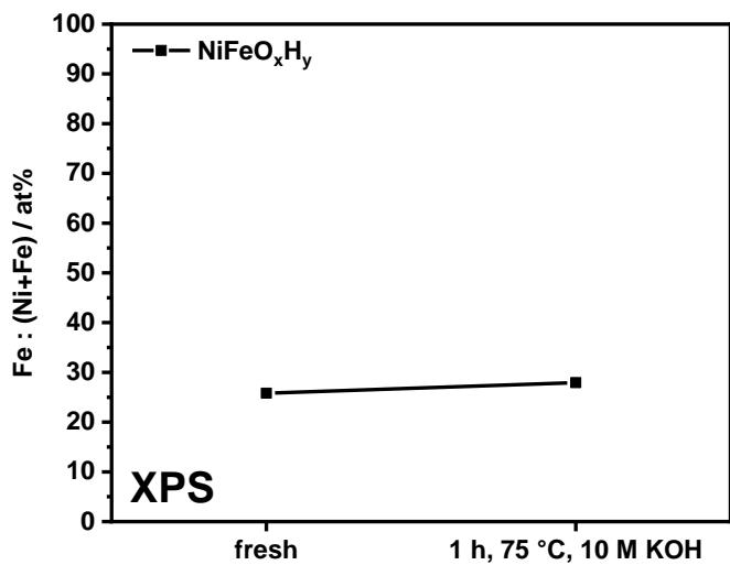
Figure S4. XPS analysis of fresh NiFeO<sub>x</sub>H<sub>y</sub> and after 1 hour of immersion in 10 M KOH at 75 °C without anodic polarization.
