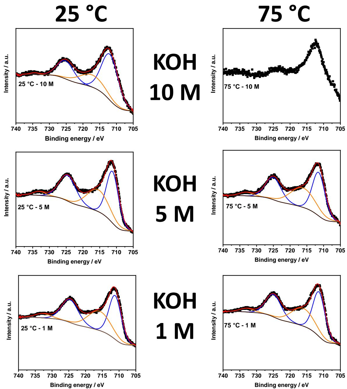
Figure S6. Fe 2p spectra of  $\text{NiFeO}_x\text{H}_y$  samples after the stability tests performed under different conditions. For the sample tested at 75 °C in 10 M KOH, no peak fitting was performed, because of the strong intensity of the Ni Auger LMM feature overlapping with the weak Fe 2p<sub>3/2</sub> peak for this low Fe-containing sample.
