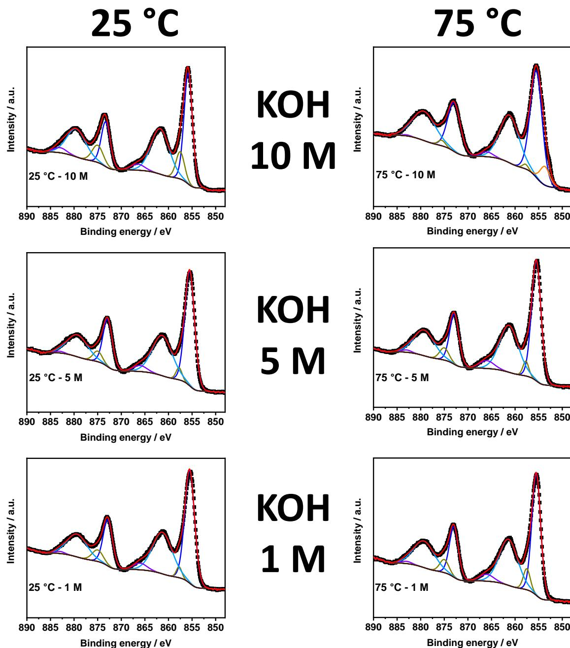
Figure S5. Ni 2p spectra of NiFeO<sub>x</sub>H<sub>y</sub> samples after the stability tests performed under different conditions.
