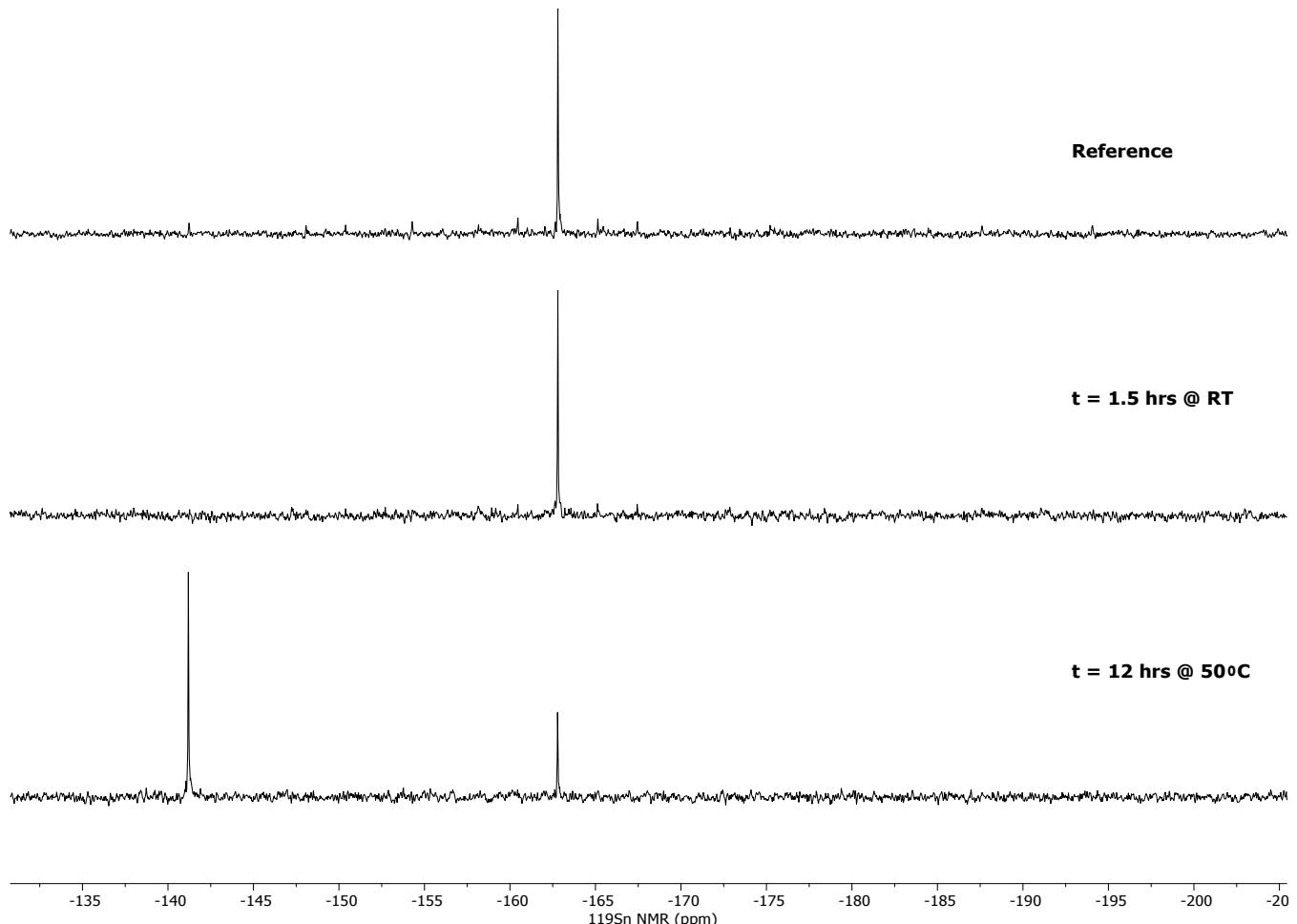
Figure S36. Stacked  $^{119}\text{Sn}$ (decoupled) NMR spectra of  $\text{Ph}_3\text{SnH}$  with **1** (5 mol%) in  $\text{C}_6\text{D}_6$  with increasing temperature over time.
