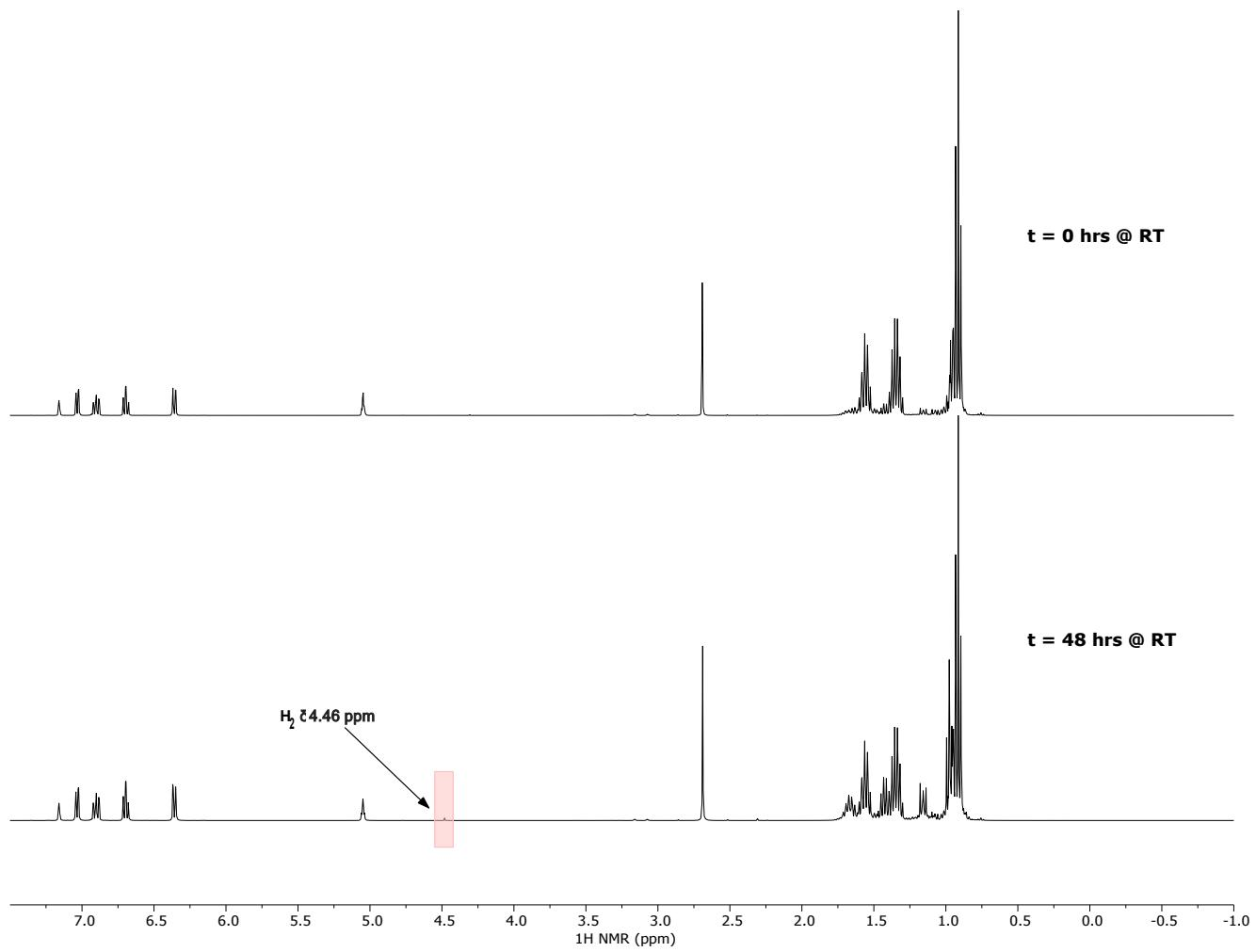
Figure S22. Stacked  $^1\text{H}$  NMR spectra of  $\text{Bu}_3\text{SnH}$  with *N*-methylphenothiazine (10 mol%) in  $\text{C}_6\text{D}_6$  at room temperature.
