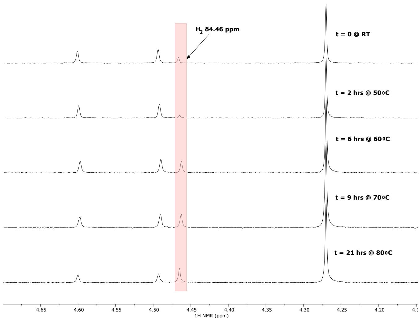
Figure S18. Stacked  $^1\text{H}$  NMR spectra of  $\text{Ph}_3\text{SnH}$  with **1** (1 eq.) in  $\text{C}_6\text{D}_6$  with increasing temperature over time; expanded region.
