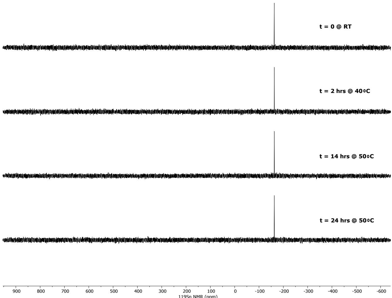
Figure S25. Stacked  $^{119}\text{Sn}$ (decoupled) NMR spectra of  $\text{Ph}_3\text{SnH}$  in  $\text{C}_6\text{D}_6$  at  $50^\circ\text{C}$  over time.
