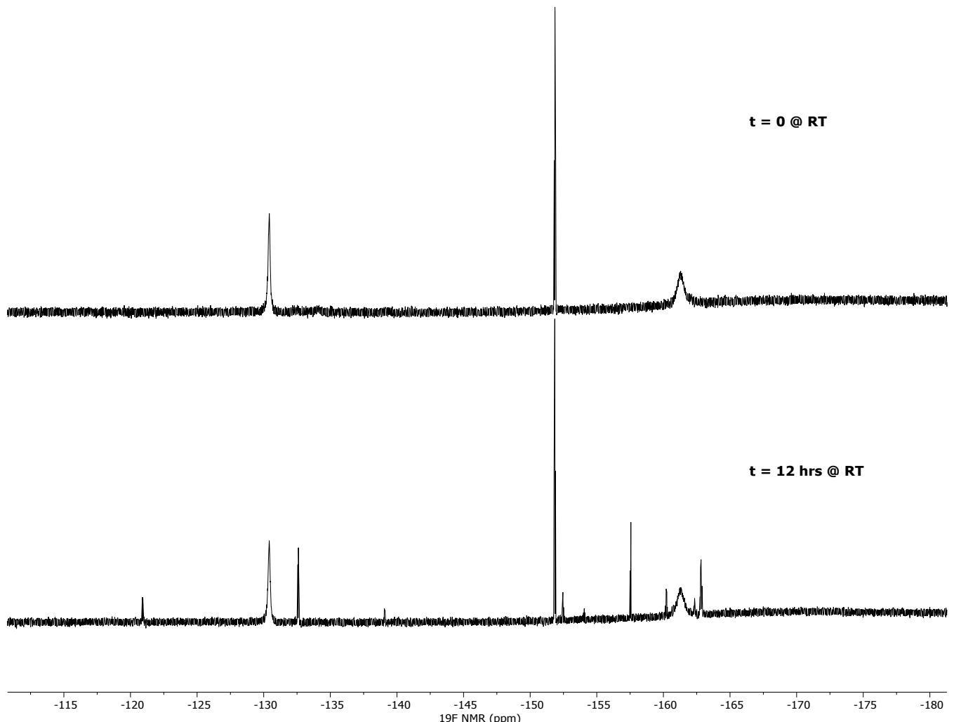
Figure S39. Stacked  $^{19}\text{F}$  NMR spectra of  $\text{Bu}_3\text{SnH}$  with **1** (5 mol%) in  $\text{C}_6\text{D}_6$  at room temperature over time.
