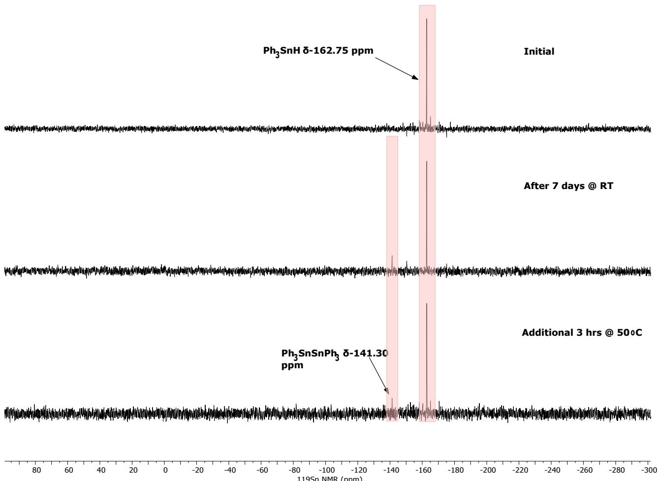
Figure S15. Stacked  $^{119}\text{Sn}$ (decoupled) NMR spectra of  $\text{Ph}_3\text{SnH}$  with **1** (1 eq.) and  $\text{Mes}_3\text{P}$  (1 eq.) in  $\text{C}_6\text{D}_6$  at ambient temperature over time.
