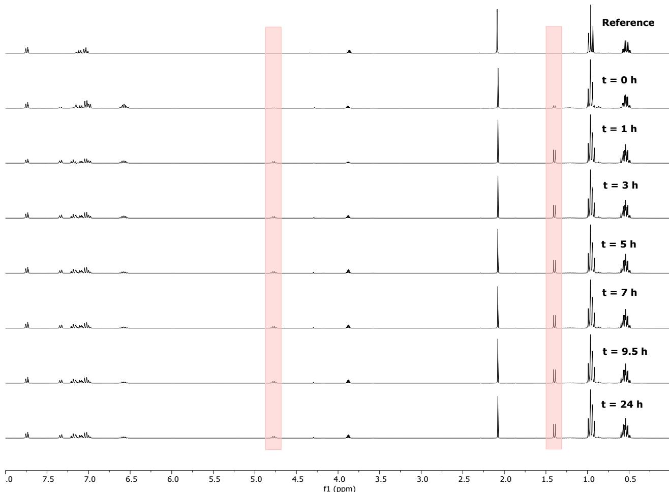
Figure S11. Stacked  $^1\text{H}$  NMR spectra of  $\text{Et}_3\text{SiH}$  (1.1 eq.) and acetophenone (1 eq.) with **1** (10 mol%) in  $\text{C}_6\text{D}_6$  (dilute).
