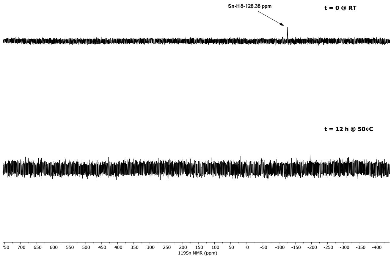
Figure S33. Stacked <sup>119</sup>Sn NMR spectra of  $\text{Ph}_3\text{SnH}$  with  $\text{HB}(\text{C}_6\text{F}_5)_2$  (1 eq.) in  $\text{C}_6\text{D}_6$  at 50 °C over time.
