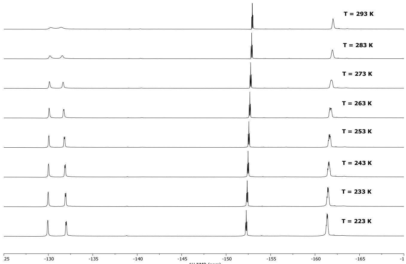
Figure S6. Stacked Variable Temperature <sup>19</sup>F NMR spectra of **1** in  $\text{CD}_2\text{Cl}_2$  from 293 K to 223 K.
