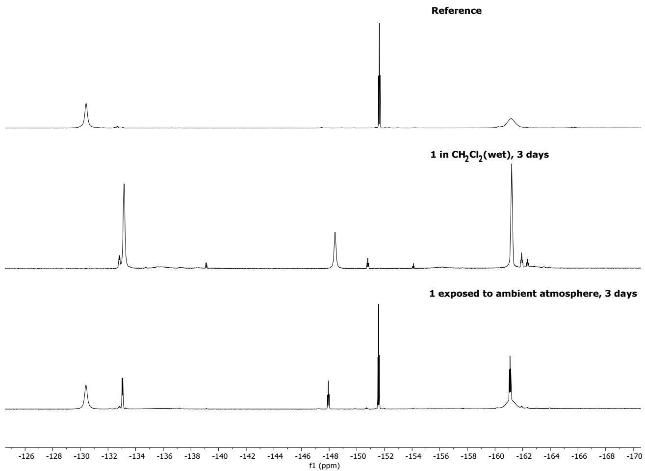
Figure S9. Stacked  $^{19}\text{F}$  NMR spectra of **1** exposed to wet solvent (middle) and ambient atmosphere (bottom) in  $\text{C}_6\text{D}_6$ .
