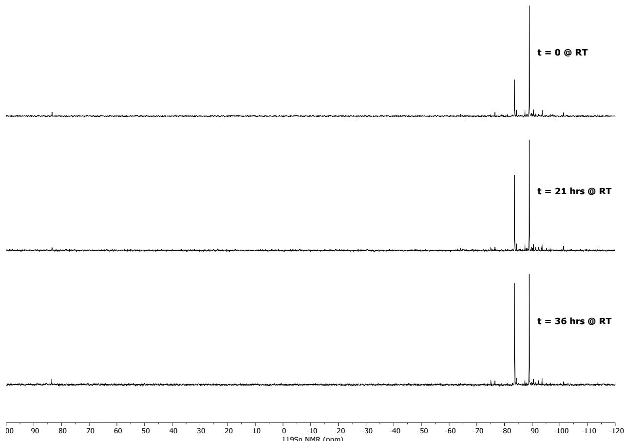
Figure S38. Stacked  $^{119}\text{Sn}$ (decoupled) NMR spectra of  $\text{Bu}_3\text{SnH}$  with **1** (5 mol%) in  $\text{C}_6\text{D}_6$  at room temperature over time.
