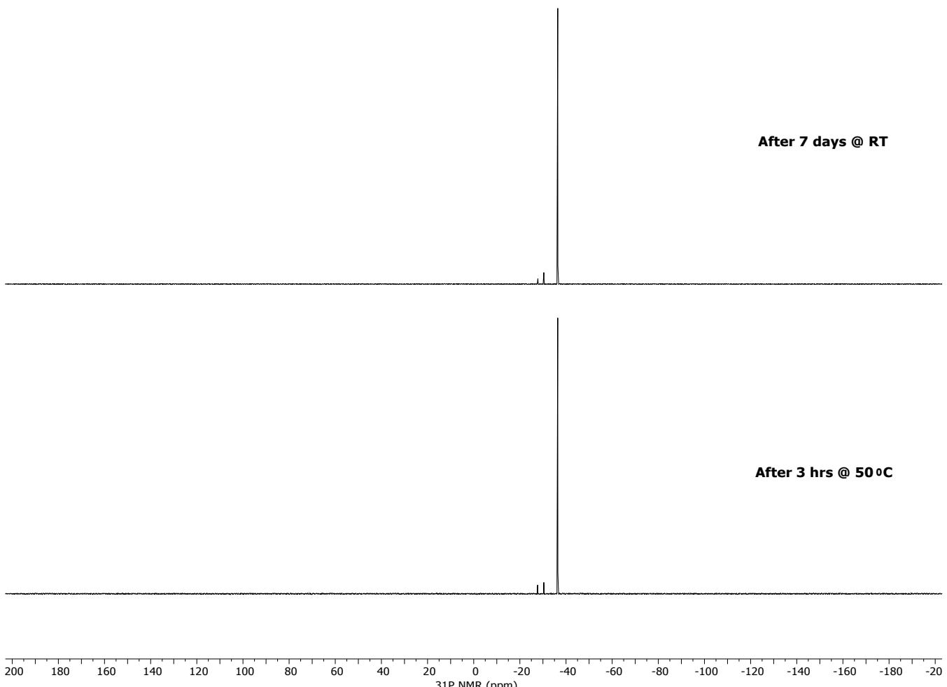
Figure S16. Stacked  $^{31}\text{P}$ (decoupled) NMR spectra of  $\text{Ph}_3\text{SnH}$  with **1** (1 eq.) and  $\text{Mes}_3\text{P}$  (1 eq.) in  $\text{C}_6\text{D}_6$  at ambient temperature over time.
