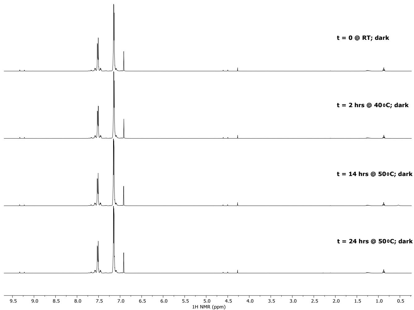
Figure S24. Stacked <sup>1</sup>H NMR spectra of Ph<sub>3</sub>SnH in C<sub>6</sub>D<sub>6</sub> at 50 °C over time.
