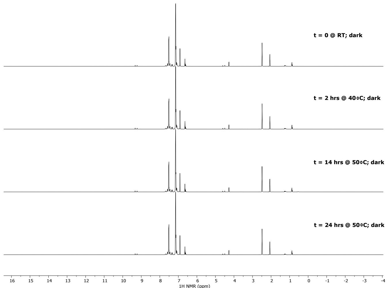
Figure S26. Stacked <sup>1</sup>H NMR spectra of Ph<sub>3</sub>SnH with N-dimesitylboryl-phenothiazine (10 mol%) in C<sub>6</sub>D<sub>6</sub> at 50 °C over time.
