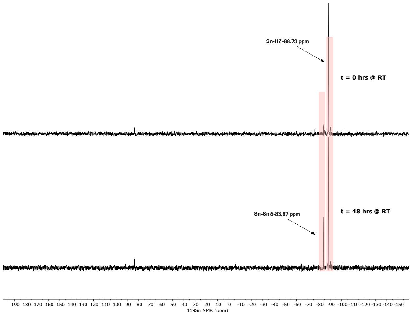
Figure S23. Stacked  $^{119}\text{Sn}$ (decoupled) NMR spectra of  $\text{Bu}_3\text{SnH}$  with N-methylphenoxythiazine (10 mol%) in  $\text{C}_6\text{D}_6$  at room temperature.
