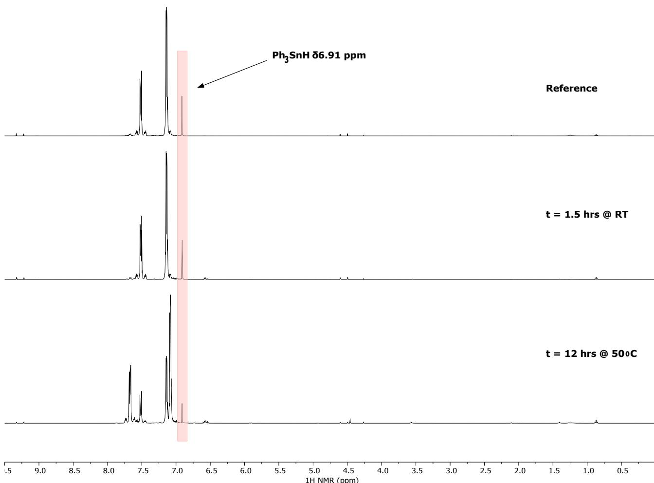
Figure S34. Stacked  $^1H$  NMR spectra of  $Ph_3SnH$  with **1** (5 mol%) in  $C_6D_6$  with increasing temperature over time.
