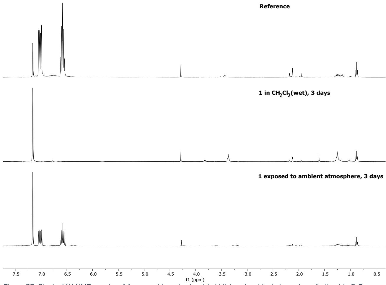
Figure S7. Stacked  $^1\text{H}$  NMR spectra of **1** exposed to wet solvent (middle) and ambient atmosphere (bottom) in  $\text{C}_6\text{D}_6$ .
