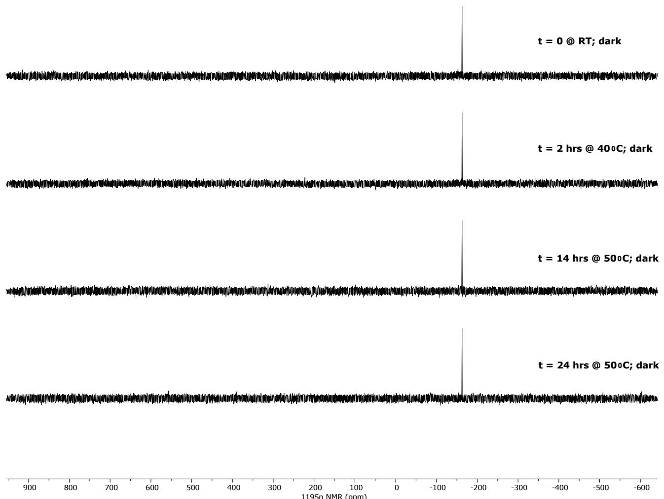
Figure S27. Stacked  $^{119}\text{Sn}$ (decoupled) NMR spectra of  $\text{Ph}_3\text{SnH}$  with *N*-dimesitylboryl-phenothiazine (10 mol%) in  $\text{C}_6\text{D}_6$  at 50 °C over time.
