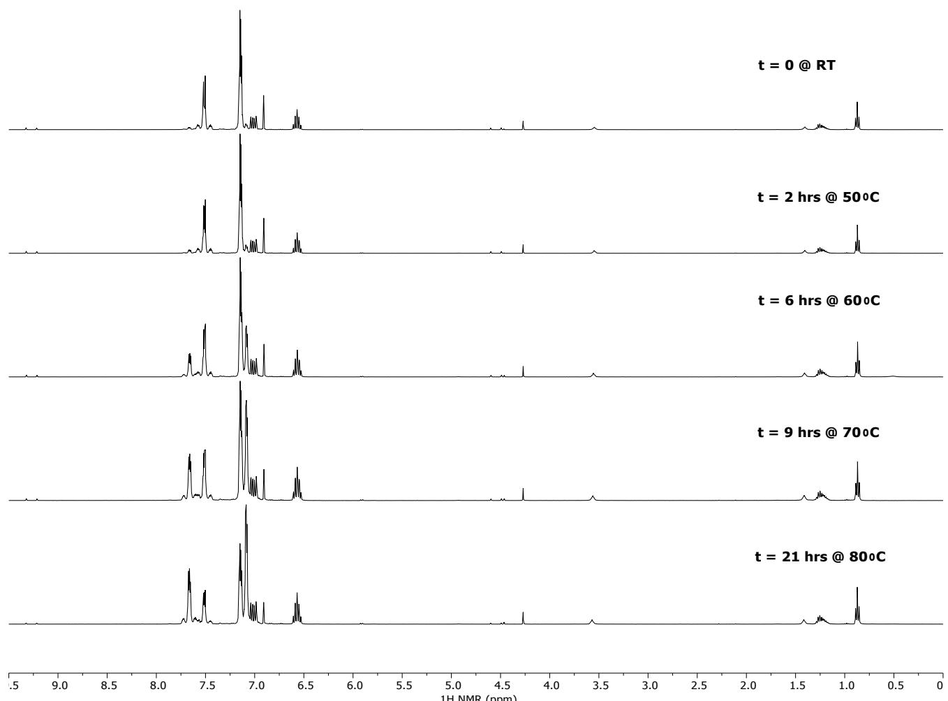
Figure S17. Stacked <sup>1</sup>H NMR spectra of Ph<sub>3</sub>SnH with **1** (1 eq.) in C<sub>6</sub>D<sub>6</sub> with increasing temperature over time.
