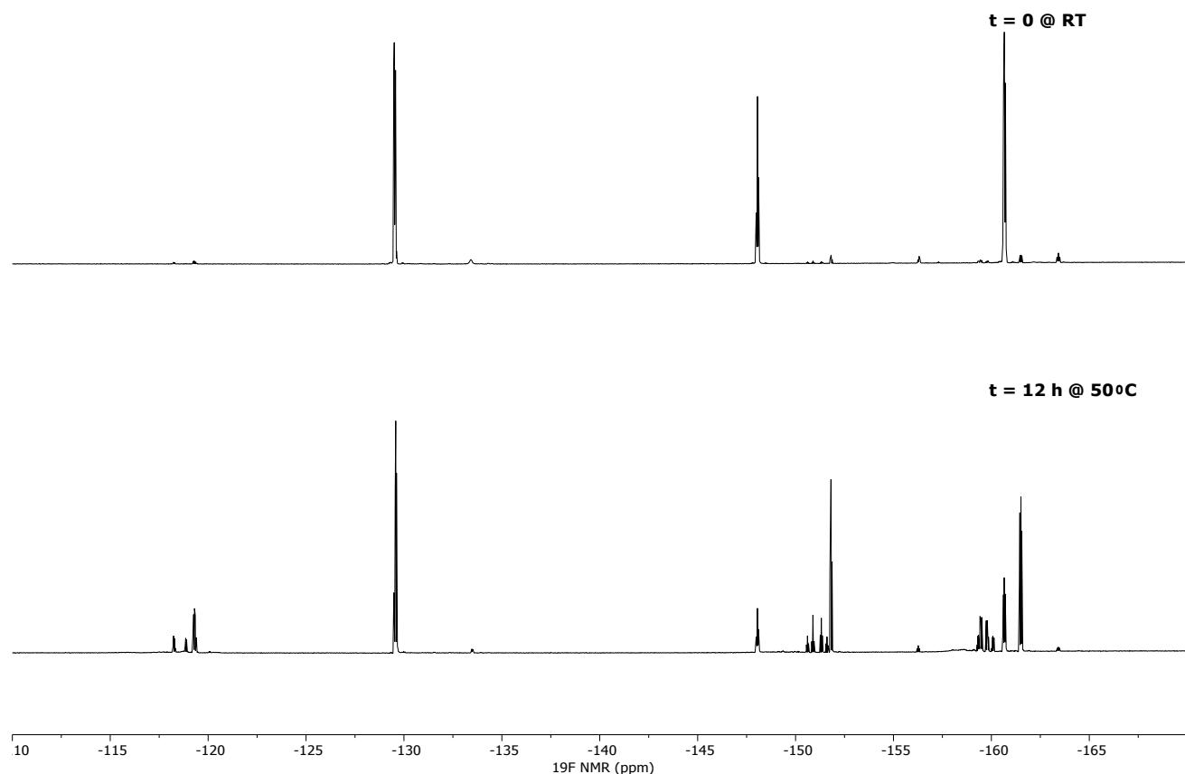
Figure S32. Stacked  $^{19}\text{F}$  NMR spectra of  $\text{Ph}_3\text{SnH}$  with  $\text{HB}(\text{C}_6\text{F}_5)_2$  (1 eq.) in  $\text{C}_6\text{D}_6$  at  $50^\circ\text{C}$  over time.
