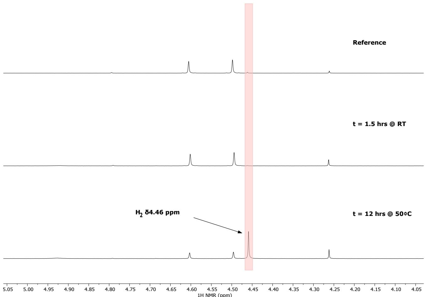
Figure S35. Stacked <sup>1</sup>H NMR spectra of Ph<sub>3</sub>SnH with **1** (5 mol%) in C<sub>6</sub>D<sub>6</sub> with increasing temperature over time; expanded region.
