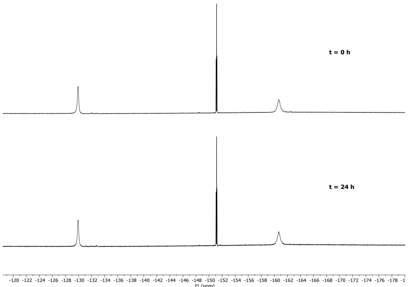
Figure S12. Stacked  $^{19}\text{F}$  NMR spectra of  $\text{Et}_3\text{SiH}$  (1.1 eq.) and acetophenone (1 eq.) with **1** (10 mol%) in  $\text{C}_6\text{D}_6$  (dilute).
