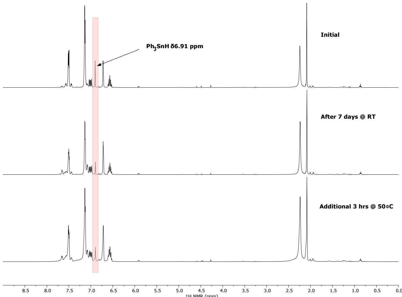
Figure S13. Stacked  $^1\text{H}$  NMR spectra of  $\text{Ph}_3\text{SnH}$  with **1** (1 eq.) and  $\text{Mes}_3\text{P}$  (1 eq.) in  $\text{C}_6\text{D}_6$  at ambient temperature over time.
