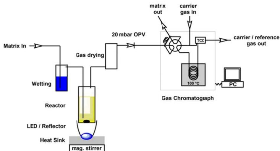
**Scheme S2.** Representation of the setup for photocatalysis experiments with in-line H<sub>2</sub> detection
