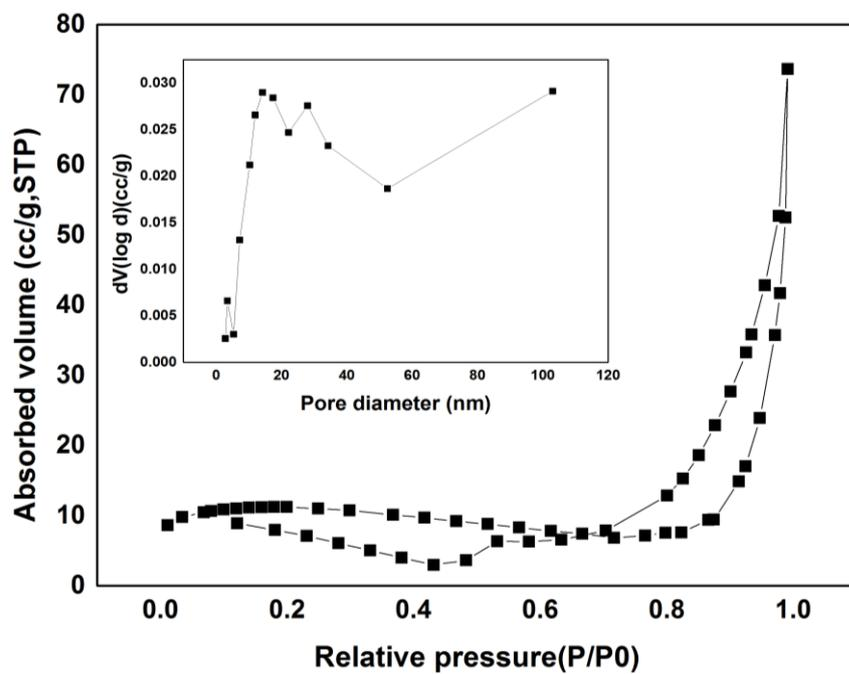
Fig. S3. N<sub>2</sub> adsorption–desorption isotherms of samples: (a) C/Si, (b) PG/Si/Ni. The inset in each figure shows the relevant pore size distribution calculated by the BJH formula.
