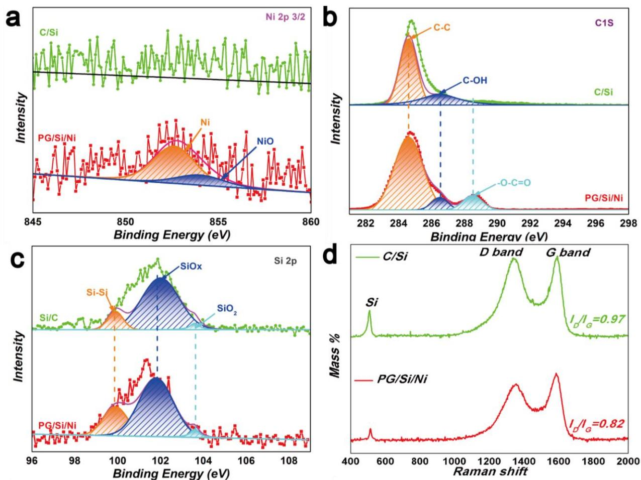
Fig. S1. High-resolution XPS spectra of the C/Si and PG/Si/Ni: (a) Ni 2p<sub>3/2</sub>, (b) Si 2p,
