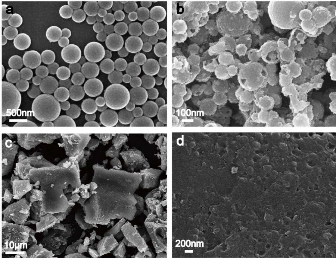
Fig. S2. SEM images of (a) as-prepared SiO<sub>2</sub> nanospheres. (c) as-prepared Si nanospheres. (b,c) C/Si composite.
