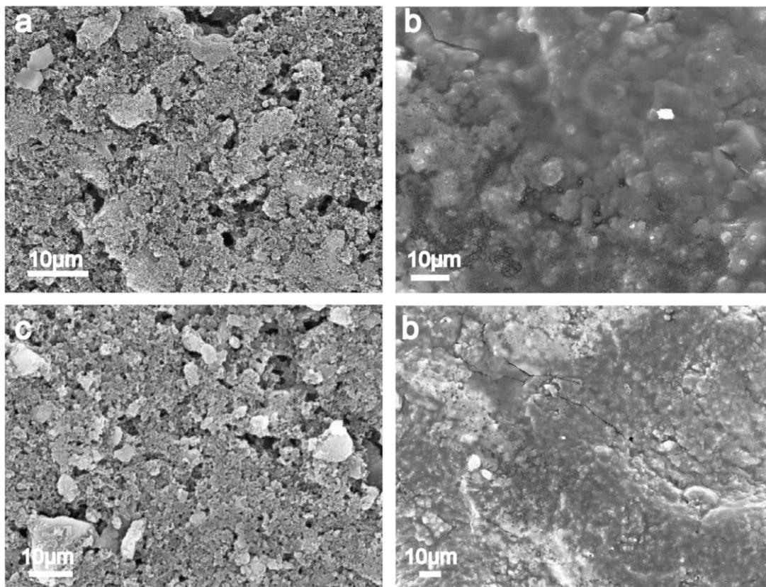
Fig. S4. SEM images of C/Si composite, (a) before cycling, and (b) after 2000 cycles; SEM images of PG/Si/Ni hybrid composite, (c) before cycling and (d) after 2000 cycles.
