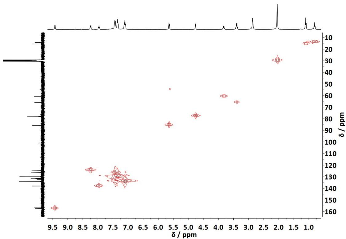
Figure S10 - HSQC NMR spectrum of  $[\text{Ru}(\eta^5\text{-C}_5\text{H}_4\text{COOCH}_2\text{CH}_3)(2,2'\text{-bipy})][\text{CF}_3\text{SO}_3]$  (**3**) in  $(\text{CD}_3)_2\text{CO}$ .
