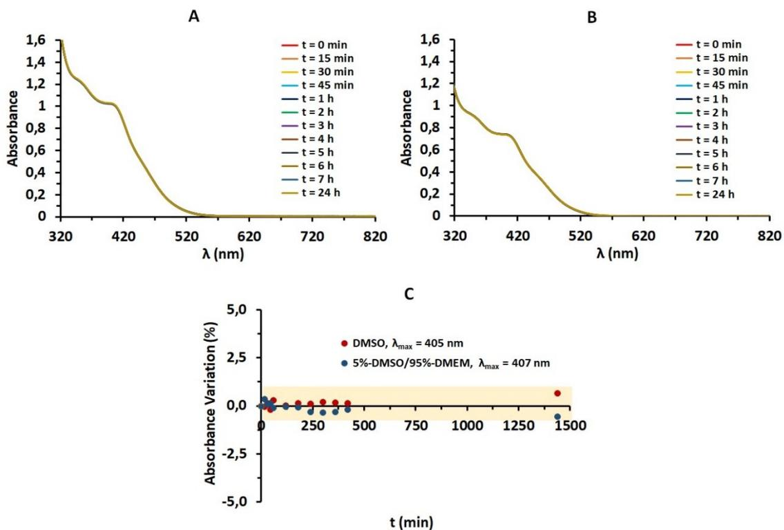
**Figure S26** - Stability of  $[\text{Ru}(\eta^5\text{-C}_5\text{H}_4\text{COOH})(\text{PPh}_3)(2,2'\text{-bipy})][\text{CF}_3\text{SO}_3]$  (TM281) in solution over 24 hours: UV-visible spectra acquired from 0 min up to 24 h in DMSO at 280  $\mu\text{M}$  (A) and in 5%-DMSO/95%-DMEM+GlutaMAX-I™ at 200  $\mu\text{M}$  (B); variation of the maximum absorption observed at 405 nm in DMSO (•) and at 407 nm 5%-DMSO/95%-DMEM+GlutaMAX-I™ (•) along time (0 min to 1440 min = 24 h).
