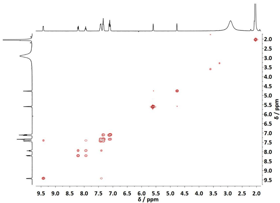
Figure S14 - COSY NMR spectrum of  $[\text{Ru}(\eta^5\text{-C}_5\text{H}_4\text{COOH})(2,2'\text{-bipy})][\text{CF}_3\text{SO}_3]$  (**TM281**) in  $(\text{CD}_3)_2\text{CO}$ .
