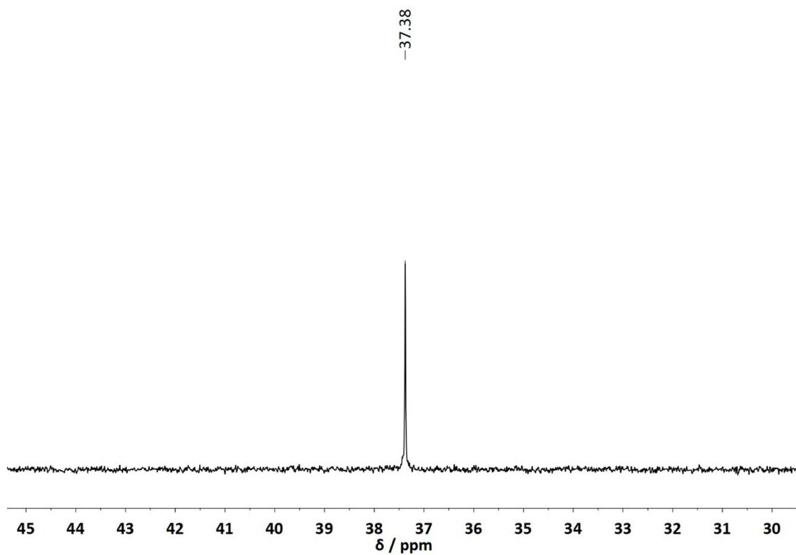
Figure S6 -  $^{31}\text{P}$  NMR spectrum of  $[\text{Ru}(\eta^5\text{-C}_5\text{H}_4\text{COOCH}_2\text{CH}_3)(\text{PPh}_3)_2\text{Cl}]$  (**2**) in  $\text{CDCl}_3$ .
