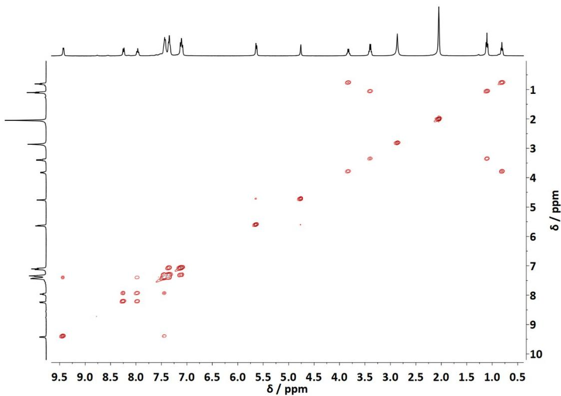
Figure S8 - COSY NMR spectrum of  $[\text{Ru}(\eta^5\text{-C}_5\text{H}_4\text{COOCH}_2\text{CH}_3)(2,2'\text{-bipy})][\text{CF}_3\text{SO}_3]$  (**3**) in  $(\text{CD}_3)_2\text{CO}$ .
