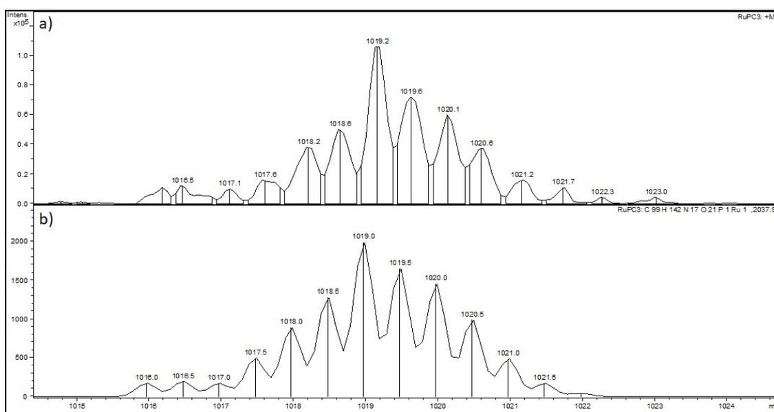
**Figure S25** - Observed (a) and simulated (b) ESI-MS Spectra of RuPC-3 (Ru-PEG(3)- VSPPLTLGQLLS)
