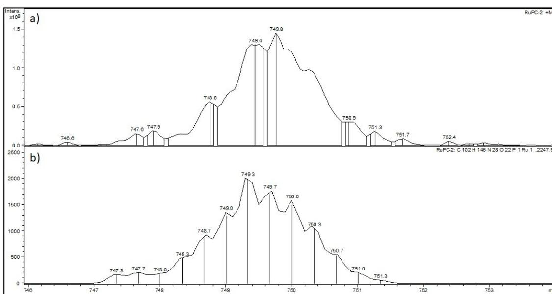
Figure S23 - Observed (a) and simulated (b) ESI-MS Spectra of RuPC-2 (Ru-PEG(3)- SRRPASFR(TARE))
