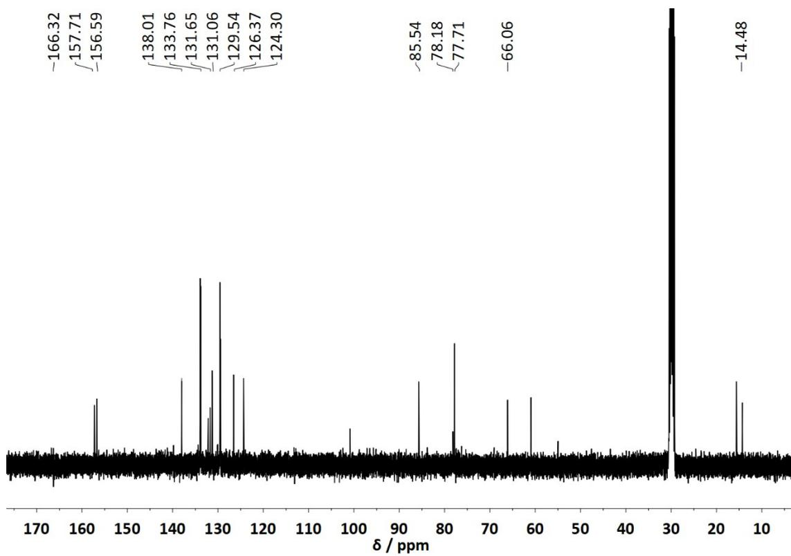
Figure S9 -  $^{13}\text{C}$  NMR spectrum of  $[\text{Ru}(\eta^5\text{-C}_5\text{H}_4\text{COOCH}_2\text{CH}_3)(2,2'\text{-bipy})][\text{CF}_3\text{SO}_3]$  (**3**) in  $(\text{CD}_3)_2\text{CO}$ .
