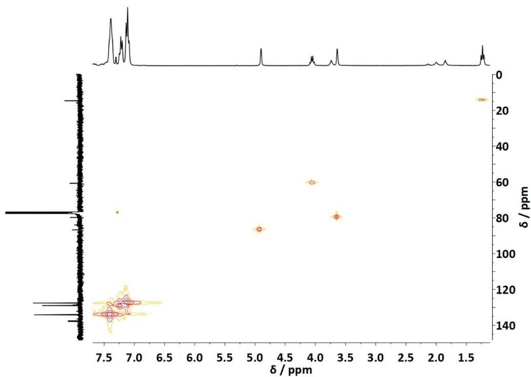
Figure S4 - HSQC NMR spectrum of  $[\text{Ru}(\eta^5\text{-C}_5\text{H}_4\text{COOCH}_2\text{CH}_3)(\text{PPh}_3)_2\text{Cl}]$  (**2**) in  $\text{CDCl}_3$ .
