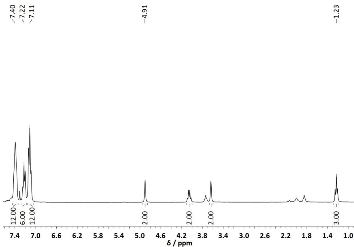
**Figure S1** -  $^1\text{H}$  NMR spectrum of  $[\text{Ru}(\eta^5\text{-C}_5\text{H}_4\text{COOCH}_2\text{CH}_3)(\text{PPh}_3)_2\text{Cl}]$  (**2**) in  $\text{CDCl}_3$ .
