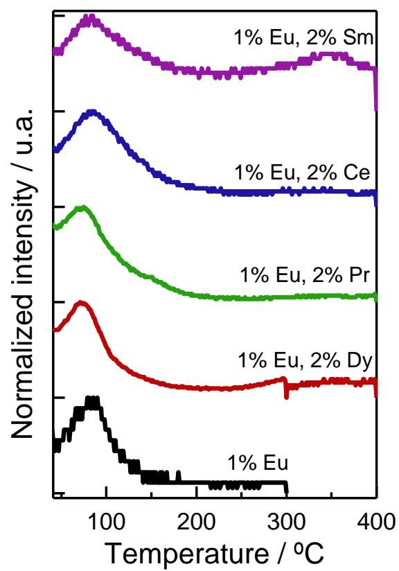
Fig. S4. Thermoluminescence glow curves of  $\text{SrS}:\text{Eu}^{2+},\text{RE}^{3+}$ .
