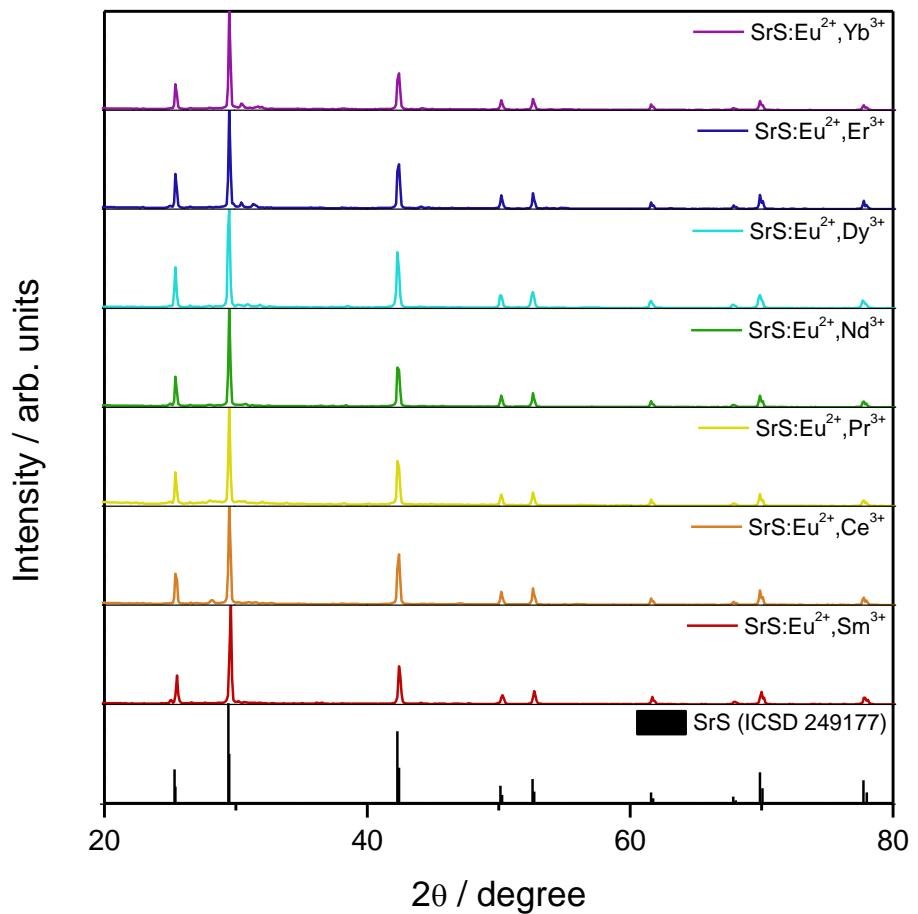
Fig S1. X-ray diffraction patterns of SrS:Eu<sup>2+</sup>,RE<sup>3+</sup> materials
