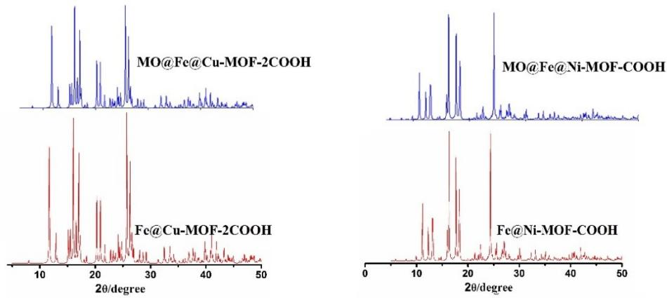
Fig. 4S. PXRD patterns recorded for both the post synthetically modified MOFs before and after adsorption of dye.
