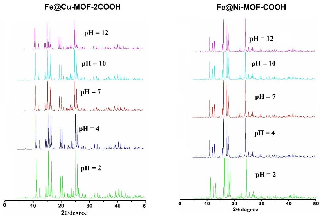
Fig. 5S. PXRD patterns recorded for both the post synthetically modified MOFs at varying pH.
