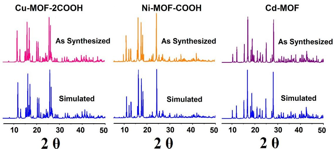
Fig 2S. As synthesized and simulated PXRD patterns of Cu-MOF-2COOH, Ni-MOF-COOH and Cd-MOF.
