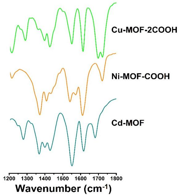
Fig 1S. FTIR spectra of the MOFs in the carboxylate frequency region.
