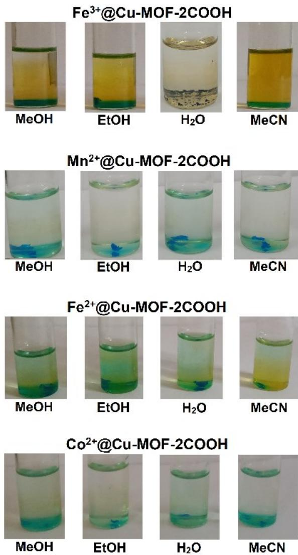
Fig 3S. Colour changes observed in the crystals after soaking Cu-MOF-2COOH in various cationic solutions in different solvents after 24 h.
