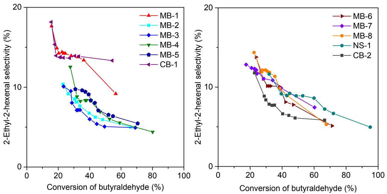
**Fig. S17** 2-Ethyl-2-hexenal **6** selectivity versus conversion of butyraldehyde in Prins–Friedel–Crafts reaction over the obtained and reference samples.
