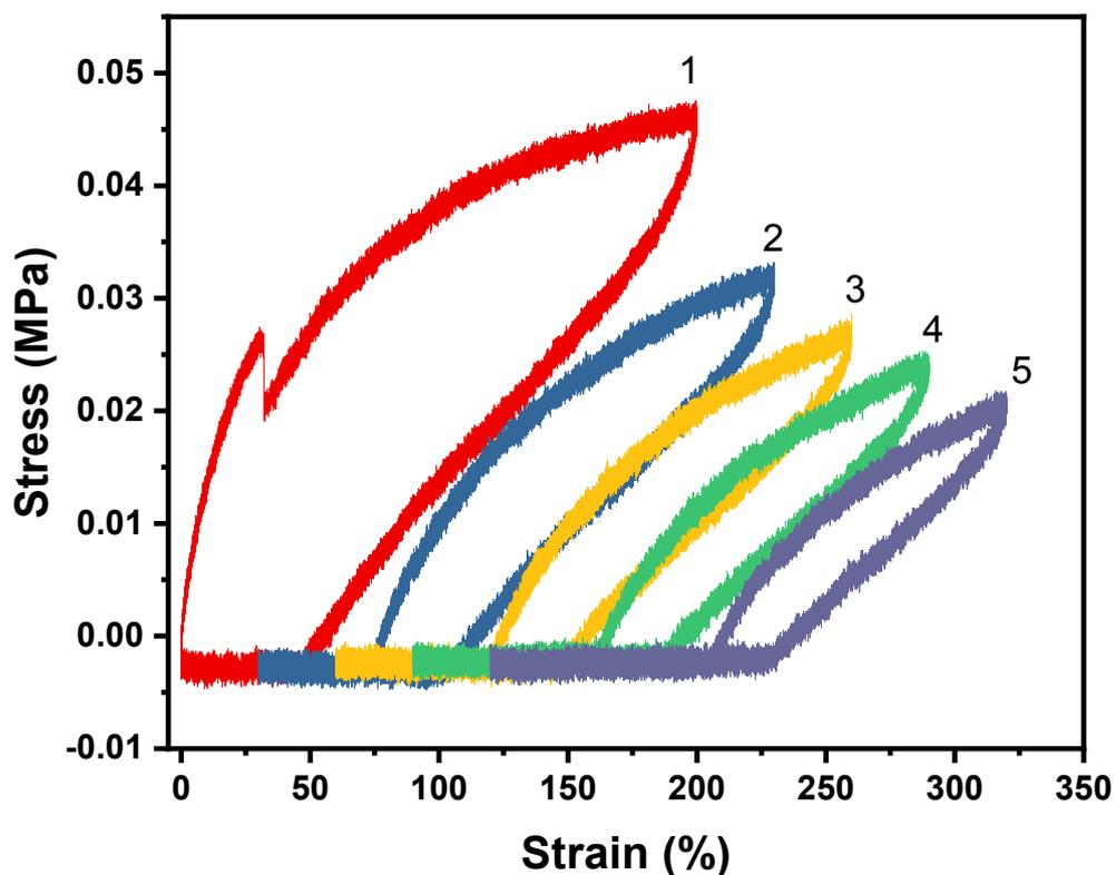
**Fig. S16** Cyclical tensile testing for ABA (81,48) (0-200 % strain, 10 cycles). Curves 1 -5 shown with a horizontal offset for clarity.
