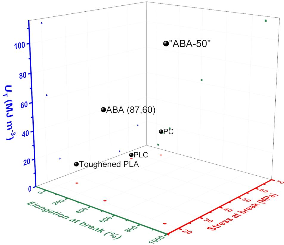
**Fig. S17** 3D scatter plot comparison of mechanical properties of ABA (87,60) and selected commercial and literature materials. Tensile toughness ( $U_T$ ) = blue axis (zy plane) & triangle marker; elongation at break ( $\epsilon_b$ ) = green axis (xz plane) & square marker; stress at break ( $\sigma_b$ ) = red axis (xy plane) & circle marker.
