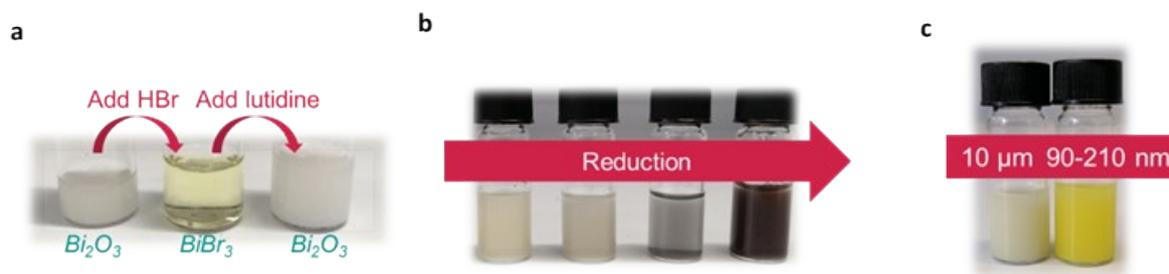
**Fig. S5** Physicochemical properties of  $\text{Bi}_2\text{O}_3$  particles. **(a)** reaction with HBr and prevention with the addition of 2,6-lutidine. **(b)** reduction into  $\text{Bi}^0$  in various solvents. From left to right: acetone; acetone:PEG 400 (8:2); acetone:ethylene glycol (8:2); benzyl alcohol. **(c)** effect of the particle size on the color of the solution.
