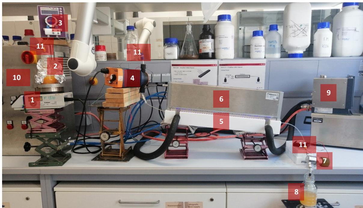
**Fig. S3** General continuous flow setup for the ATRA reaction photocatalyzed by  $\text{Bi}_2\text{O}_3$  particles. **1** magnetic stirrer; **2** reaction mixture; **3** metering peristaltic pump (SF-10, Vapourtec); **4** pulsator (Creaflow customized ProMinent (beta/4) pump with PTFE/carbon pump head); **5** HANU reactor; **6** Peschl LED module (405 nm); **7** BPR (Swagelok, 5 bar); **8** collection vessel; **9** Huber cryostat; **10** LED cooling system; **11** Vibrators
