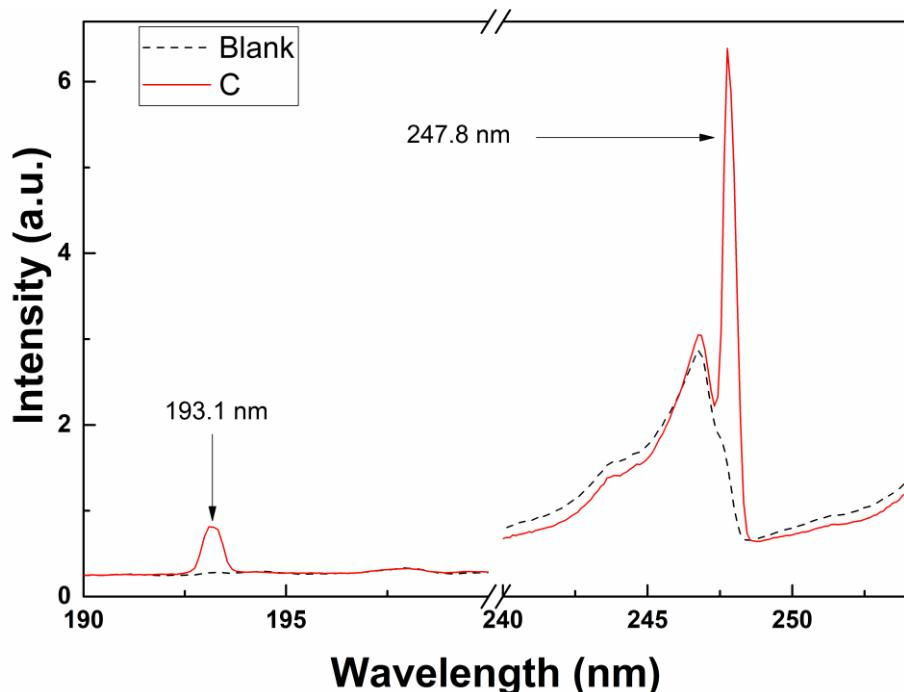
Fig. S2. Carbon atomic emission spectra.
