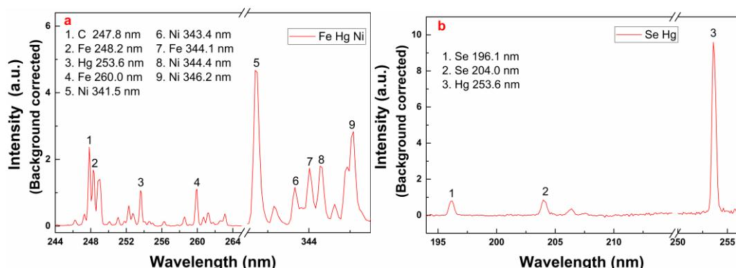
Fig. S1. Atomic emission spectra of simultaneous determination of : (a)  $15 \text{ mg L}^{-1}$  Ni(II),  $500 \mu\text{g L}^{-1}$  Hg(II) and  $10 \text{ mg L}^{-1}$  Fe(III); (b)  $500 \mu\text{g L}^{-1}$  Se(IV) and  $4 \text{ mg L}^{-1}$  Hg(II).
