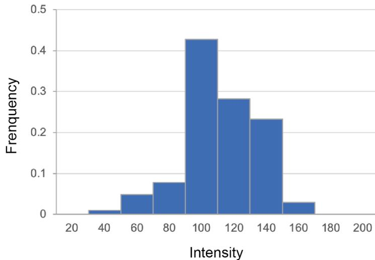
Figure S4. The intensity distribution of droplets with fluorescence signals after 40 cycles of thermal ramping.
