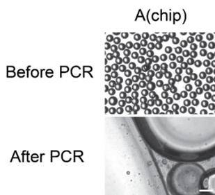
Figure S2. Droplets generated with PCR buffer (NEB) and oil-surfactant mixture of 4.5% (v/v) Span 80, 0.4% (v/v) Tween 80, and 0.05% (v/v) Triton X-100 in mineral oil by microfluidic chip (Droplet Junction Chip with 100  $\mu$ m etch depth, Dolomite) before and after 40 PCR cycles. Coalescence was obviously observed. Similar results got from chip and MiCA shows MiCA as a method for producing droplets does not change inherent properties of emulsion. Scale bar: 100  $\mu$ m.
