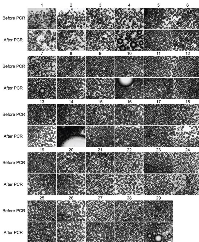
Figure S3. Droplets generated with PCR buffer (NEB) and all oil-surfactant mixtures using MiCA, observed before and after 40 PCR cycles. Scale bar: 100  $\mu$ m.
