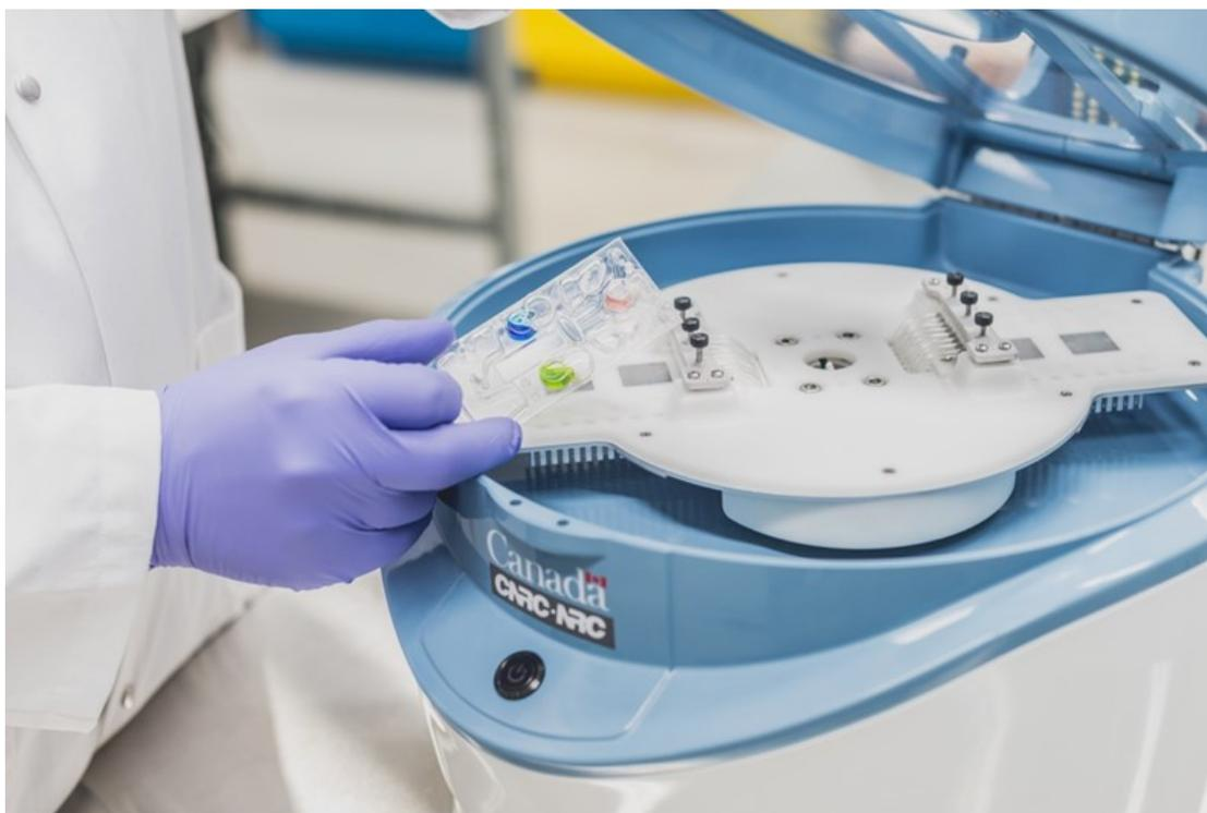
**Fig. S1** Centrifugal microfluidic platform. The photograph shows a prototype instrument during the installation of a microfluidic cartridge (unrelated to the work described in here).
