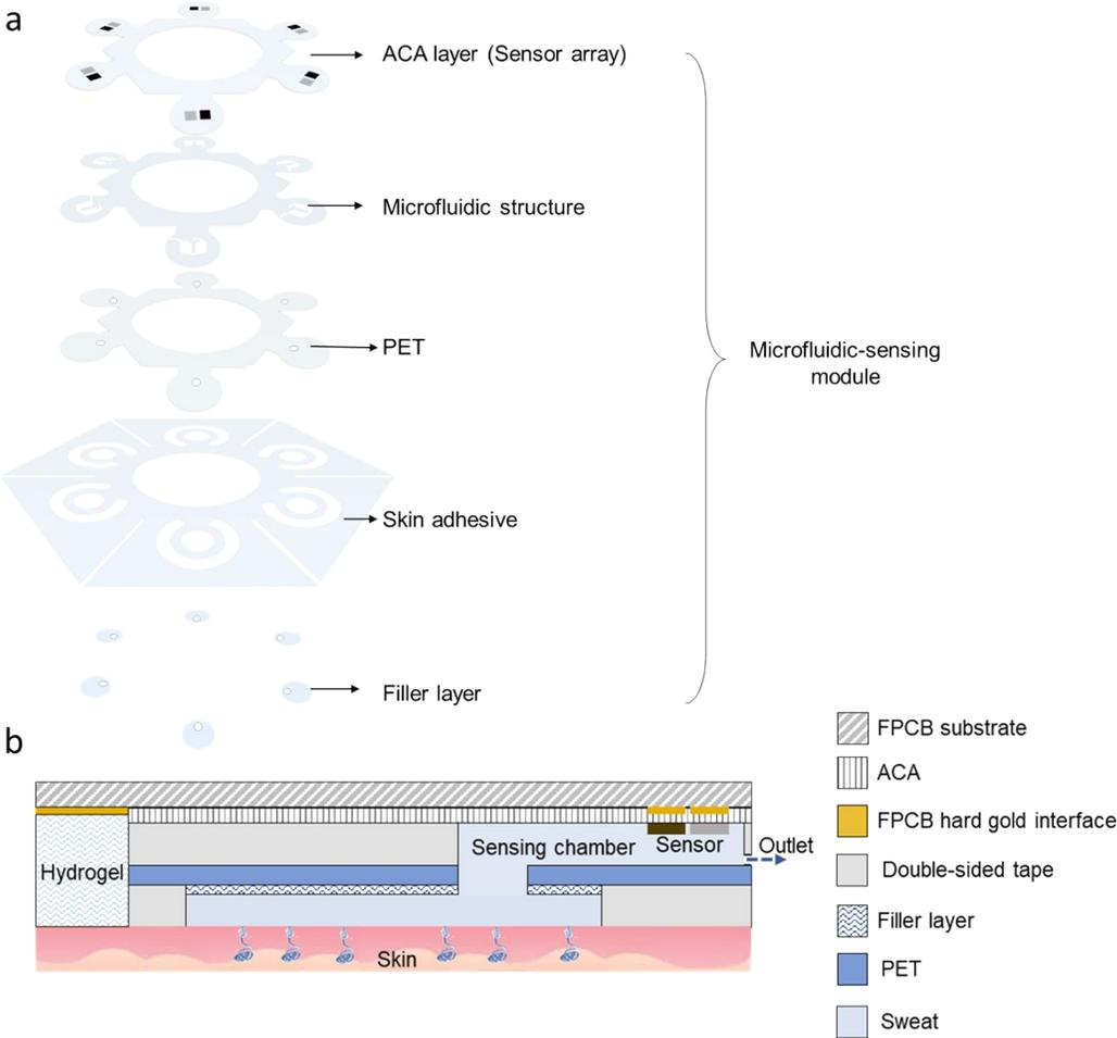
**Figure S1:** a) Exploded view of the microfluidic-sensing module; b) Cross-section view of the microfluidic-sensing module-skin interface.
