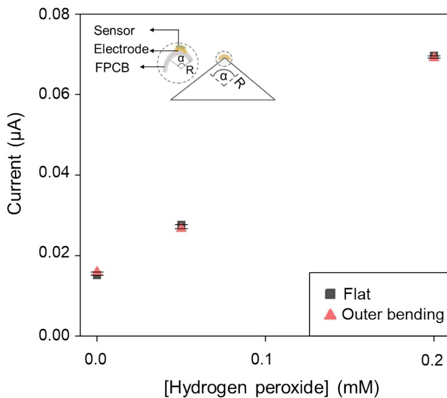
**Figure S5:** Evaluation of the PtNP/Au electrode (sensor substrate) response to hydrogen peroxide under different bending conditions (1. no bending, and 2.  $\alpha = 60^\circ$ ,  $R = 15$  mm).
