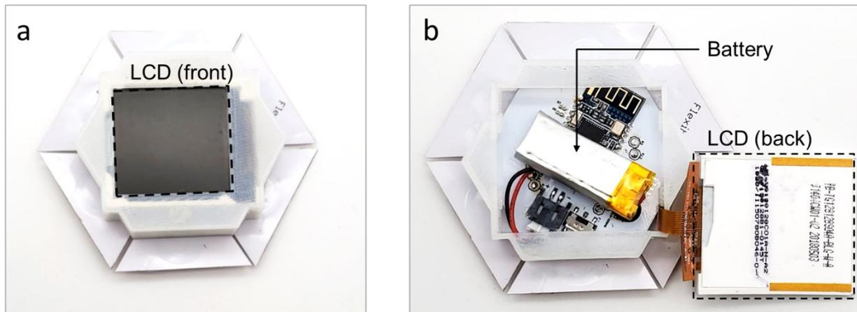
**Figure S8:** Photographs of the system illustrating the LCD display (a) and a rechargeable lithium-ion polymer battery with 150 mAh capacity (b) enclosed by/embedded within a 3D-printed case.
