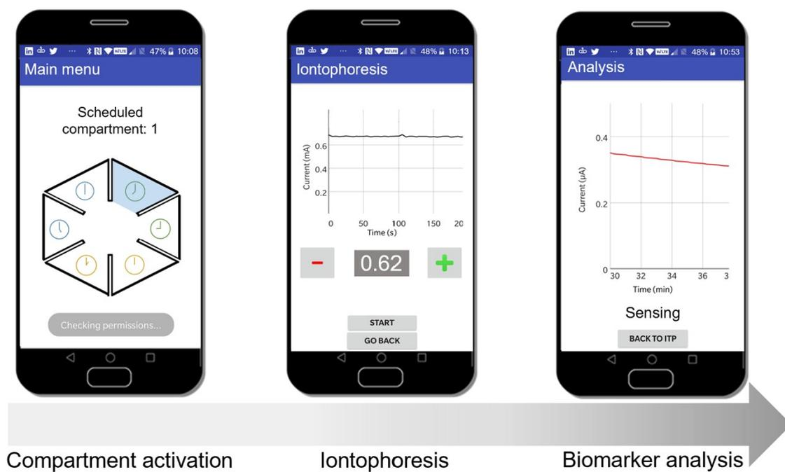
**Figure S6:** The custom-developed mobile application to control compartmentalized operations (programmable iontophoresis and sensing) and data display/storage.
