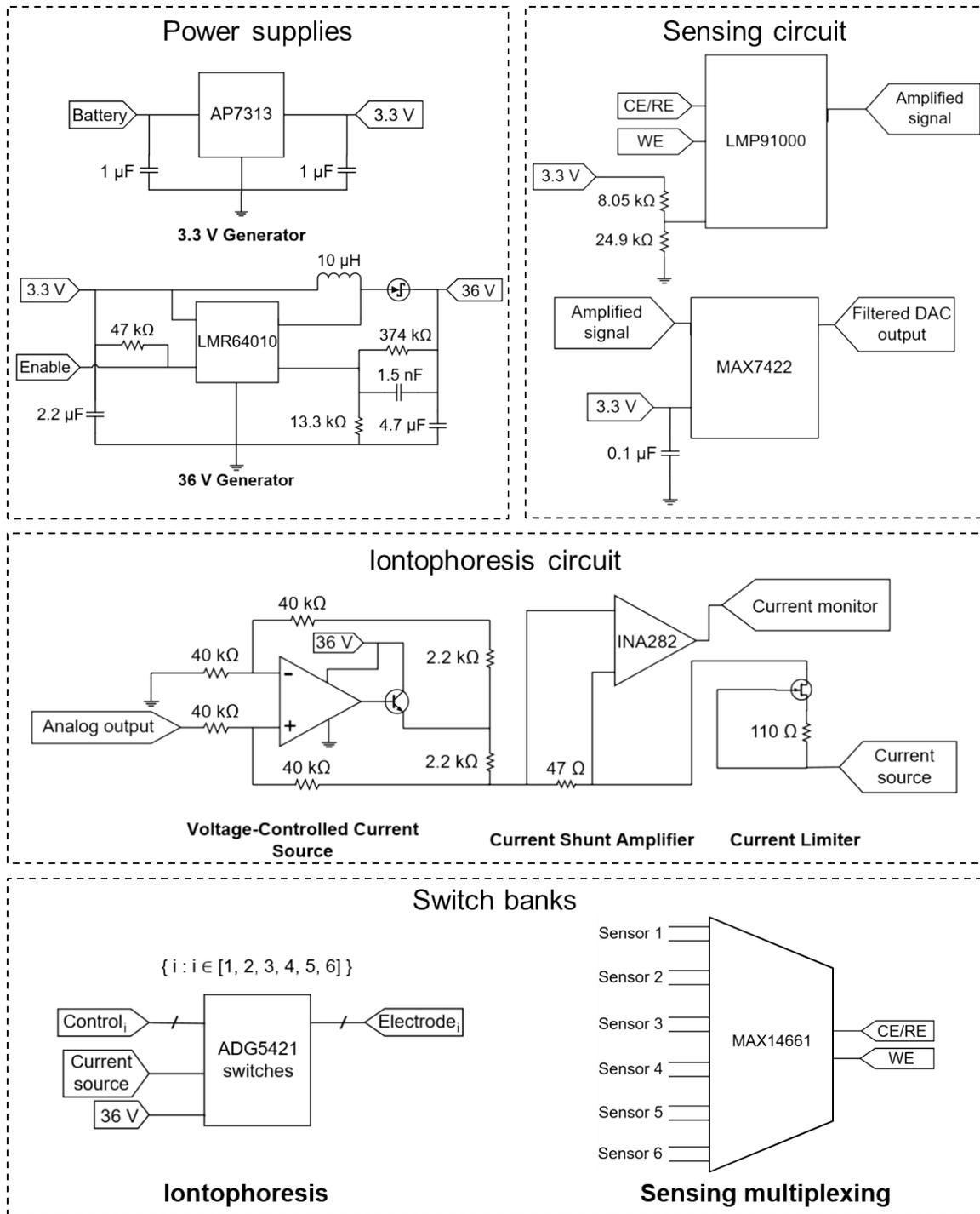
Figure S7: Schematic diagram of the wireless FPCB's circuitries.
