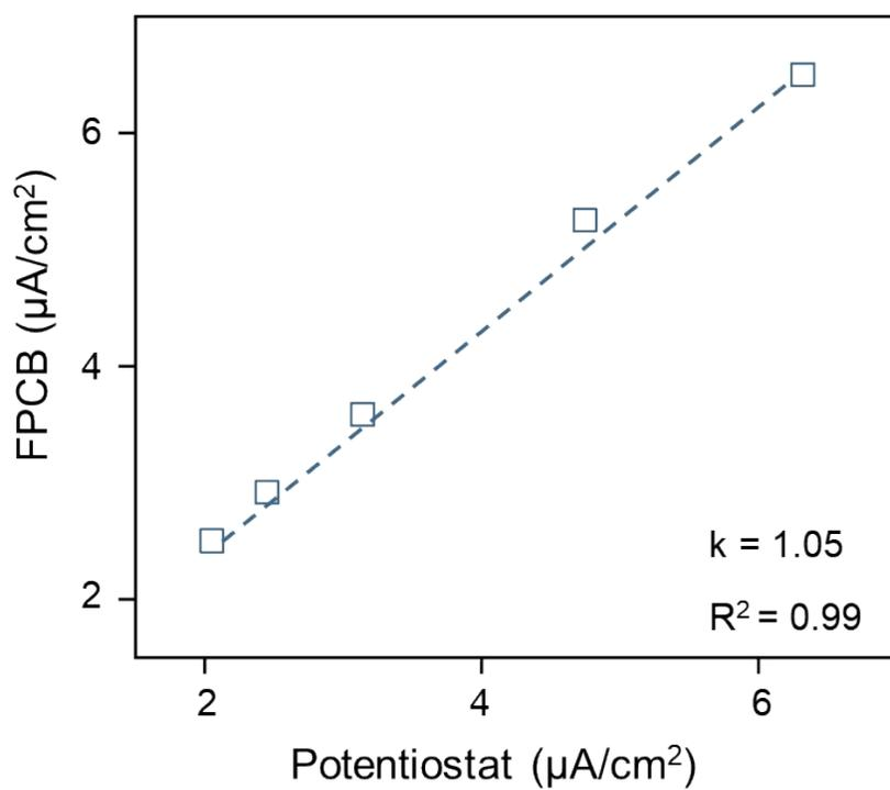
**Figure S4:** Comparison of glucose sensor readouts (current density) captured by the FPCB vs. potentiostat.
