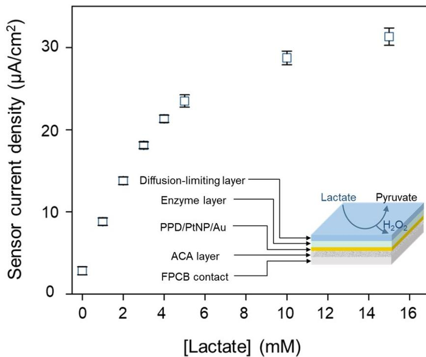
**Figure S3:** The developed lactate sensor's responses to different lactate solutions (SE,  $n = 3$ ). Inset illustrates the underlying layers of the constructed lactate sensing interface.
