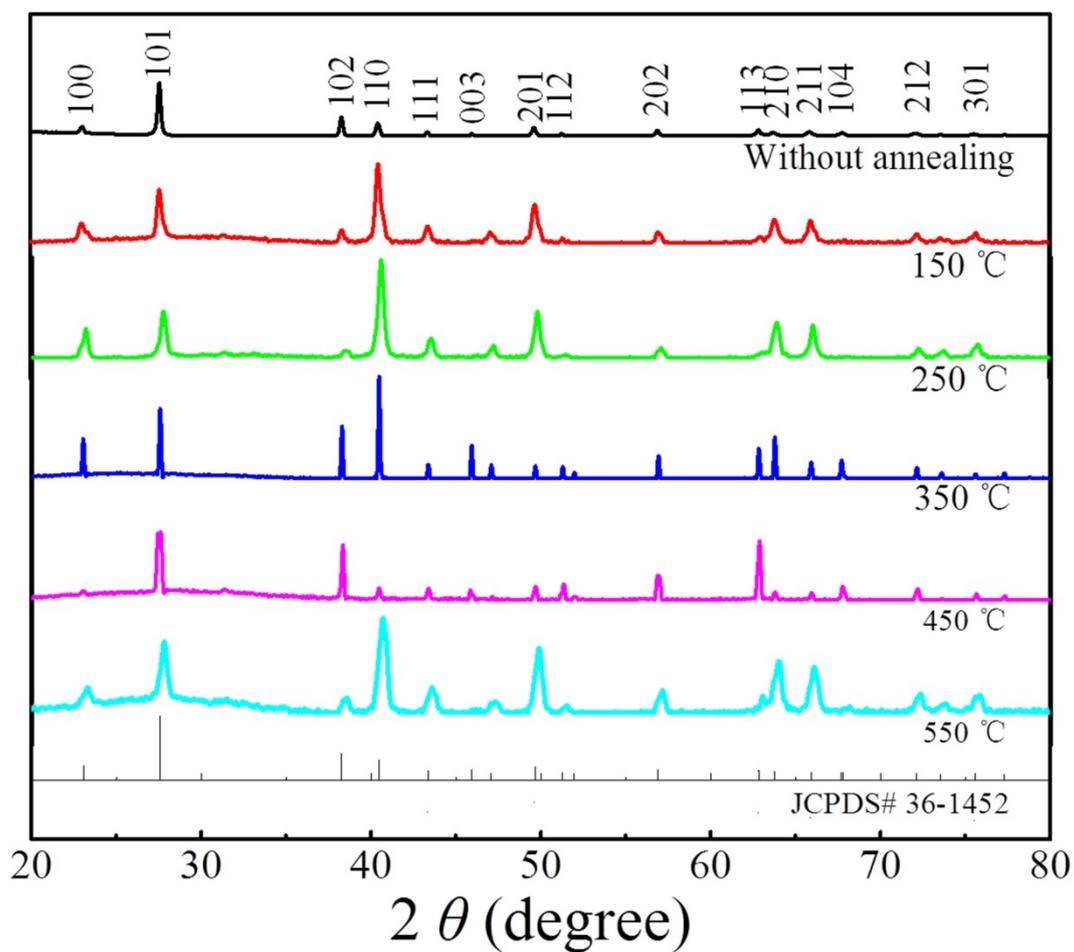
Fig. S4 XRD patterns of optimized Te NWs thin pieces with or without annealing at different temperature for 3 h.
