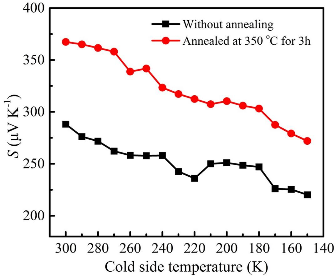
Fig. S7 Temperature-dependent Seebeck coefficient of the optimized Te NWs thin pieces with or without annealing at 350 °C for 3 h.
