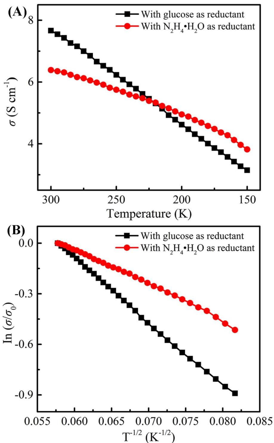
Fig. S6 Dependence of electrical conductivity on temperature (A) and analysis of the temperature-dependent of the electrical conductivity with the 1D VRH model (B) of the as-fabricated Te NWs thin piece after annealing at 350 °C for 3 h, where the Te NWs were synthesized with glucose (black line) at 120 °C for 12 h and N<sub>2</sub>H<sub>4</sub>•H<sub>2</sub>O (red line) as reductant, respectively.
