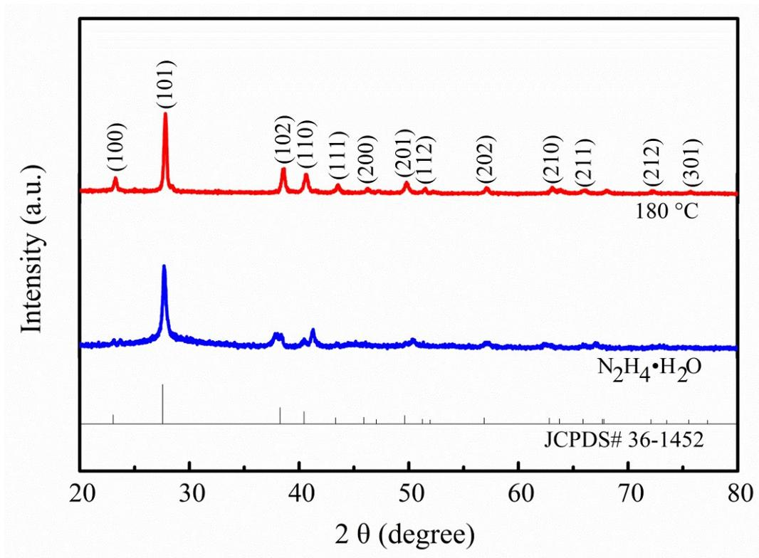
Fig. S1 XRD pattern of the as-synthesized Te NWs with glucose at 180 °C for 12 h and the N<sub>2</sub>H<sub>4</sub>•H<sub>2</sub>O synthesized one.
