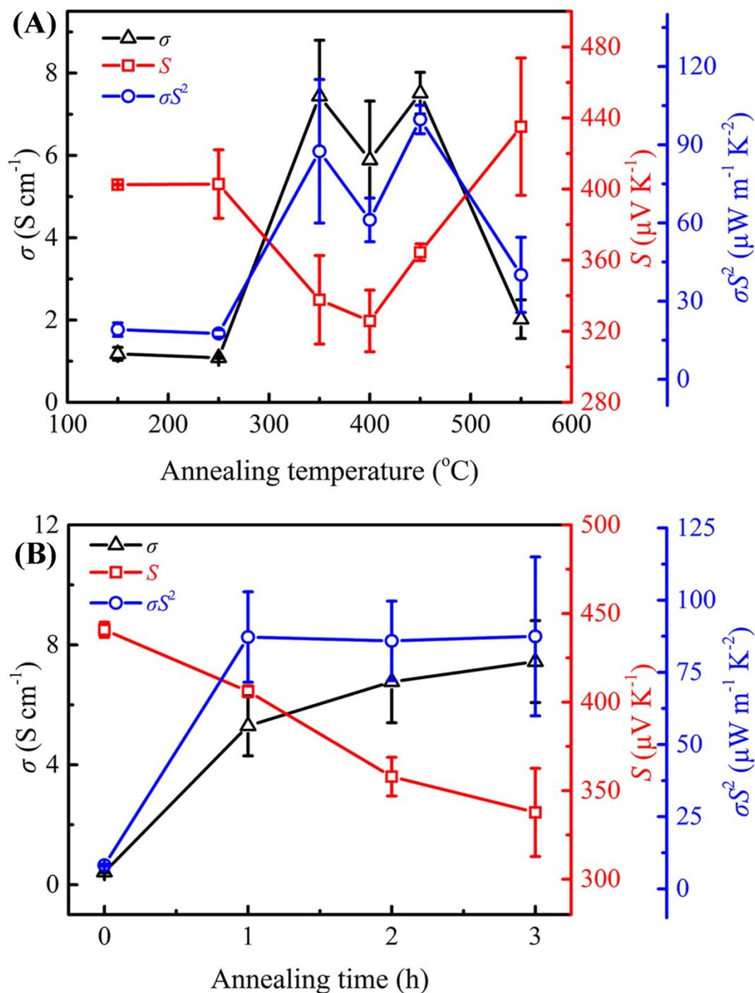
Fig. S3 The TE performance of the as-fabricated Te NWs thin piece versus different annealing temperature for 3 h (A) and different annealing time at 350 °C (B), where the Te NWs were synthesized with  $\text{N}_2\text{H}_4 \cdot \text{H}_2\text{O}$ .
