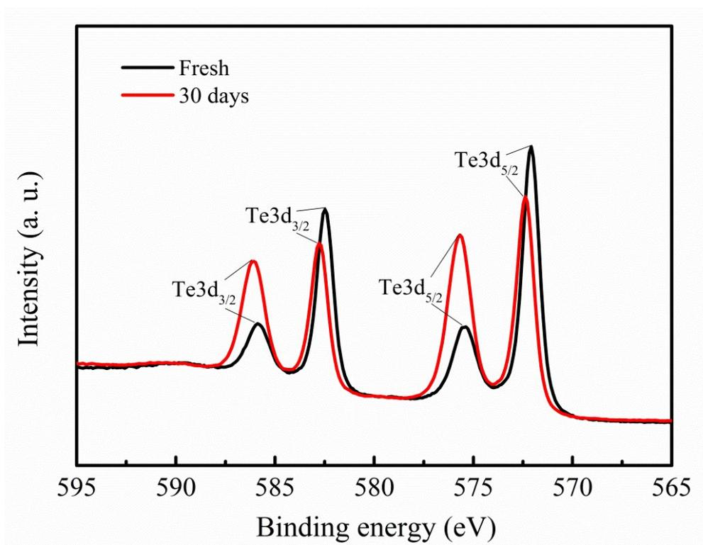
Fig. S9 Te3d XPS spectra of the fresh (red line) and keeping at ambience condition for 30 days (black line) of the  $\text{N}_2\text{H}_4 \cdot \text{H}_2\text{O}$  synthesized Te NWs.
