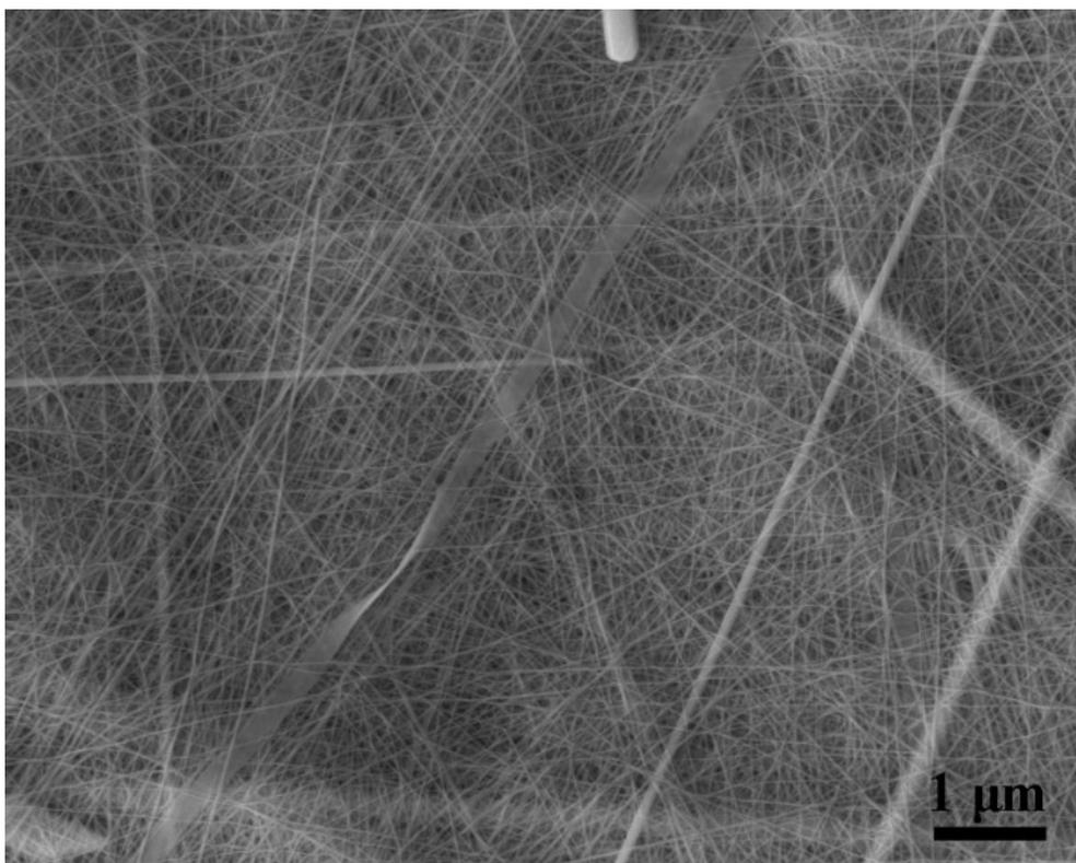
Fig. S2 SEM image of the as-synthesized Te NWs with  $\text{N}_2\text{H}_4 \cdot \text{H}_2\text{O}$  as reductant.
