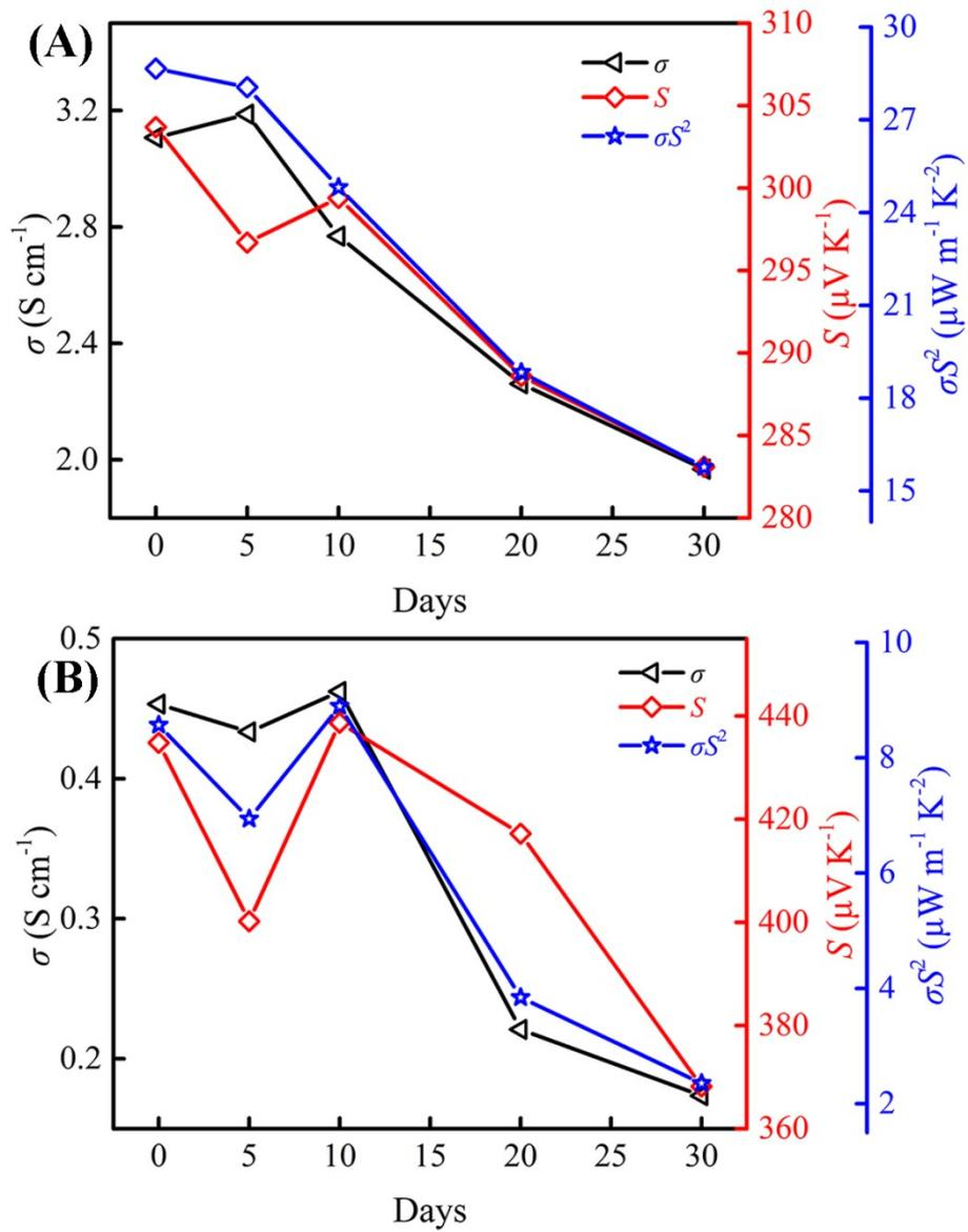
Fig. S8 Dependence of electrical conductivity, Seebeck coefficient, and power factor of the as-fabricated Te NWs thin piece on time (days), where the Te NWs were synthesized with glucose (A) at 120 °C for 12 h and  $\text{N}_2\text{H}_4\cdot\text{H}_2\text{O}$  (B).
