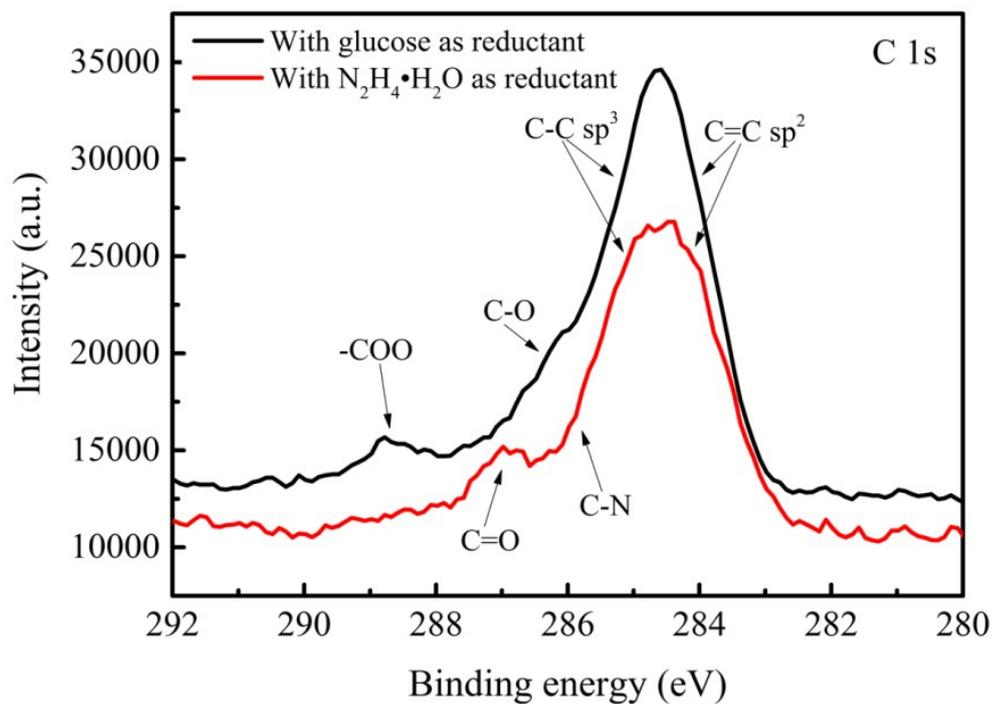
Fig. S5 C1s XPS spectra of the glucose (black line) and N<sub>2</sub>H<sub>4</sub>·H<sub>2</sub>O (red line) synthesized fresh Te NWs, the glucose synthesized one was synthesized at 120 °C for 12 h.
