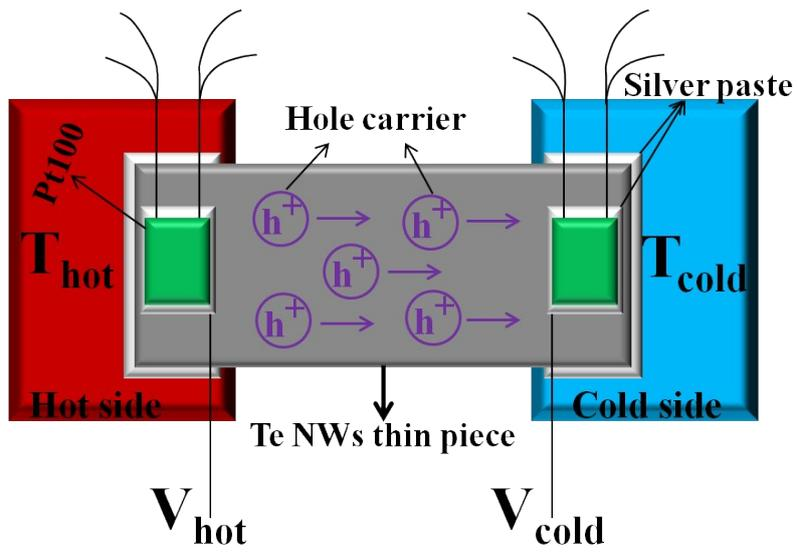
Scheme S1 The schematic measurement of Seebeck coefficient for Te NW film.
