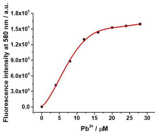
**Fig. S2** Fluorescence intensity of **RPb1** (20 μM) at 580 nm with increasing concentrations of Pb<sup>2+</sup> in HEPES buffer (20 mM, pH 7.4, containing 2% DMSO as a cosolvent, v/v).
