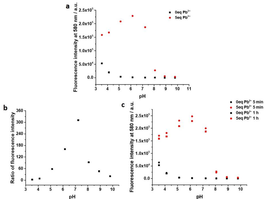
**Fig. S6** (a) Fluorescence intensity of **RPb1** (20 μM) at 580 nm in the absence and presence of Pb<sup>2+</sup> at different pH values in HEPES buffer (20 mM, containing 2% DMSO as a cosolvent, v/v). (b) Ratio of fluorescence intensity of **RPb1** at 580 nm in the presence of Pb<sup>2+</sup> to that in the absence of Pb<sup>2+</sup>. (c) Fluorescence stabilities of **RPb1** (20 μM) at 580 nm at different pH values in HEPES buffers after treatment of Pb<sup>2+</sup> for 5 min and 1 h.
