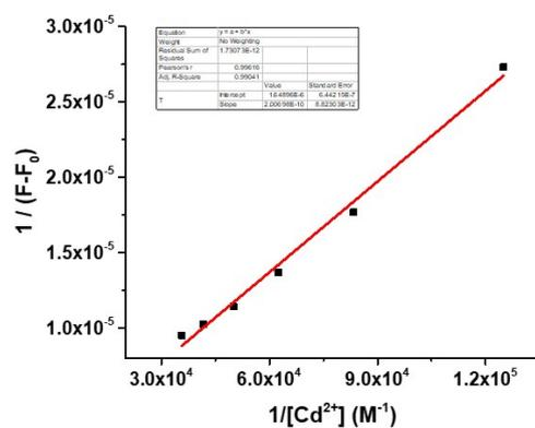
**Fig. S7** Benesi-Hildebrand plot of **RPb1** (20 μM) with different concentrations of Cd<sup>2+</sup> in HEPES buffer (20 mM, pH 7.4, containing 2% DMSO as a cosolvent, v/v).  $y = 1.64896 \times 10^{-6} + 2.00698 \times 10^{-10}x$
