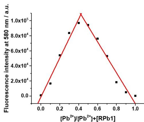
**Fig. S3** Job's plot of **RPb1** with Pb<sup>2+</sup> in HEPES buffer (20 mM, pH 7.4).
