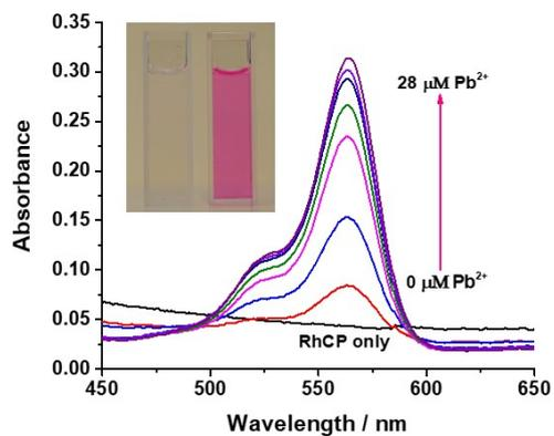
**Fig. S1** UV-vis absorbance spectra of **RPb1** (20 μM) in the presence of various amounts of Pb<sup>2+</sup> (0-28 μM) in HEPES buffer (20 mM, pH 7.4, containing 2% DMSO as a cosolvent, v/v). The inset shows color of **RPb1** (20 μM) before (left) and after (right) addition of Pb<sup>2+</sup> (20 μM).
