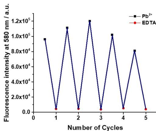
**Fig. S5** Fluorescence intensity of **RPb1** (20  $\mu\text{M}$ ) at 580 nm upon alternative addition of  $\text{Pb}^{2+}$  (20  $\mu\text{M}$ ) and EDTA (20  $\mu\text{M}$ ) in HEPES buffer (20 mM, pH 7.4). Number of cycles refers to alternating  $\text{Pb}^{2+}$ /EDTA cycles.
