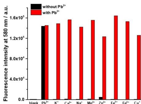
**Fig. S9** Fluorescence intensity of **RPb1** (20 μM) at 580 nm (λ<sub>ex</sub> = 526 nm) after addition of various metals (100 equivalents for K<sup>+</sup>, Ca<sup>2+</sup>, Na<sup>+</sup> and Mg<sup>2+</sup>, one equivalent for others) followed by Pb<sup>2+</sup> (one equivalent).
