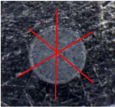
**Figure S5.** Picture of a white stain, the red line indicates the region where the profile on white stain was measured by a stylus profilometer.
